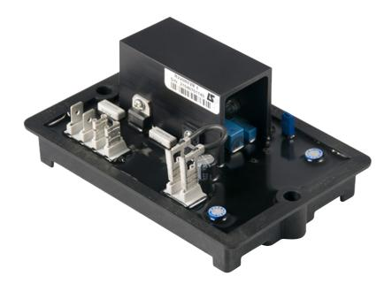
R220 is an analog AVR with power controled by transistors. It is designed for small alternators with a SHUNT excitation.
