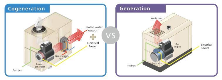
By capturing the waste heat from the gas engine the energy efficiency in the case of cogeneration is much higher than that of generation.
