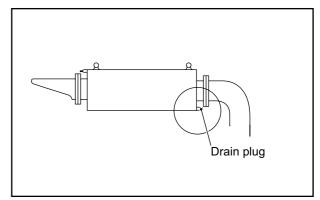
Fig. 8-25 Draining Water From the Exhaust Muffler
