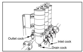
Fig. 8-5 Water Separator - Drain Water
