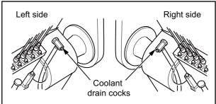
The coolant drain cocks located in the crankcase respectively (behind the each fuel injection pump accessory drive unit).
