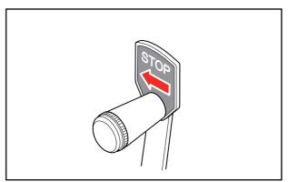
Fig. 3-19 Manual Stop Lever
