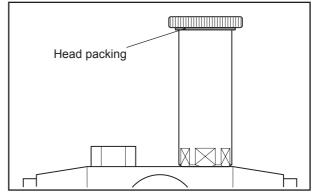
Fig. 3-5 Priming Pump Head Packing
