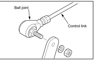
Fig. 8-11 Fuel Control Link - Remove
