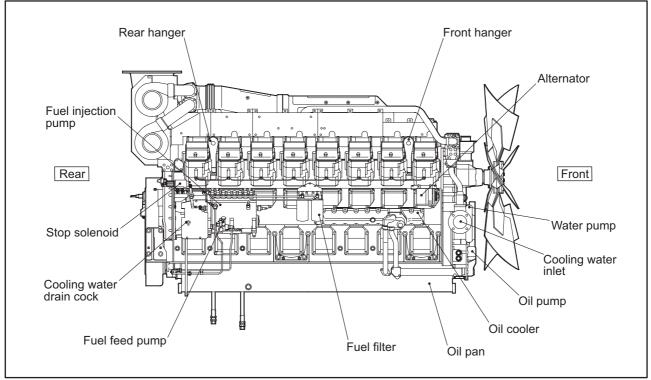
Fig. 2-2 Engine Right Side View
