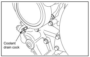
Fig. 8-22 Coolant Drain Cock (Water Pump)
