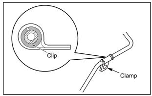
Fig. 8-19 Oil Pipe and Clip - Inspect and Replace
