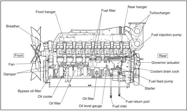
Fig. 2-1 Engine Left Side View
