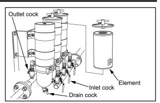
Fig. 8-6 Water Separator Element - Replace
