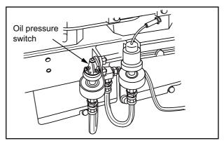
Fig. 2-9 Oil Pressure Switch
