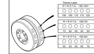
Fig. 8-3 Damper Temperature Management
