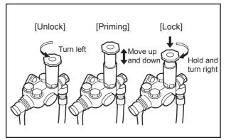
Fig. 3-1 Priming Pump - Handle
