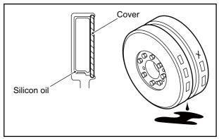
Fig. 8-2 Damper - Check Visually
