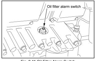
Fig. 2-11 Oil Filter Alarm Switch
