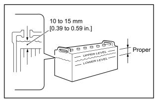
Fig. 3-11 Battery Electrolyte Level - Inspect
