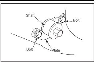
Fig. 2-14 Manual Turning Gear Position (While Engine is Running)
