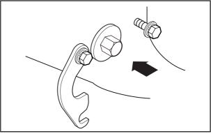
Fig. 2-15 Manual Turning Gear Position (When Pushing Shaft in)
