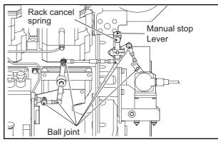
Fig. 3-13 Fuel Control Link - Check
