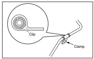
Fig. 8-13 Low Pressure Fuel Pipe and Clip - Inspect
