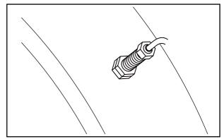
Fig. 2-8 Revolution Detection Pickup
