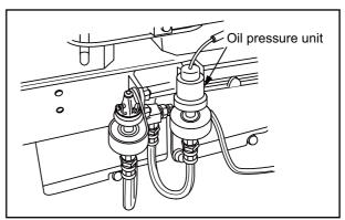
Fig. 2-6 Oil Pressure Unit
