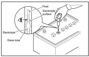
Fig. 8-31 Specific Gravity of Battery Electrolyte -Check
