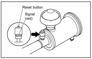
Fig. 3-15 Air Cleaner - Check for Clogging
