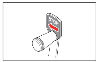
Fig. 2-4 Manual Stop Lever
