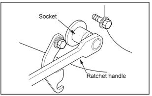
Fig. 2-16 Turning Gear Position (When Turning Shaft)
