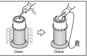
Fig. 8-28 Air Cleaner Element - Clean and Check
