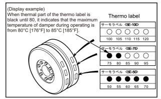
Fig. 3-18 Thermo label of damper
