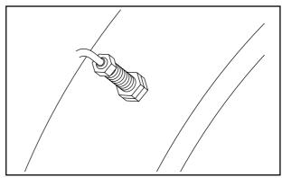
Fig. 2-12 Revolution Detection Pickup
