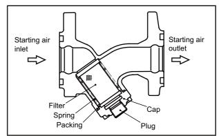
Fig. 8-34 Air Strainer - Drain Water and Clean
