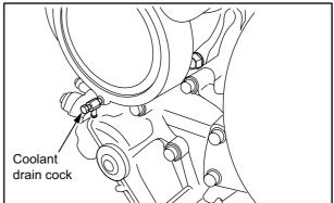
Fig. 3-10 Coolant Drain Cock (Water Pump)
