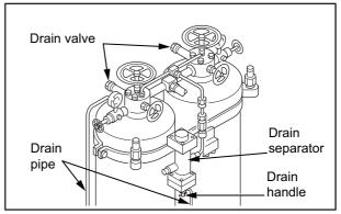
Fig. 8-35 Air tank - Drain water
