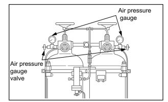
Fig. 3-17 Starting Air Tank Air Pressure - Check
