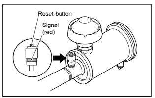
Fig. 8-29 Air Cleaner - Check for Clogging
