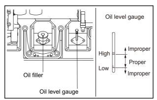
Fig. 3-14 Oil Filler and Oil Level Gauge
