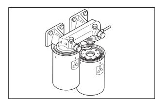
Fig. 8-8 Fuel Filter - Replace
