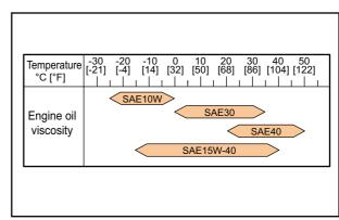
Fig. 5-2 Selection of Oil Viscosity
