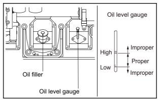
Fig. 8-14 Oil Filler and Oil Level Gauge
