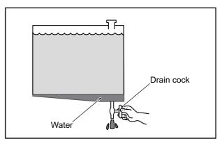
Fig. 8-4 Fuel Tank - Drain Water
