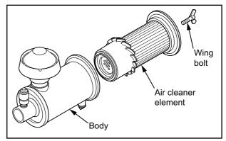
Fig. 8-27 Air Cleaner Element - Remove
