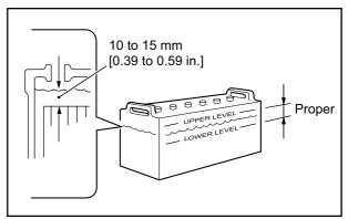
Fig. 8-30 Battery Electrolyte Level - Inspect
