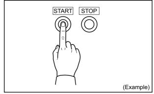
Fig. 2-3 Start Switch and Stop Switch
