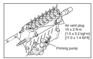
Fig. 3-3 Fuel Injection Pump - Bleed Air
