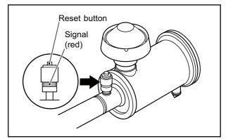
Fig. 8-26 Air Cleaner - Check for Clogging
