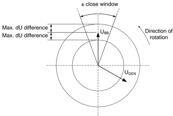
The synchronisation pulse is sent depending on the settings in **2020 Synchronisation**. It depends on whether it is the GB/SCB/BTB or the TB (EDG only) that is to be synchronised.
