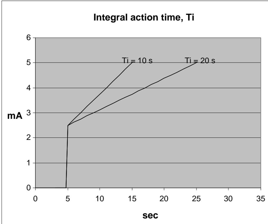
As seen on the drawing, the output reaches 5 mA twice as fast at a  $T_i$  setting of 10 s than with a setting of 20 s.
