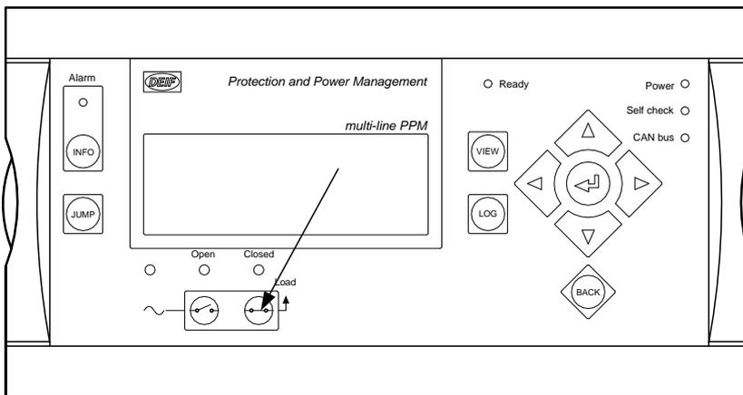
As soon as the shore breaker is closed, the status text "SHIP TO SHIP ACTIVE" is indicated at the display unit for the shore connection controller.
