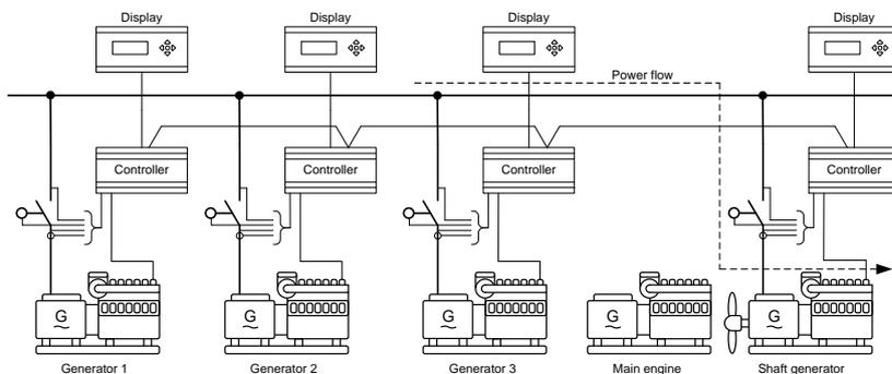
The shaft generator has to be synchronised manually when PTH mode is selected. Since the main engine is shut off, the synchronisation has to take place using a pony motor or the like.
