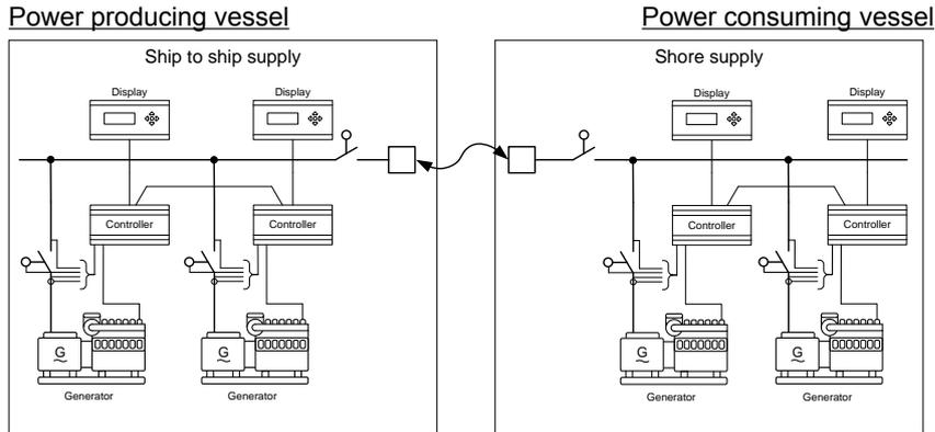
As soon as "ship-to-ship" supply is selected for a PPM-3 SC unit, the display unit will indicate the status message: "SHIP TO SHIP ENABLED".
