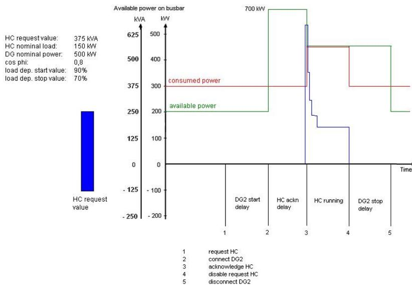
After the available power is above the requested HC power, the heavy consumer is subsequently blocked until the programmed HC acknowledge delay runs out (fixed delay of 4 s).
