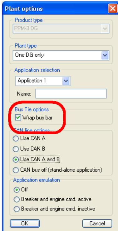
To allow closed ring connection on the busbar, parameter 8990 (Closed Ring) is selected to ON. When requesting BTB open with a closed ring connection, the BTB that is requested will trip the breaker. De-load will not be performed!
