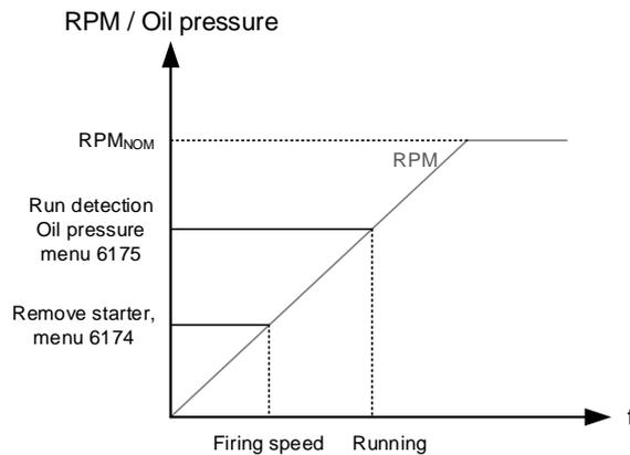
**i** The remove starter function can be using the MPU or a digital input.
