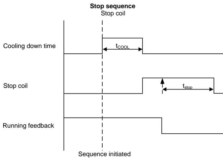
The stop sequence will be activated, if a stop command is given. The stop sequence includes the cooling down time if the stop is a normal or controlled stop.
