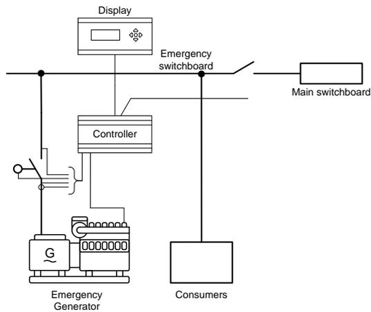
**i** With an emergency generator in the system, a maximum of 15 diesel generators can be controlled.
