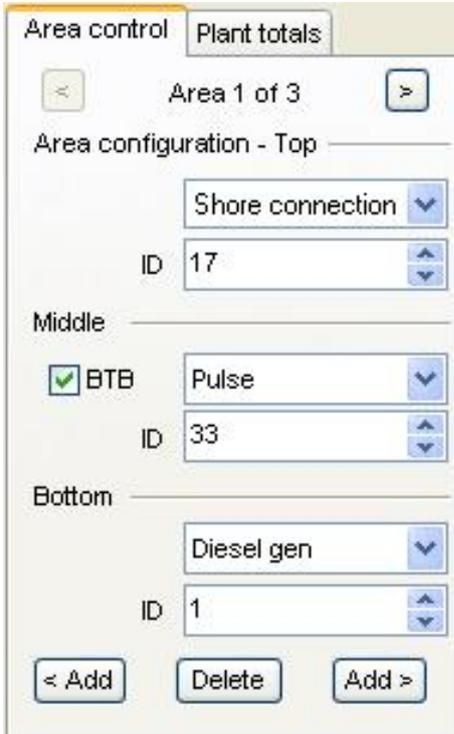
For each section, it is defined whether a generator and a shaft generator and/or a shore connection is present, and the amount and type of breakers.
