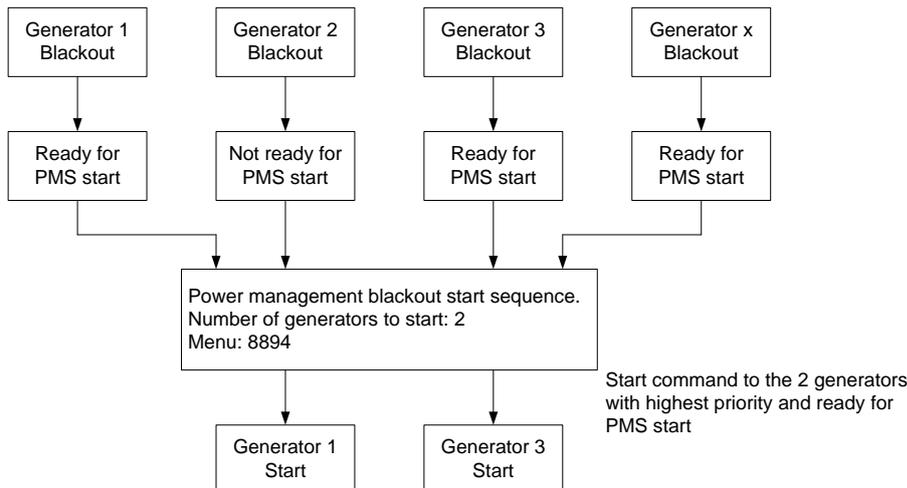
The blackout start sequence will activate the automatic start sequence, starting the generators with the highest priority and the second highest start priority (if selected), which at the same time are "ready for PMS start".
