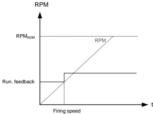
The diagram illustrates how the digital running feedback (terminal 117) is activated, when the engine has reached its firing speed.
