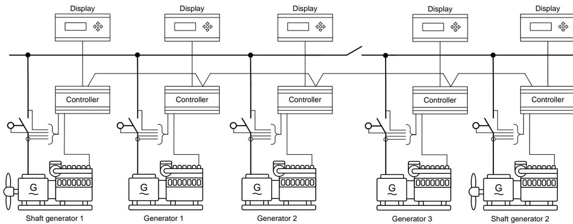
**i** Diesel generators can be added on both sides of the bus tie breaker.
