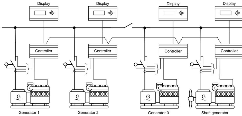
**i** Diesel generators can be added on both sides of the bus tie breaker.
