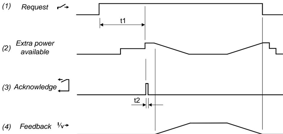
The analogue power feedback for the heavy consumer is intended for a power transducer with a 4 to 20 mA output corresponding to 0 to 100 % load. If the heavy consumer is of 400 kW, then the power transducer has to be calibrated to 0 to 400 kW = 4 to 20 mA, and the setting has to be set for 400 kW.
