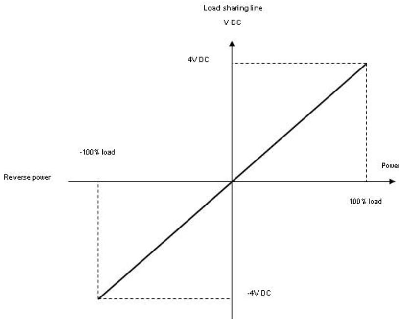
The active load sharing line is illustrated above, and the characteristics of the reactive load sharing line are equivalent to it.
