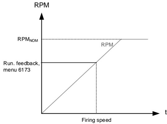
**⚠ Notice that the factory setting of 1000 RPM is higher than the RPM level of starter motors of typical design. Adjust this to a lower value to avoid damage of the starter motor.**
