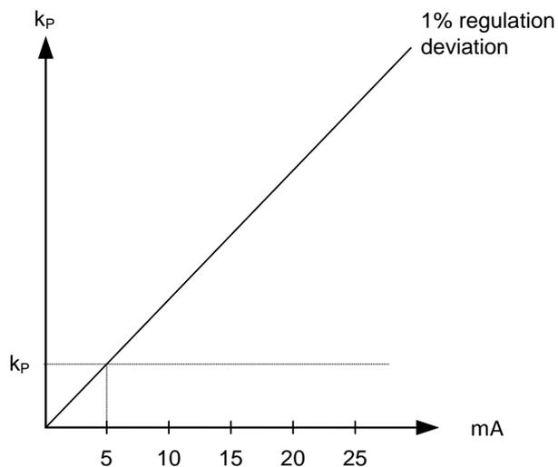
A 1 % regulation deviation occurs. With the Kp setting adjusted, the deviation causes the output to change 5 mA. The table shows that the output of the PPM-3 changes relatively much, if the maximum speed range is low.
