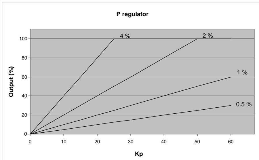
In this example, we have a 2 percent regulation deviation and an adjusted value of the  $K_p = 20$ . The calculated regulator value of the unit is 40 %. Now the pulse length can be calculated with a period time = 2500 ms:
