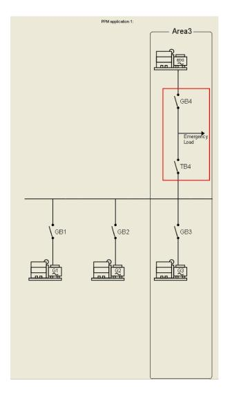
b) Define the ID numbers of each unit. In this example, the EDG unit has the ID number 4. Select parameter 7530 on the EDG unit and then select ID number 4.
