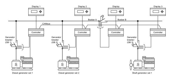
By default, this application supports two diesel generators (DGs) in parallel operation, one bus tie breaker (BTB) and one shore connection (SC)/shaft generator (SG) as illustrated above. The number of DGs can be extended to 16.
