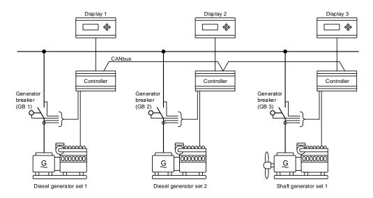
By default, this application supports two diesel generators (DGs) in parallel operation and one shore connection (SC) or shaft generator (SG) as illustrated above. The number of DGs can be extended to 16.
