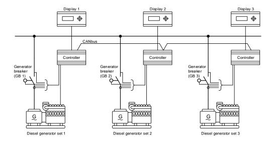
By default, this application supports three diesel generators (DGs) in parallel operation as illustrated above. The number of DGs can be extended to 16.
