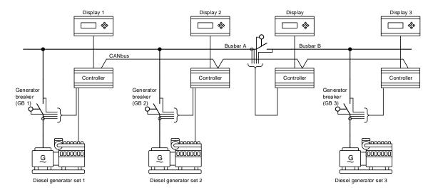
By default, this application supports four diesel generators (DGs) in parallel operation and one bus tie breaker (BTB). The number of DGs can be extended to 16 and the number of BTBs to eight.
