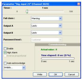
9 Select M-Logic and setup the digital inputs for breaker feedback.
