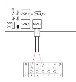
**NOTE** The DU-2 CAN bus communication is intended for DEIF use only and cannot be connected to other CAN bus systems.
