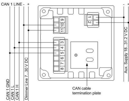
**NOTE** You can only install two terminations at a time on a CAN bus network.
