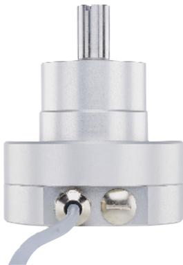
DEIF's rudder/azimuth angle transmitters convert the rudder or azimuth thruster's position angles into either electrical current signals or digital data values with a 16 bit resolution (+/-180de.g. = +/-32767).
