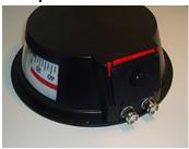
The transport lock (bright red plastic) is mounted to prevent the pointers from being damaged under heavy vibration and shock (transportation). The transport lock must be removed before connecting the indicator!
