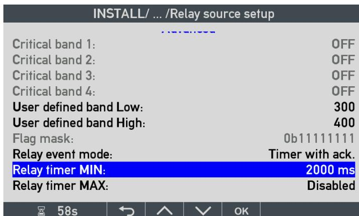
In this example with Relay timer MIN at 2000ms the relay will first activate when the rudder has stayed at, or above, 30° for the 2 second period and it will then stay active until you acknowledge by pushing any of the front buttons.
