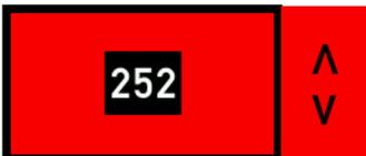
Using the front button  $\wedge$  or  $\vee$  you can adjust the red colour from 0 to 252. (Steps size is 4)
