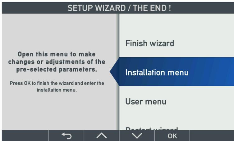
When the first 4 selections are made, you can either press OK to finish the wizard and go to normal operation or select one of the detailed setup menus.
