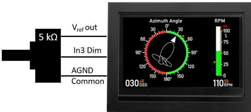
It is recommended to use a potentiometer in the range from 1 to 20 kΩ.
