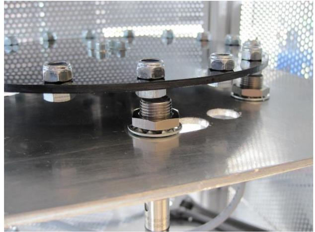
For unidirectional RPM measurements (direction independent) only one sensor is used.
