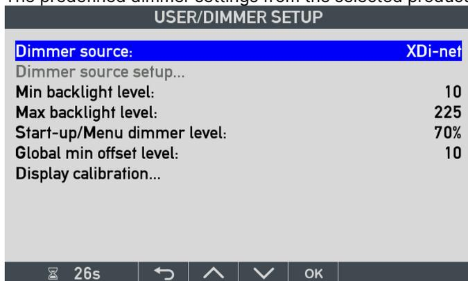
**Min backlight level** (local) is the backlight level that equals a dimmer value of 0 %. This setting should never be set to 0 since it turns the backlight totally off, and it will no longer be in accordance with regulations for a display-based bridge product. The valid value range is 0-100 out of the total of 250 backlight steps.
