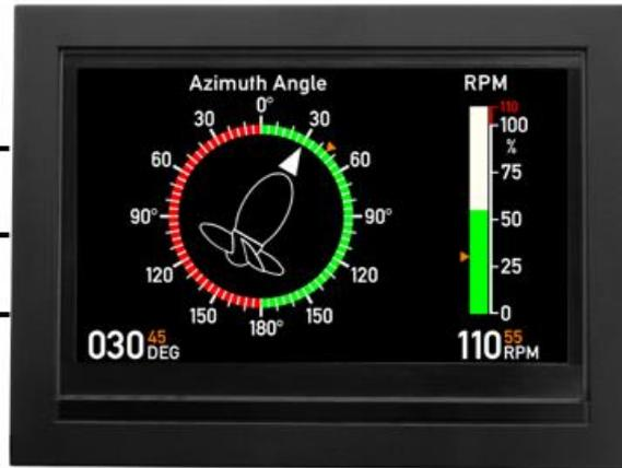
Example: In the DEIF standard library for azimuth thruster indication, it is possible to select a VS for sin/cos potentiometer input. This input pair has a predefined potentiometer supply voltage of +/-10 V, but this indicator will also work fine with any potentiometer supply between +/- 6 V and +/-15 V.
