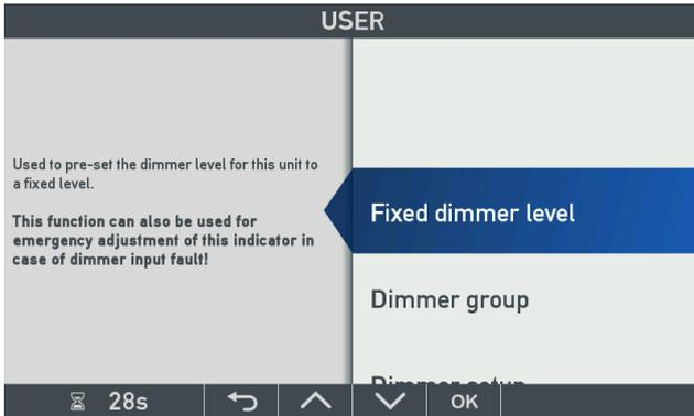
Press OK to enter "Fixed dimmer level", and a new menu will appear showing the actual virtual indicator together with a new soft-key menu for adjusting the fixed dimmer level:
