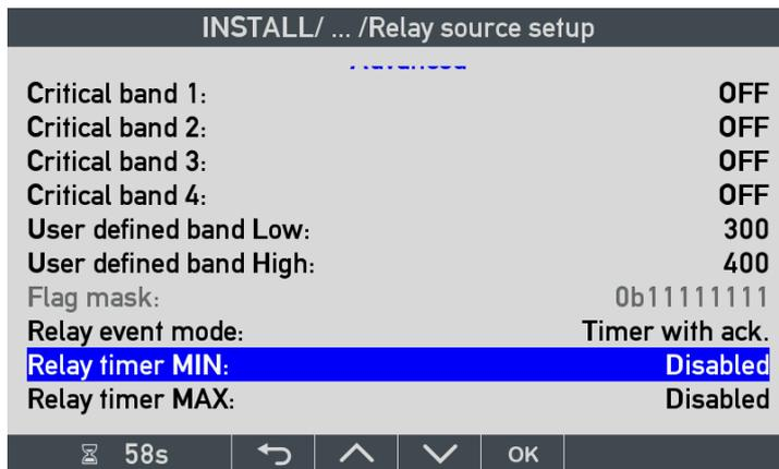
The relay will activate immediately when the rudder angle exceeds 30° and it will stay active until you make an acknowledge by pushing any of the front buttons.
