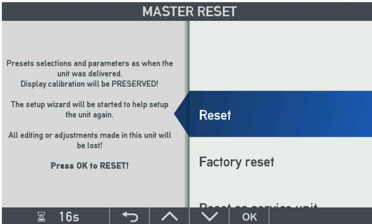
In this menu we have added a new “Reset” function that is bringing all back to factory settings except the colour calibration made via the “Display calibration” menu.
