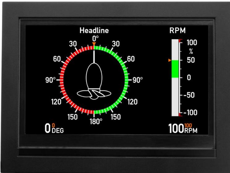
In this example, the default scaling setting in the VS02 profile is changed, so that +/-200 RPM is equal to 100 % (110 % is 220 RPM).
