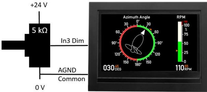
The supply voltage for the potentiometer in this configuration should be relatively stable since changes in this voltage will directly affect the dimmer level. The potentiometer value is not critical in a dimmer application.
