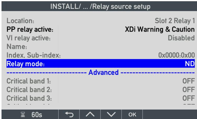
In this example, relay 1 is set up to be activated when a warning or caution event is present in the XDi. The actual warning or caution that will activate the relay depends on which warnings or cautions are activated in the selected PP or set up via the XDi user menu.
