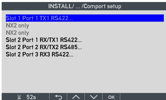
Please note that NMEA input 1 (RX1) and output 1 (TX1) is using the same UART and is therefore setup as one port, that is COM1.
