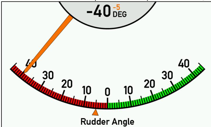
The result of the CCW setup above with input value -7828, the pointer shows PS 41.0°
