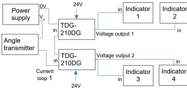
The indicators must be connected directly to the voltage output terminals to obtain the most robust system. (Star coupled)
