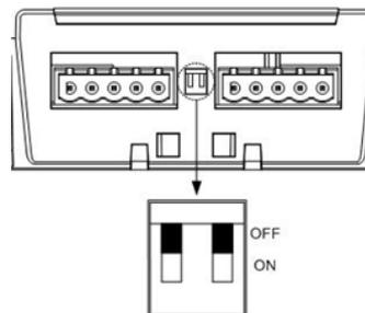
If a BRW-2 and TRI-2 CAN is located in an endpoint of the Can bus, the build in termination resistor can be activated.
