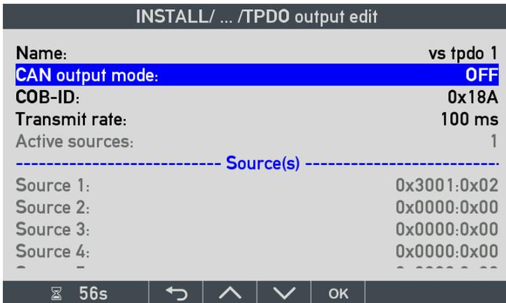
The TPDO output is disabled by default. The CAN output mode is OFF. Highlight "CAN output mode" and press OK.
