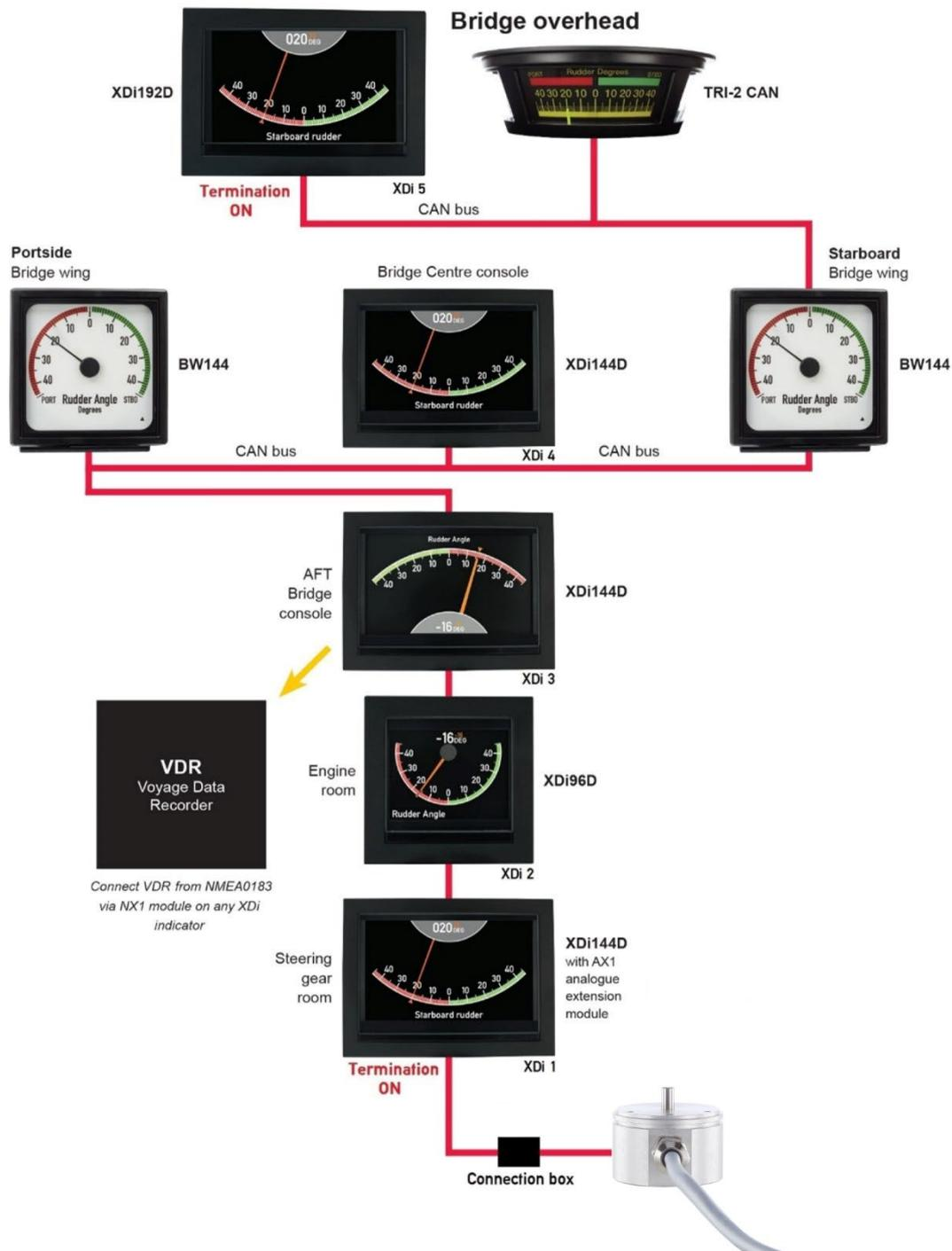
All the XDi indicators receive CAN data directly from the angle transmitter.
