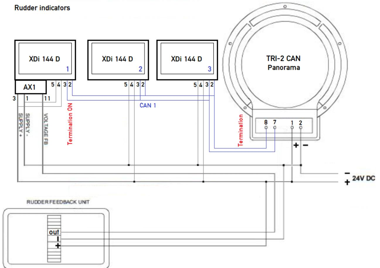
Remember to terminate the bus in both ends with a 120  $\Omega$  resistor when using CAN bus. The build in termination resistor can be activated by a switch located between the Power/CAN connectors.
