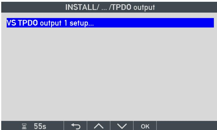
All rudder angle indicators in the standard rudder library has a VS02 profile that is prepared for transmission of the actual rudder angle value. In this case there is only one TPDO output defined. Press OK.
