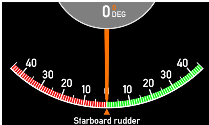
In this example the XDi system can receive the commanded rudder angle via CAN either in a TPDO with COB-ID 0x1A1 (Byte 0 and 1: value +/-1800) or via XDi-net format.
