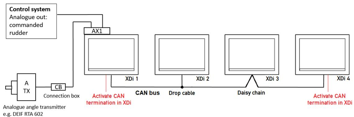
The standard terminal block, with a single row of 5 screw terminals, is well suited for a drop cable connection. Daisy chaining requires two wires to be mounted in each terminal location.
