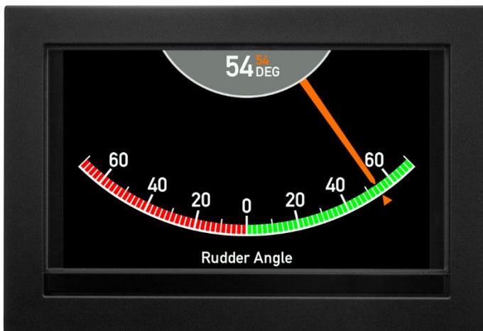
All the XDi rudder indicators can show both the actual rudder angle and the commanded rudder position (or the rudder setpoint). If commanded data is not available, the commanded rudder presentation must be disabled from the XDi installation menu.
