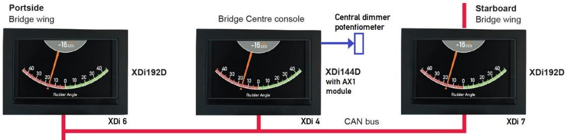
For the XDi units located in the steering gear room and engine control room, a fixed dimmer level and dimmer group “Local” is often used. Local means that dimming is not controlled via the CAN bus.
