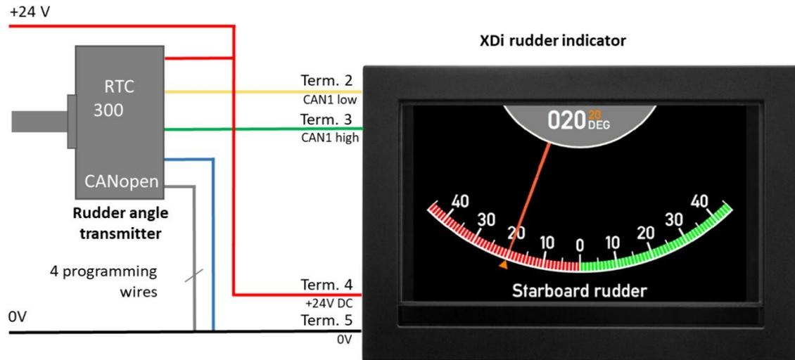
Connecting RTC to XDi via CAN bus 1
