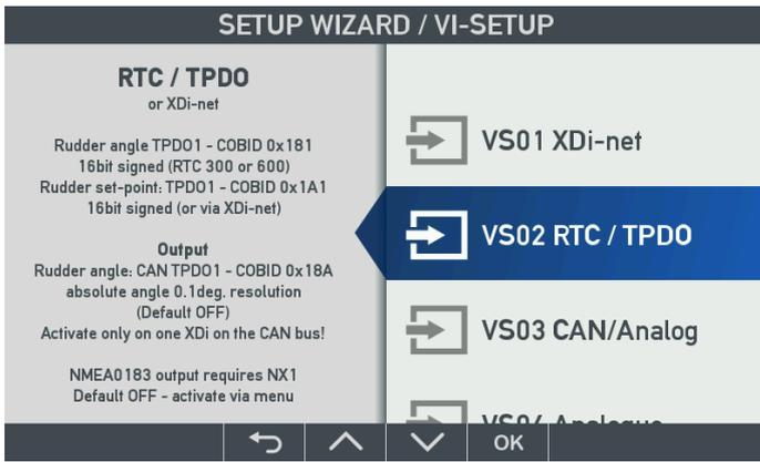
**VS02** profile is intended for use in a CAN bus system with a CAN angle transmitter connected as data source for rudder angle and another CAN bus parameter containing the commanded rudder value. The commanded rudder indicator can be disabled from menu.
