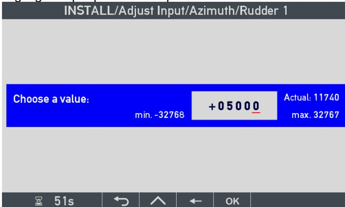
After a few seconds the actual input voltage value (in mV) is shown in the corner, reading 11740mV.
