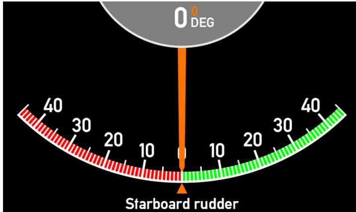
The commanded rudder presentation must be disabled on all XDi indicators where you do not want to use this feature. If it is not disabled on all units, then it is presented as an out of range fixed value, or as data loss if the unit uses a CAN bus data input.
