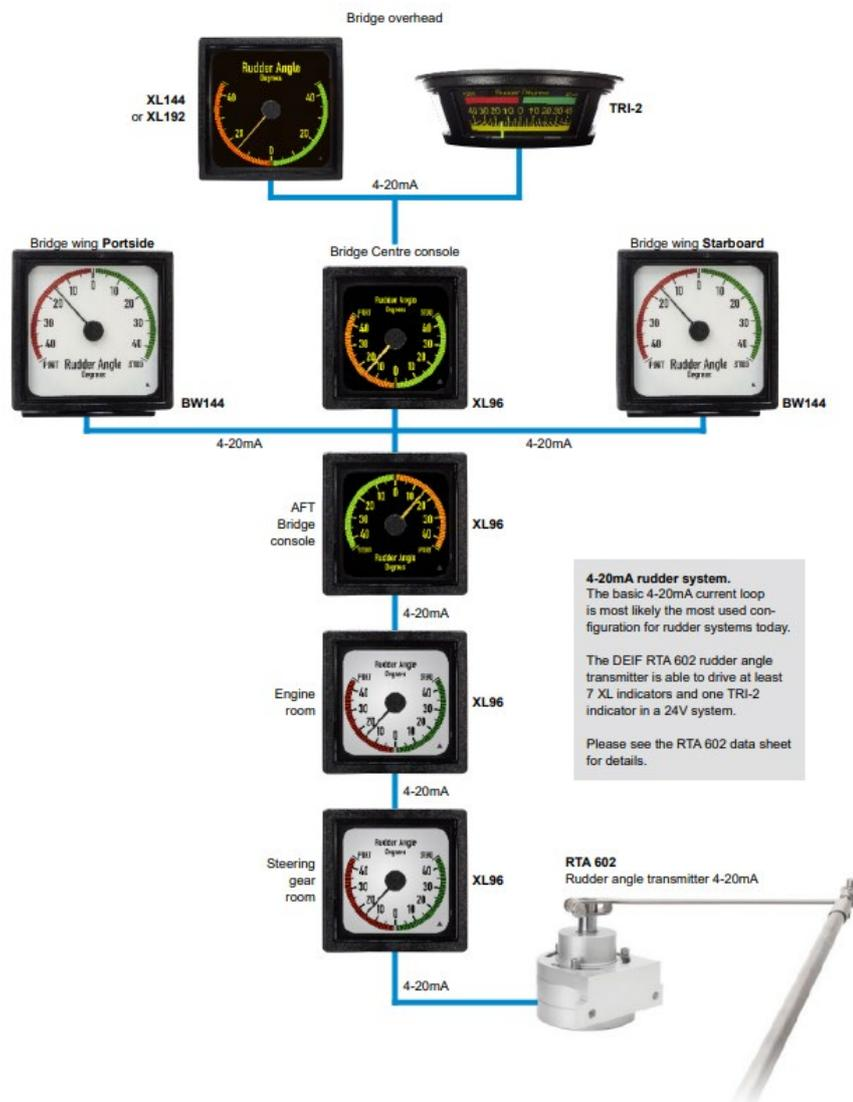
In rudder indicator systems with many indicators, it is always a good idea to make a load calculation to make sure that there is sufficient margin to run the system under all conditions.
