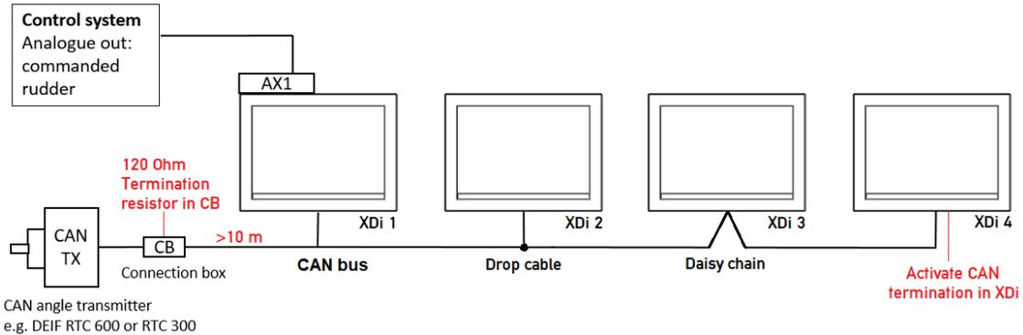
If the cable from the CAN angle transmitter is less than the maximum allowed drop cable length (10 m @125 kbps), then the CAN bus can be terminated using the internal terminations in XDi 1 (left side) and XDi 4 (right side).
