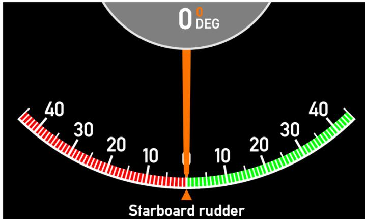
In this example the XDi system can receive the commanded rudder angle as an analogue 4-20 mA signal connected to the AX1 module on the XDi in the steering gear room (XDi 1). XDi 1 will scale the input and distribute it automatically via XDi-net (CAN) to all the other XDi units in the system.
