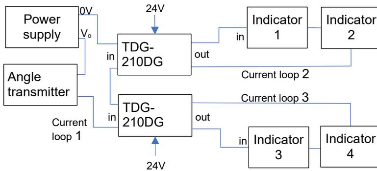
A lost connection to indicator 1 causes indicator 1 and 2 to stop working, but indicator 3 and 4 are not affected.
