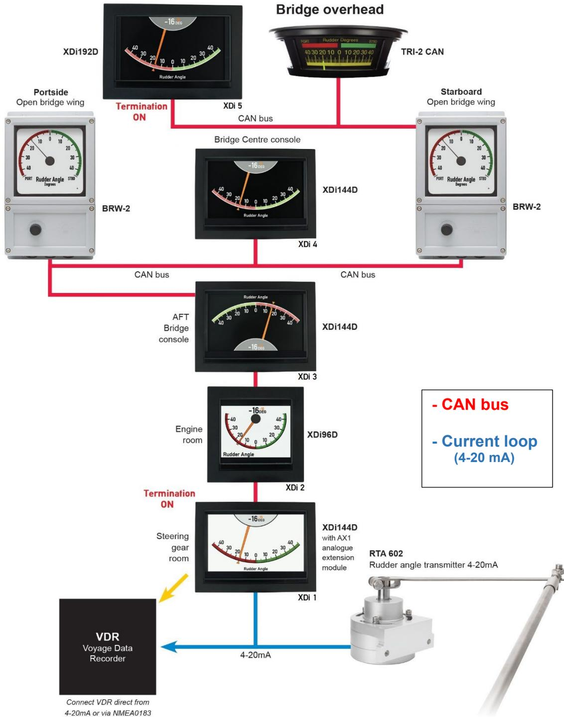
XDi 1, located in the steering gear room, is equipped with an AX1 analogue extension module to which the 4-20 mA signal from the RTA 602 is connected. This XDi unit not only presents the
