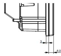
Front frame is 6.0 mm, and the IP66 gasket adds 3 mm to the height.
