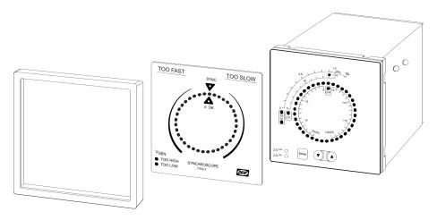
To get access to the settings, remove the front frame and the front foil.
