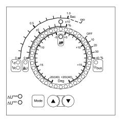
The CSQ-3 can be operated in two different modes: 'Normal mode' and 'setting mode'. Normal mode is used to display measuring values, and setting mode is used to view the settings or change them to the desired functionality.
