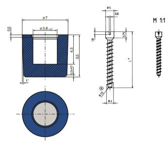
Busbar mounting screw, screw length (L) 25, 32, 36, 46, 54, 80 mm, torque 0.5 Nm
