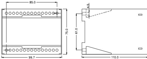
TAS-321DG is designed for panel mounting, being mounted on a 35 mm DIN rail, or by means of two 4-mm screws.
