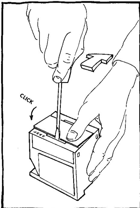
Press with a screwdriver as indicated by the arrow and press the front panel down with your thumb, simultaneously. It is recommended that one side of the front panel snaps into place before the other.
