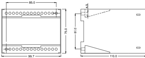
TAS-311DG is designed for panel mounting, being mounted on a 35 mm DIN rail, or by means of two 4-mm screws.
