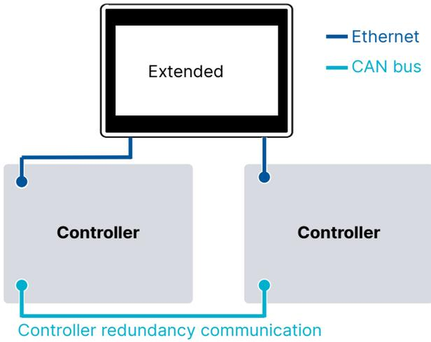
You can connect one TDU to both the master (primary) and the redundant controller. Configure the IP addresses for the *Master* and *Slave* controllers in the *Communication settings* box (*Setup > Connect to controller*).
