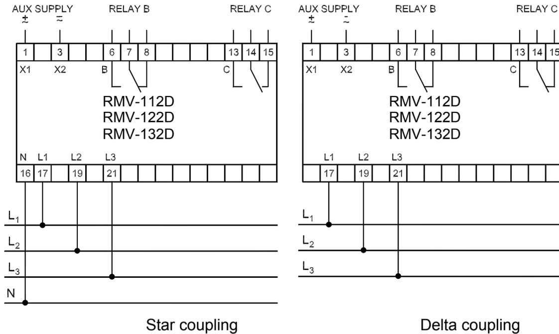
Please note the difference between relays for delta coupling and for star coupling. The coupling is stated on the label.
