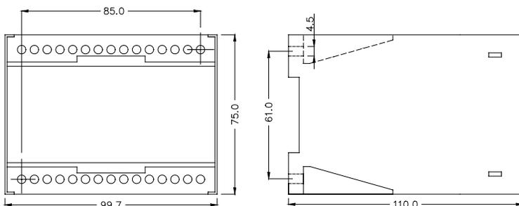
The RMV-112D is designed for panel mounting, being mounted on a 35 mm DIN rail, or by means of two 4-mm screws.
