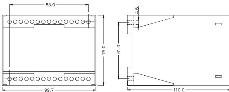
The RMC-132D is designed for panel mounting, being mounted on a 35 mm DIN rail, or by means of two 4-mm screws.
