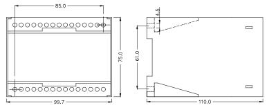
The RMC-122D is designed for panel mounting, being mounted on a 35 mm DIN rail, or by means of 2 off 4 mm screws.
