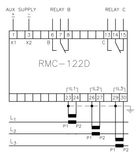
The auxiliary supply connection may be protected by a 2A fuse.
