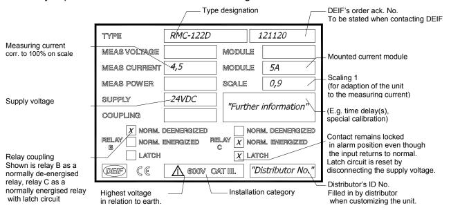
Note 1: Calculation of measuring current: module x scale = meas. current.
