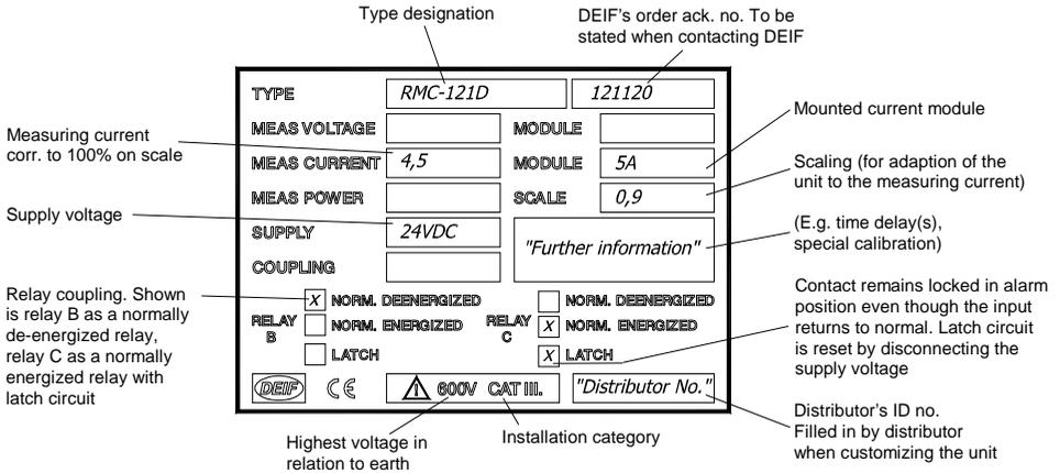
**Note:** The relay is provided with a 200 ms power-up relay, ensuring correct function of the relay on connection of the auxiliary voltage. Normally energized contacts ("NE") are not activated (contact does not open/close) until 200 ms after connection of the auxiliary voltage.
