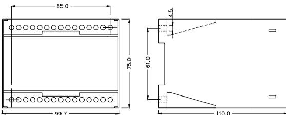
The RMC-121D is designed for panel mounting, being mounted on a 35 mm DIN rail, or by means of two 4-mm screws.
