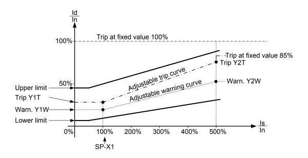
The trip/warning pickup characteristics are shown above. They are a function of:
