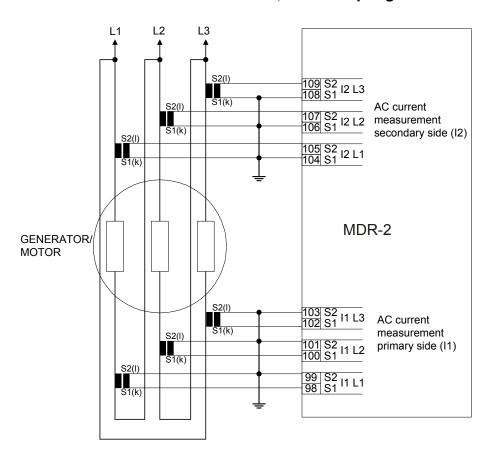
**NOTE** The nominal current setting is to be the name plate current divided by  $\sqrt{3}$ . **NOTE** The ground connections can be connected to S1 or S2 as needed.
