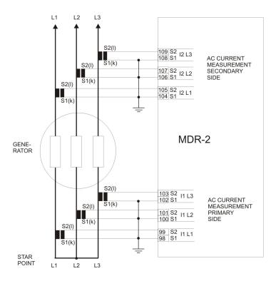
**NOTE** The ground connections can be connected to S1 or S2 as needed.
