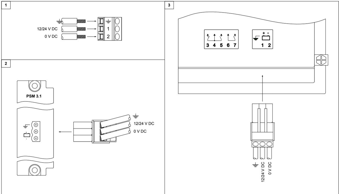
1. Connect the wires from the power supply to the power terminal blocks for the controllers and the display units.
