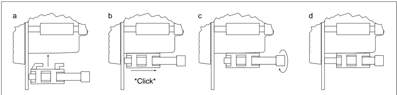
1. Check the available space at the vertical mounting position. There should be a minimum of 20 mm (0.79 inches) of free space above and below the controller for ventilation.
