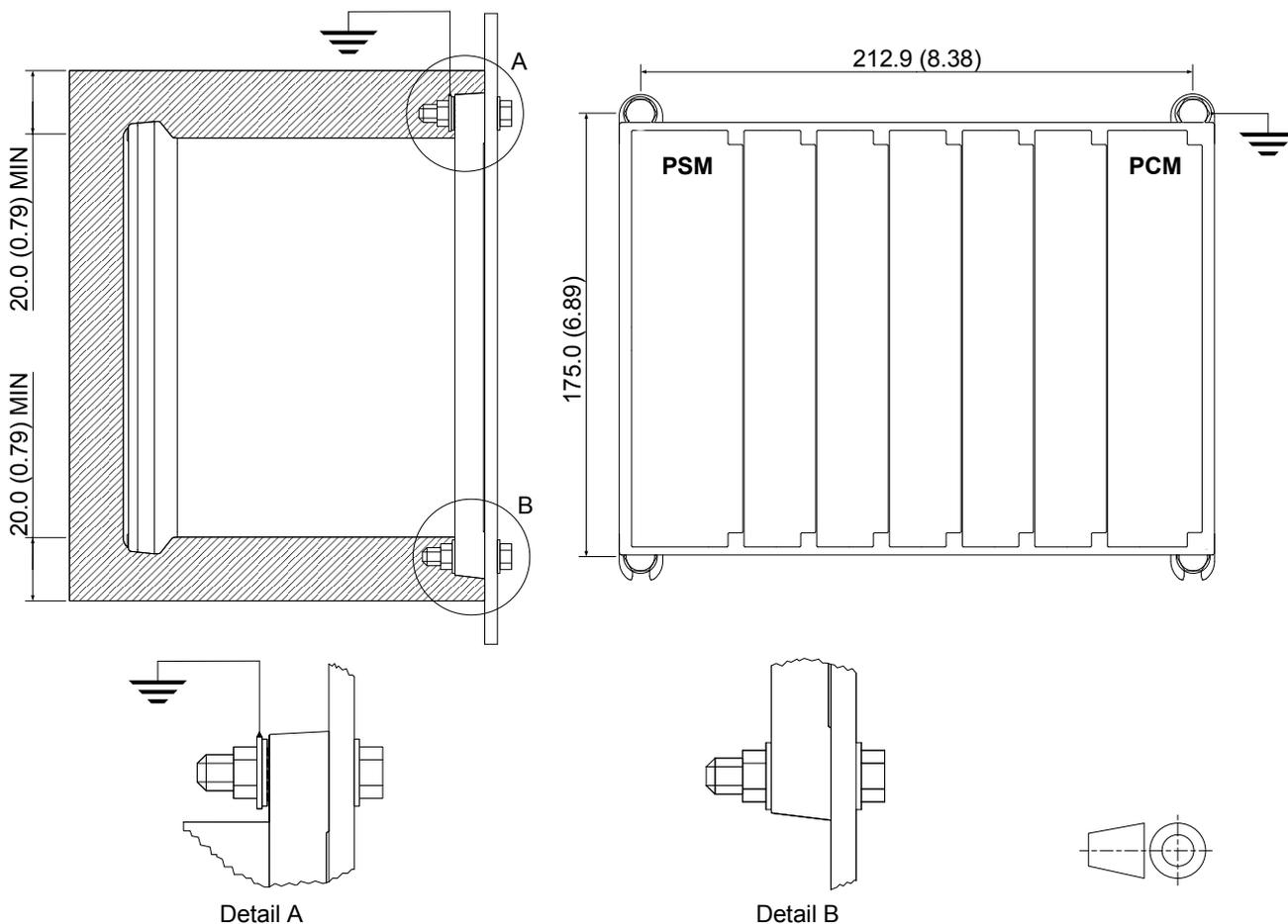
1. Check the available space at the vertical mounting position. There should be a minimum of 20 mm (0.79 inches) of free space above and below the controller for ventilation.
