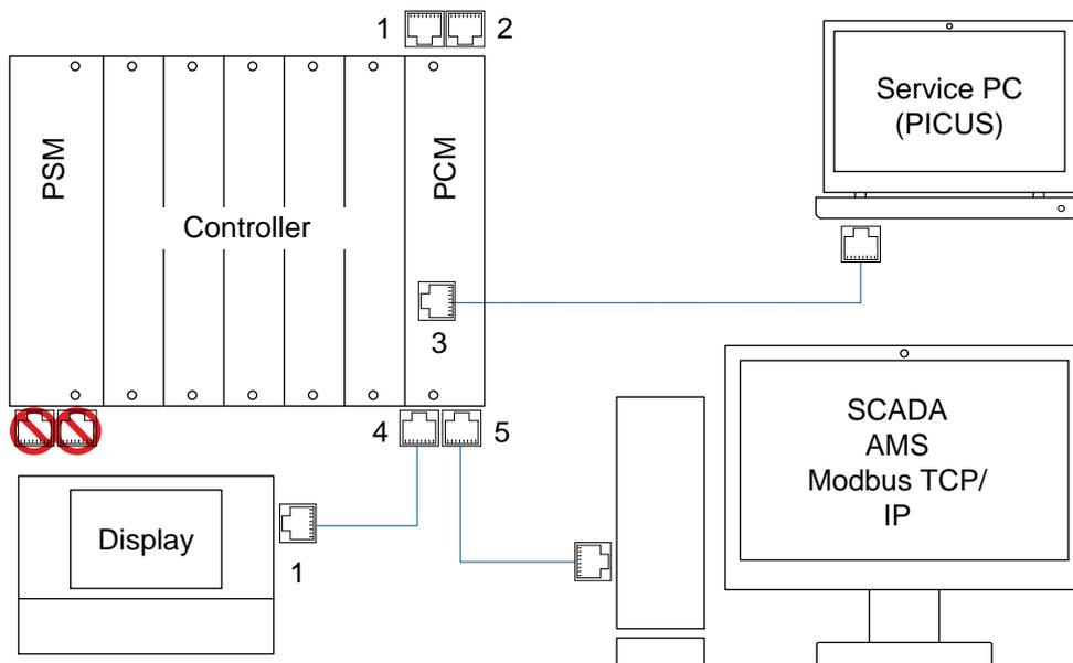
Connect the communication wires according to the system design.
