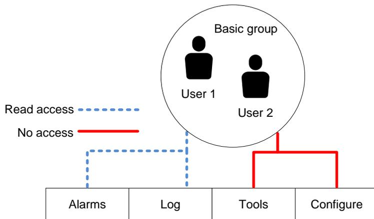
In the diagram, **User 1** and **User 2** are members of the **Basic group**. They have read access to the **Alarms**, and **Log**, but they have no access to the **Tools** or **Configure** functions.
