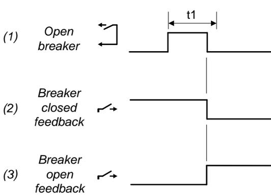
t1 Pulse on (*Parameters > Breakers > Generator breaker > Pulse time ON*)
