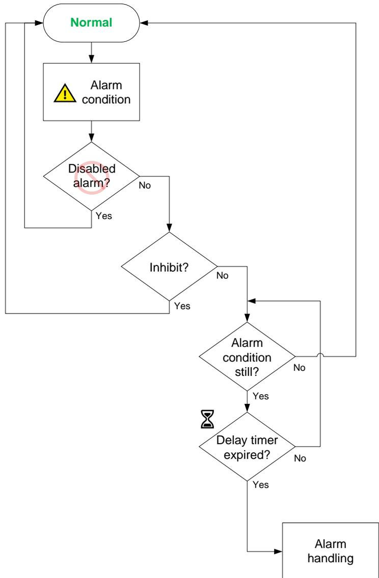
When an alarm condition is met (typically, the operating value reaches the *Set point*), then the controller starts the *Time delay*. During this period the controller checks whether the *Alarm condition* is still present. If not, the alarm returns to normal.
