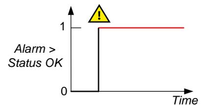
By default the *Status OK* alarm output is configured to terminals 3 and 4 of the power supply module of the controller. This configuration cannot be removed or changed.
