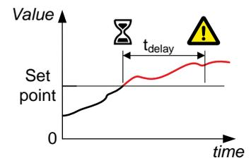
Configure the parameters under **Configure > Parameters > Generator > Current protections > Over-current**.
