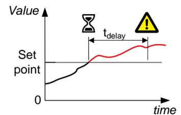
Configure the parameters under **Configure > Parameters > Non-essential load trip > Trip # > Reactive overload**.
