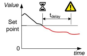
Configure the parameters under **Configure > Parameters > Power supply > PSM 1 > Low voltage alarm.**
