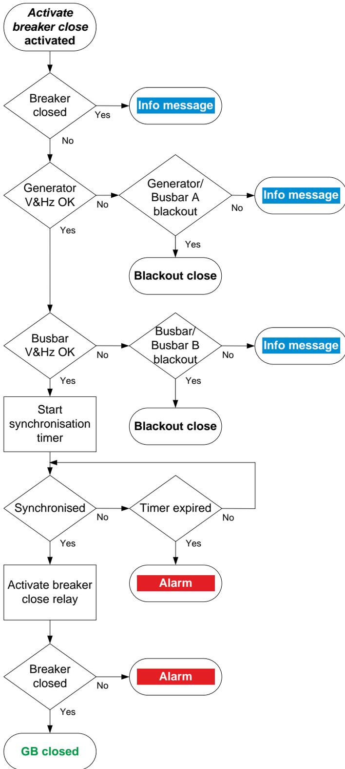
1. When the breaker close relay is activated, the controller checks whether the generator breaker is closed. If the generator breaker is already closed, the sequence stops, and an info message is shown.
