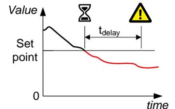
Configure the parameters under **Configure > Parameters > Generator > Frequency protections > Under-frequency**.
