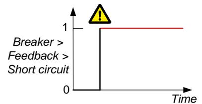
Configure the parameters under **Configure > Parameters > Breakers > [Breaker] > Short circuit**.
