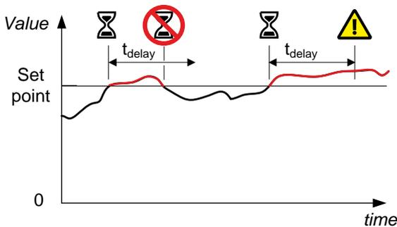
**Figure 4.4** Delay for a high alarm based on a digital input
