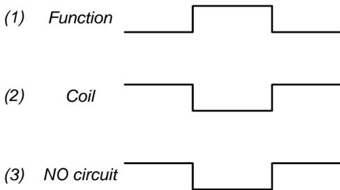
1. **Function:** The digital output function assigned to the terminals. The controller software activates the function. For example: *Breaker > Command > Close*.
