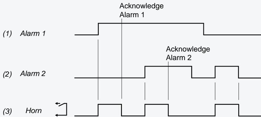
The horn output is deactivated when both alarms are acknowledged (even though both alarms are still active).
