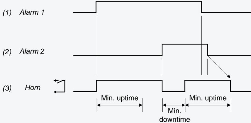
The horn output is deactivated for the *Minimum down time* when *Alarm 2* becomes active. To fulfil the *Minimum up time* requirement, the horn output remains active for a short time after both alarms become inactive.
