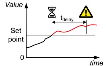
Configure the parameters under **Configure > Parameters > Generator > Voltage protections > Over-voltage**.
