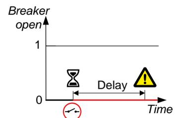
Configure the parameters under **Configure > Parameters > Breakers > Generator breaker > Opening failure**. The alarm is always enabled.
