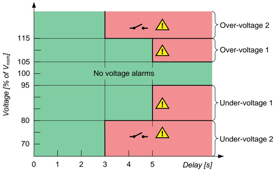
If the operation is in the green area, the controller does not activate any busbar voltage alarms.
