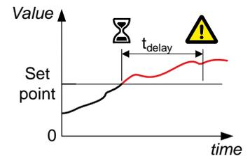
Configure the parameters under **Configure > Parameters > Busbar > Voltage protections > Over-voltage**.
