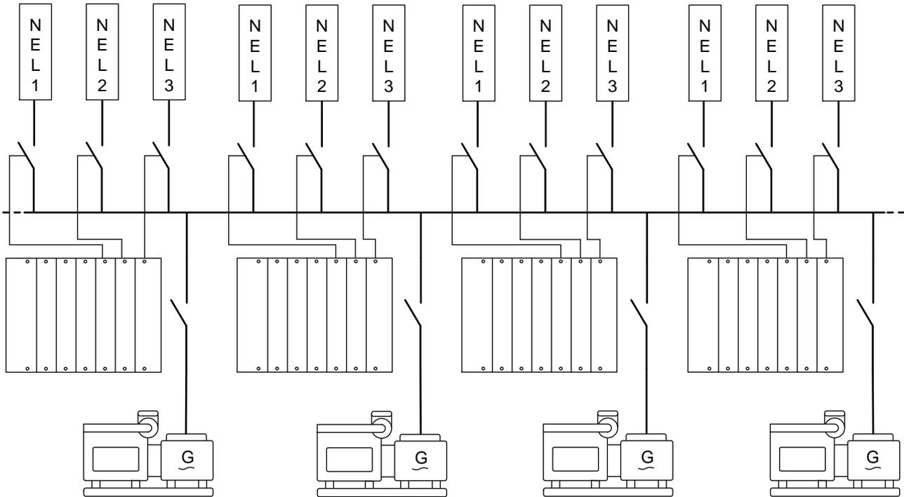
DEIF recommends that you connect each non-essential load to each controller, so that any controller can trip the non-essential loads. As a minimum, each non-essential load should be connected to at least two controllers. However, it is possible to connect each controller to up to three non-essential loads, with no interaction from the other controllers.
