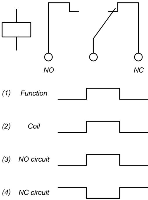
1. **Function:** The digital output function assigned to the terminals. The controller software activates the function. For example: *Breaker > Command > Close*.
