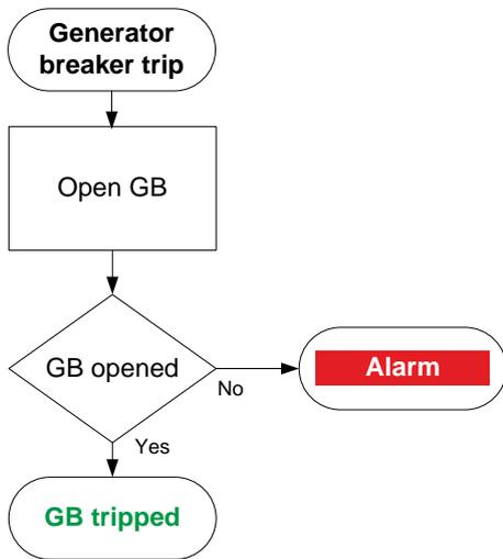
1. When a trip is required, the controller activates the *Generator breaker > Control > Open* output to open the breaker.
