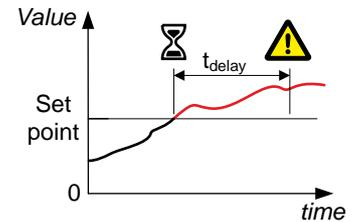
Configure the parameters under **Configure > Parameters > Busbar > Frequency protections > Over-frequency**.
