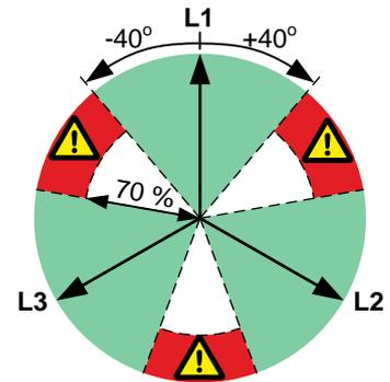
There are two alarms for each controller. These alarms correspond to the controller's AC measurements. There is one alarm for the voltage from the [Controlled equipment] (terminal A), and another alarm for the voltage on the [Busbar] (terminal B).
