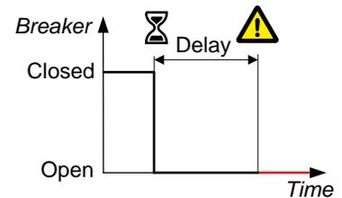
Configure the parameters under **Configure > Parameters > Breakers > [Breaker] > Tripped (external)**.
