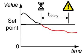
Configure the parameters under **Configure > Parameters > Busbar > Voltage protections > Under-voltage**.
