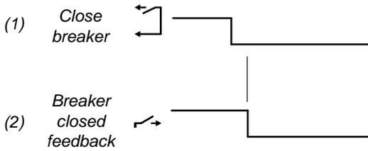
1. **Close breaker:** *Generator breaker > Control > Close* (digital output). The controller deactivates this output to open the breaker.
