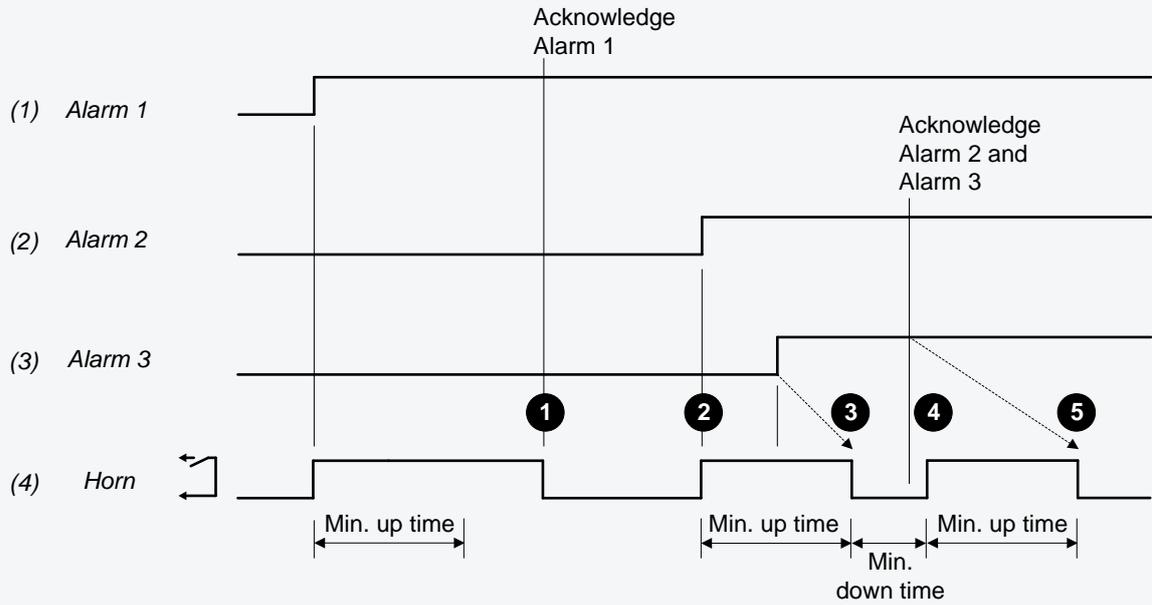
1. The horn output is deactivated when alarm 1 is acknowledged. There is no *Minimum down time* when the alarms are acknowledged.
