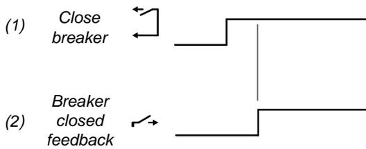
1. **Close breaker:** *Generator breaker > Control > Close* (digital output). The controller activates this output to close the breaker.
