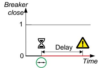
Configure the parameters under **Configure > Parameters > Breakers > [Breaker] > Closing failure**. This alarm is always enabled.
