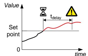
Configure the parameters under **Configure > Parameters > Non-essential load trip > Trip # > Overload 1** .
