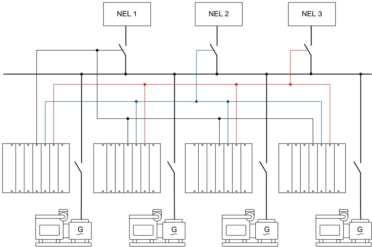
For redundancy and secure operation, DEIF strongly recommends that all controller NEL trip settings are identical.
