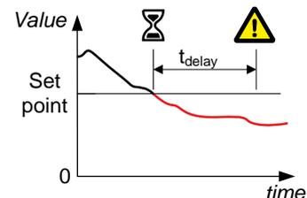
Configure the parameters under **Configure > Parameters > Busbar > Frequency protections > Under-frequency**.
