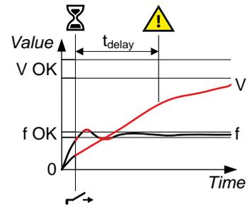
See **Configure > Parameters > AC configuration > [Controlled equipment]**. The parameters that the alarm is based on are under **Voltage and frequency OK**. The alarm is configured under **Voltage or frequency not OK**.
