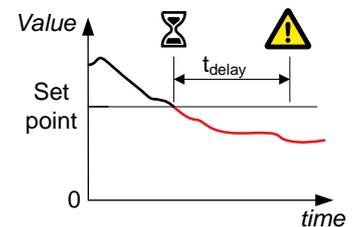
Configure the parameters under **Configure > Parameters > Generator > Voltage protections > Under-voltage**.
