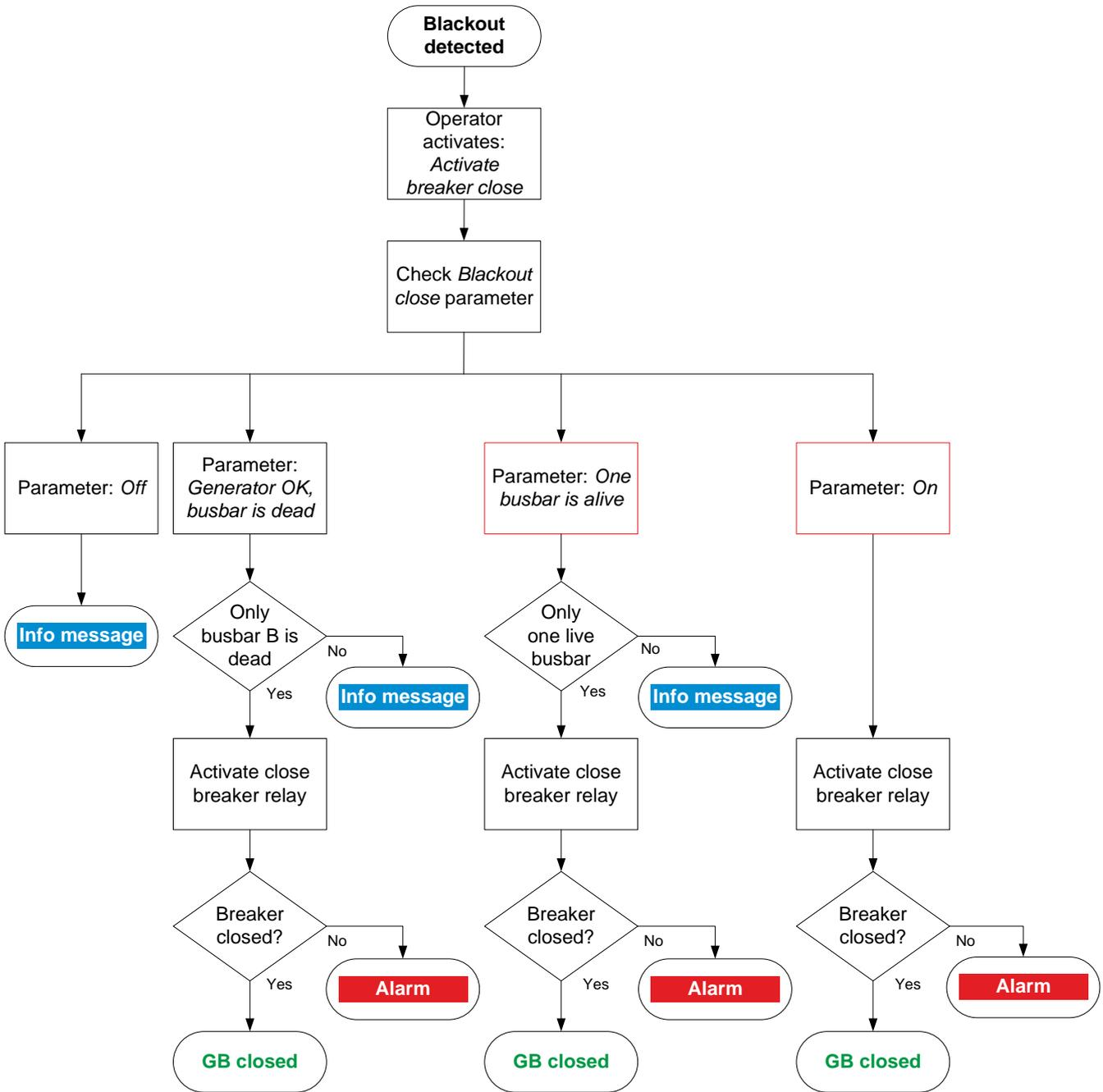
1. When there is a blackout, the operator has to activate the *Activate breaker close* digital input. When the controller detects that one or both of the busbars have a frequency and voltage that are not in range, the blackout close procedure starts.
