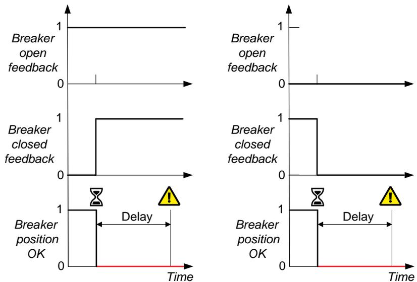
Configure the parameters under **Configure > Parameters > Breakers > Generator breaker > Position failure**.
