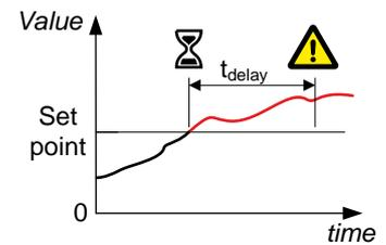
Configure the parameters under **Configure > Parameters > Generator > Voltage protections > Voltage unbalance**.
