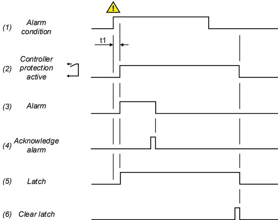
1. **Alarm condition:** When an alarm condition occurs, an alarm dependent delay timer activates. If the alarm condition occurs for longer than the delay timer, the protection activates.
