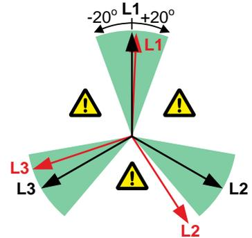
Configure the parameters under **Configure > Parameters > Synchronisation > Alarms > Vector mismatch**.
