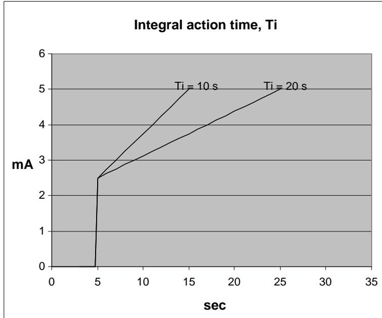
As it appears from the drawing, the output reaches 5 mA twice as fast at a Ti setting of 10 s than with a setting of 20 s.
