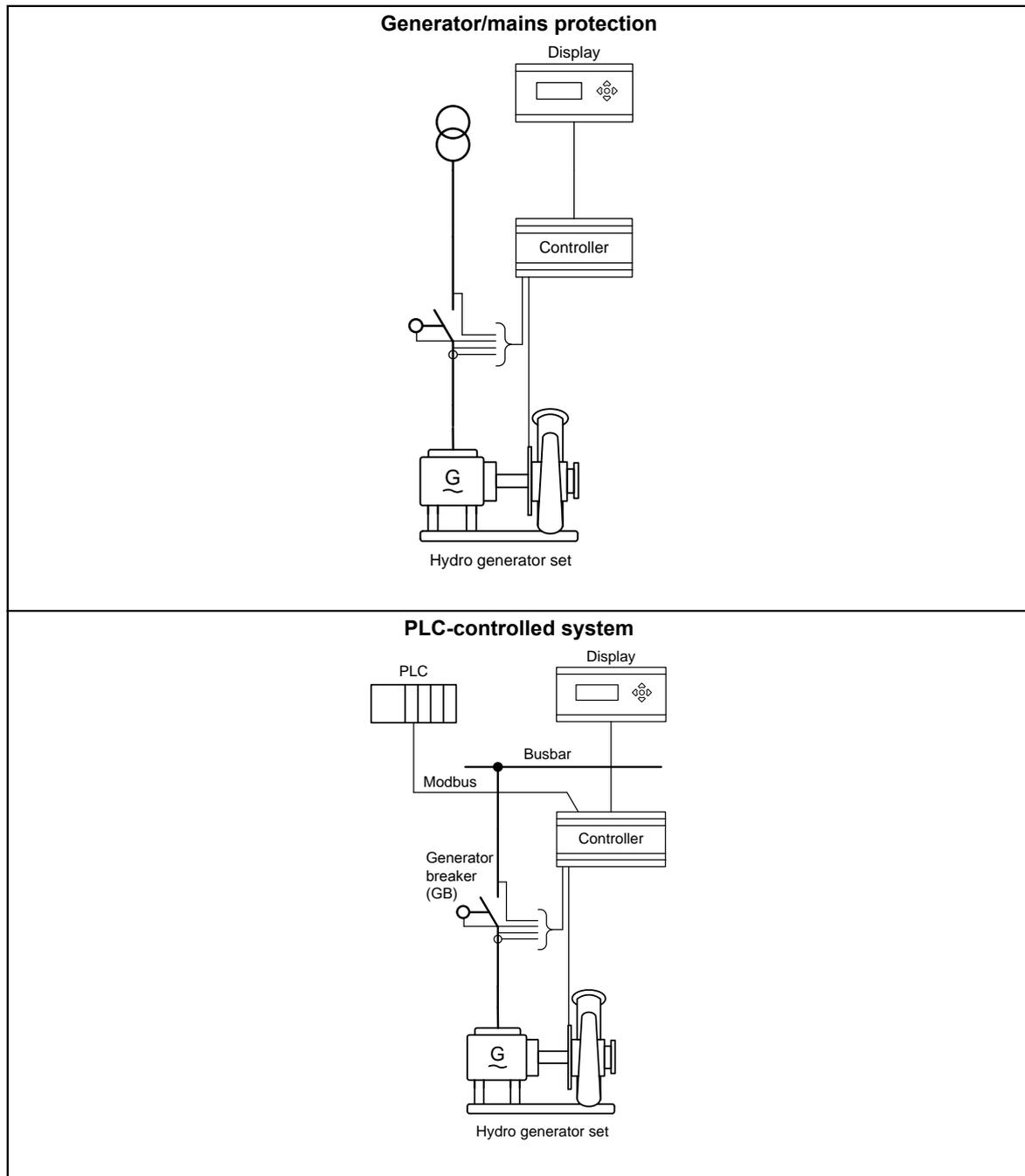
**i** The GPU-3 Hydro can be used in simple or complex applications. The above shows very simple applications only, but due to the flexibility, the GPU-3 Hydro can be used in all types of applications.
