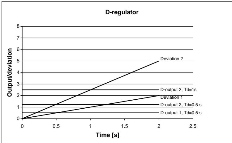
Deviation 1: A deviation with a slope of 1.
