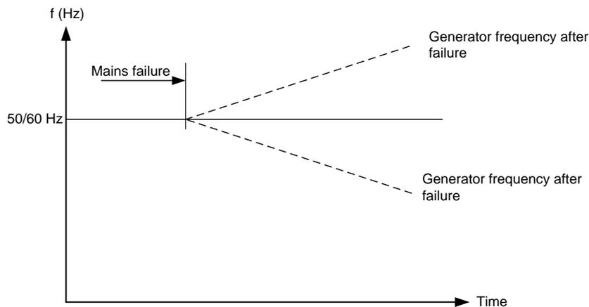
So, a dramatic drop/increase of frequency over time is a mains failure. The df/dt setting is made in Hz/s.
