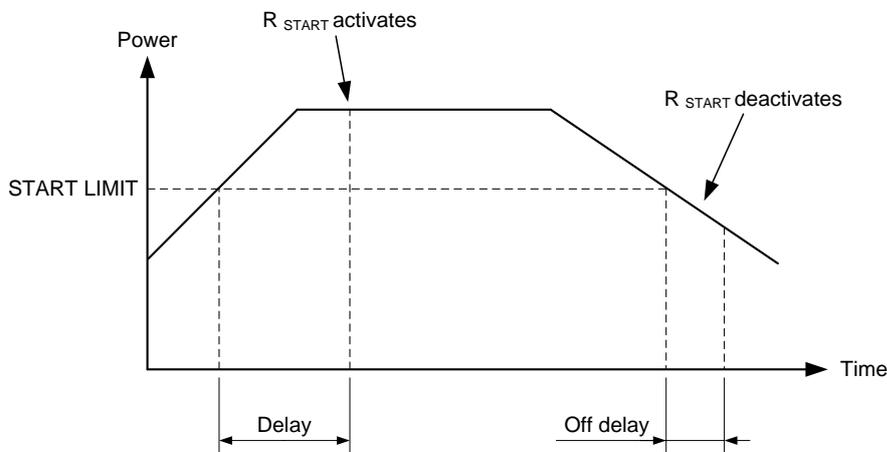
The load-dependent start relay reacts based on the power measurement of the GPU together with the breaker closed feedback.
