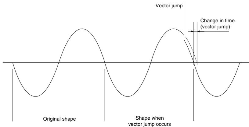
Again, comparing the half-sine curve time duration with the previous ones, a sudden change in time can be detected. This is the vector jump.
