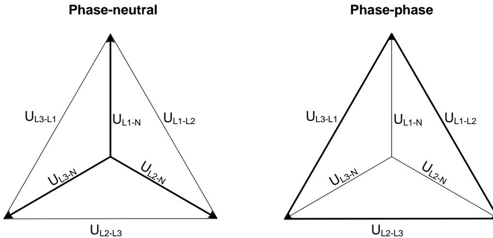
As indicated in the vector diagram, there is a difference in voltage values at an error situation for the phase-neutral voltage and the phase-phase voltage.
