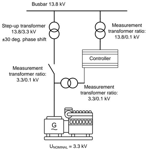
When used for synchronising, the GPU-3 uses the ratio of the nominal voltages of the generator and the busbar when calculating the AVR setpoint and the voltage synchronising window ( $dU_{MAX}$ ).
