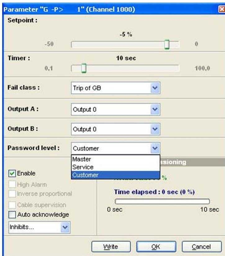
The password level can also be changed from the parameter view in the column "Level".
