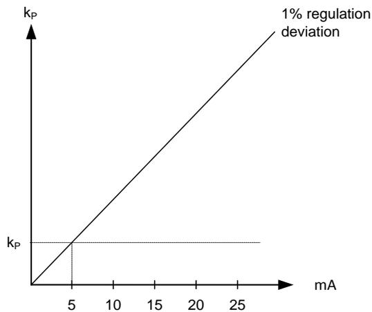
A 1% regulation deviation occurs. With the  $K_p$  setting adjusted, the deviation causes the output to change 5 mA. The table shows that the output will change relatively much, if the maximum speed range is low.
