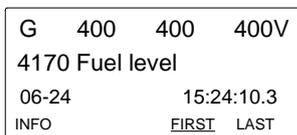
The specific alarm or event is shown in the second line. In the example above the fuel level alarm has occurred. The third line shows the time stamp.
