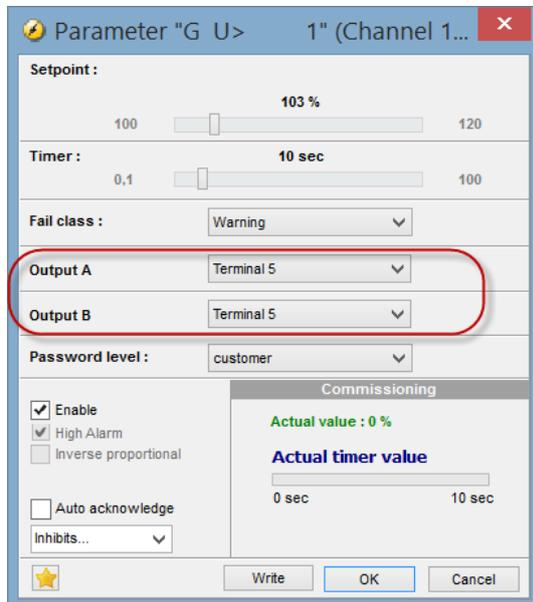
The timer configured in the alarm window is an ON delay that determines the time during which the alarm conditions must be met before activation of any alarms or outputs.
