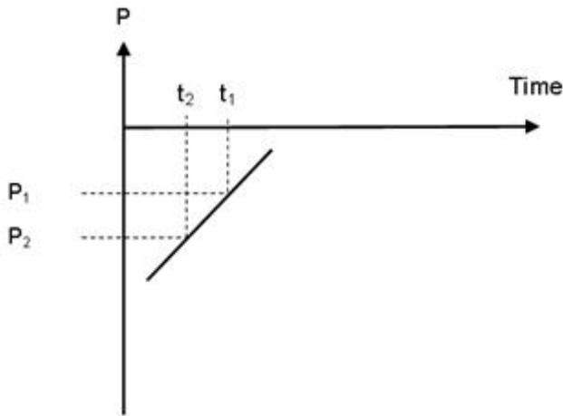
The diagram above shows that when the reverse power increases from P1 to P2, the delay will also be shorter.
