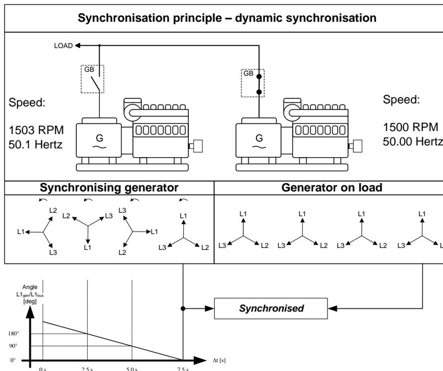
In the above example, the synchronising genset is running at 1503 RPM ~ 50.1 Hz. The generator on load is running at 1500 RPM ~ 50.0 Hz. This gives the synchronising genset a positive slip frequency of 0.1 Hz.
