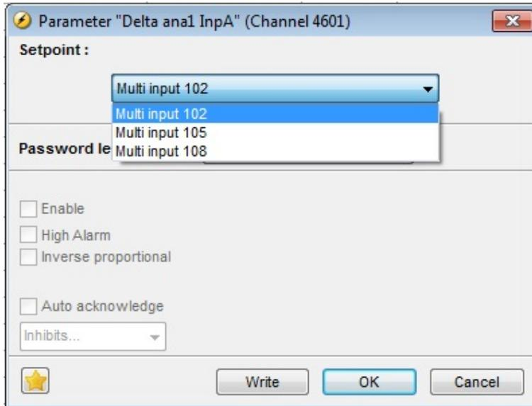
Each alarm can be configured in two alarm levels for each differential measurement between the analogue inputs A and B as follows. The configurations are done in menus 4610-4650 and 4680-4730.
