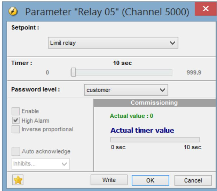
The timer in the image above is an OFF delay, meaning that when the alarm level is OK again, the relay will remain activated until the timer runs out. The timer is only effective when it is configured as "Limit relay". If it is configured to any "Alarm relay", the relay is deactivated instantly when the alarm conditions disappear and it is acknowledged.
