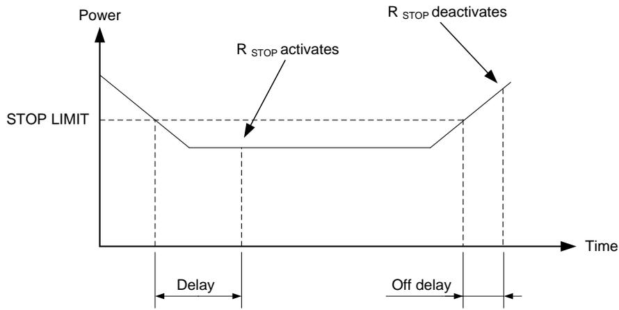
The load-dependent start relay reacts based on the power measurement of the GPU-3 together with the breaker closed feedback.
