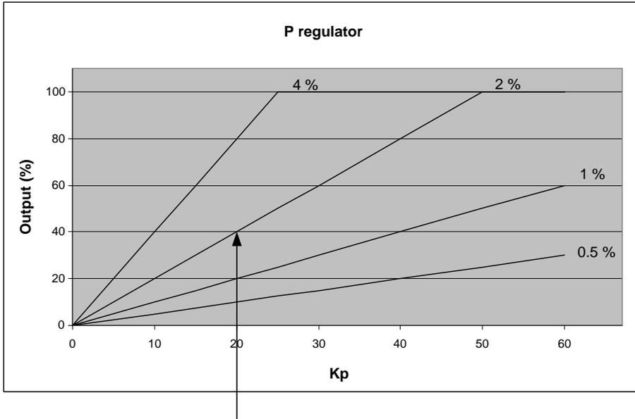
In this example we have a 2 percent regulation deviation and an adjusted value of the Kp = 20. The calculated regulator value of the unit is 40 %. Now the pulse length can be calculated with a period time = 2500 ms:
