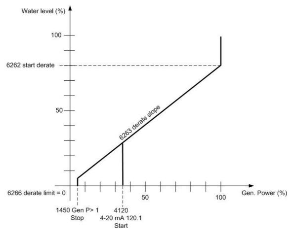
The turbine will start at water level 35 % and stop at generator power 5 %. 100 % output is reached when the water level reaches 80 %.
