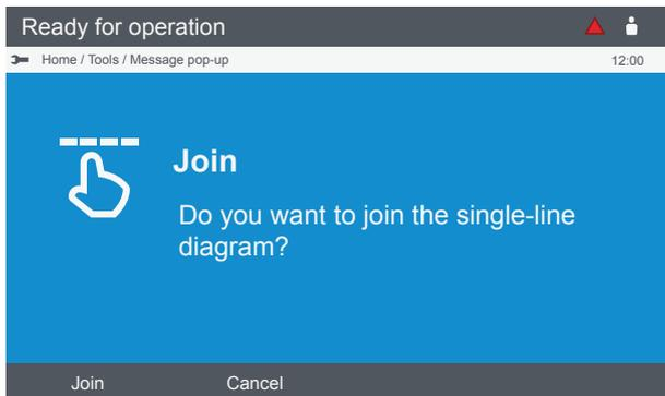
Select **Join** to add the controller to the application single-line diagram.
