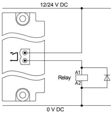
Use a diode size as recommended by the relay supplier.
