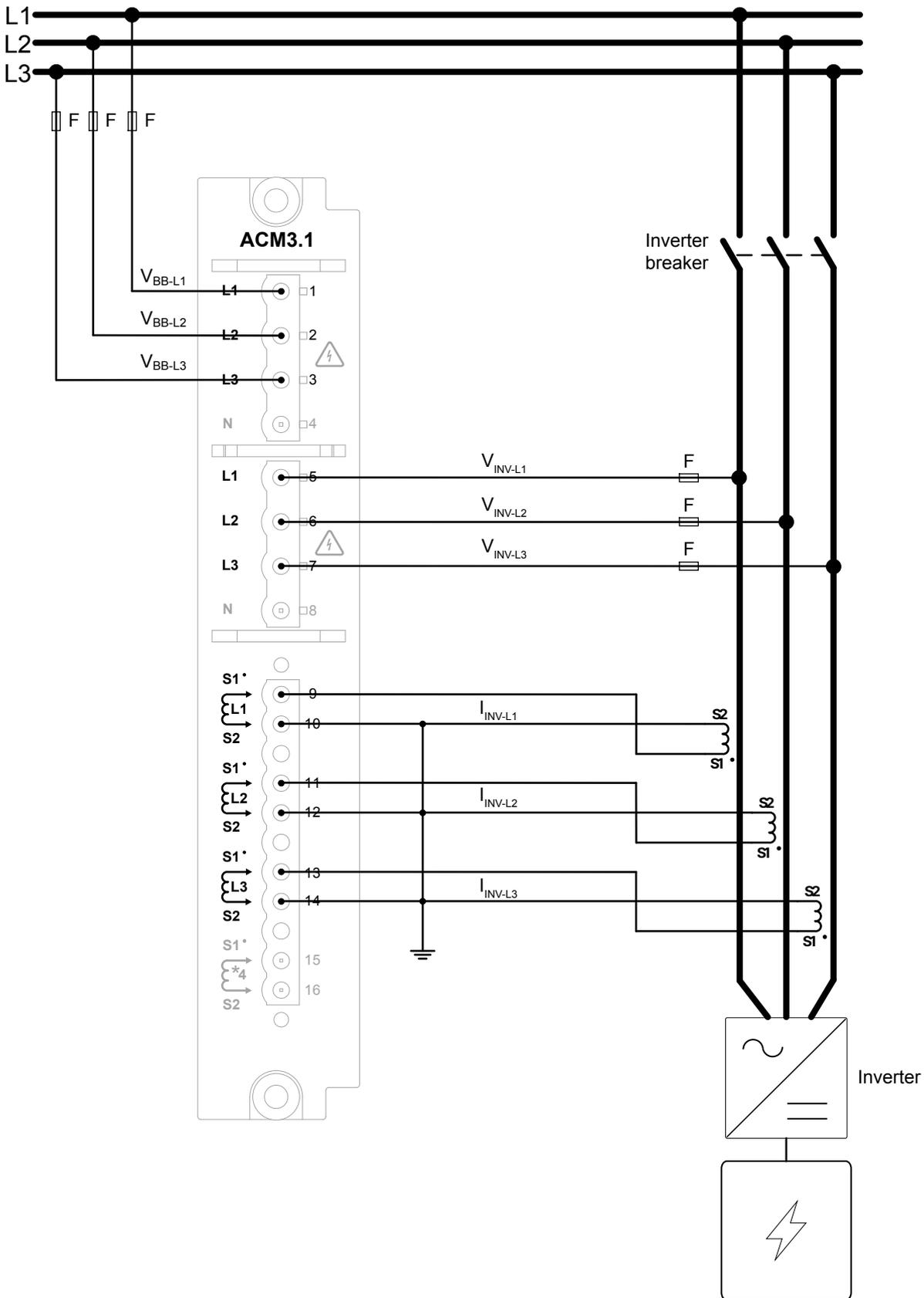
Alternatively, you can ground the S1 side of the current transformers, instead of S2 as shown.
