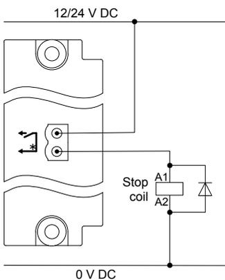
Do not connect the terminals to an alternating current supply. Alternating current will destroy the wire break detection.
