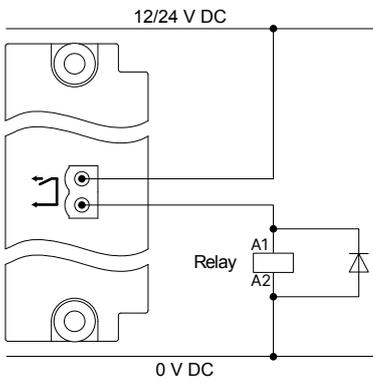
Use a diode size as recommended by the relay supplier.
