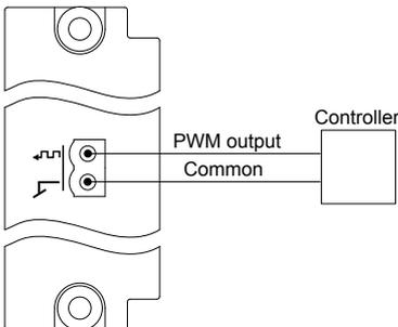
**NOTE** The PWM output is galvanically connected to the first analogue output (terminals 12 and 13) on GAM3.1. This means that wiring errors or noise on either output can affect the other output.
