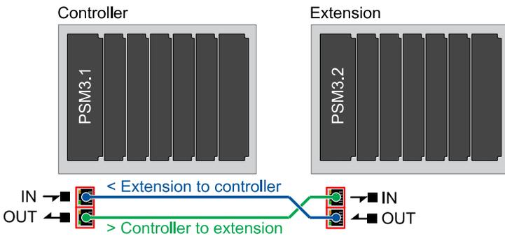
**Ring (redundancy connection)**
