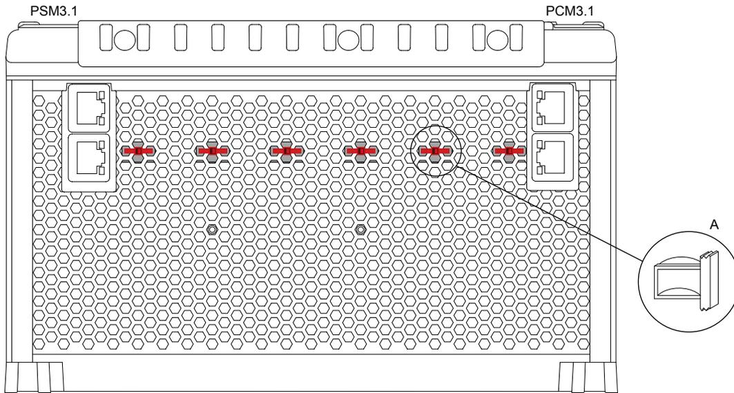
The cable tie slots are inside the rack's aluminium frame. Only use them if the maritime classification societies rules allow the wiring to be secured directly to metal. Alternatively, you can use extra insulation between the rack's frame and the wire.
