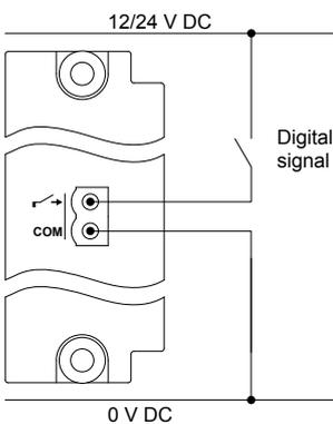
**Figure 4.77** Example: Digital input wiring (common = 12 or 24 V)
