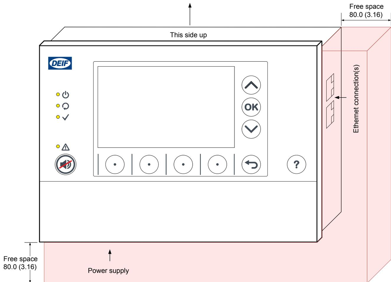
For the Ethernet cables, the bends must not be tighter than the minimum bend radius specified by the cable manufacturers. Make sure there is enough space to the right of the display (as seen from the front) for the Ethernet cables.
