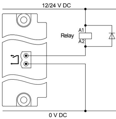
Install a freewheeling diode (
