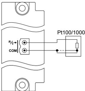
You do not have to connect the third wire (shown by the dashed line). If you want to connect the third wire, connect it to the common, as shown in the diagram.
