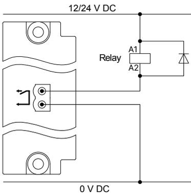
Install a freewheeling diode (
