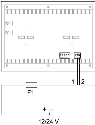
**Figure 4.85** Incorrect wiring of the power supply
