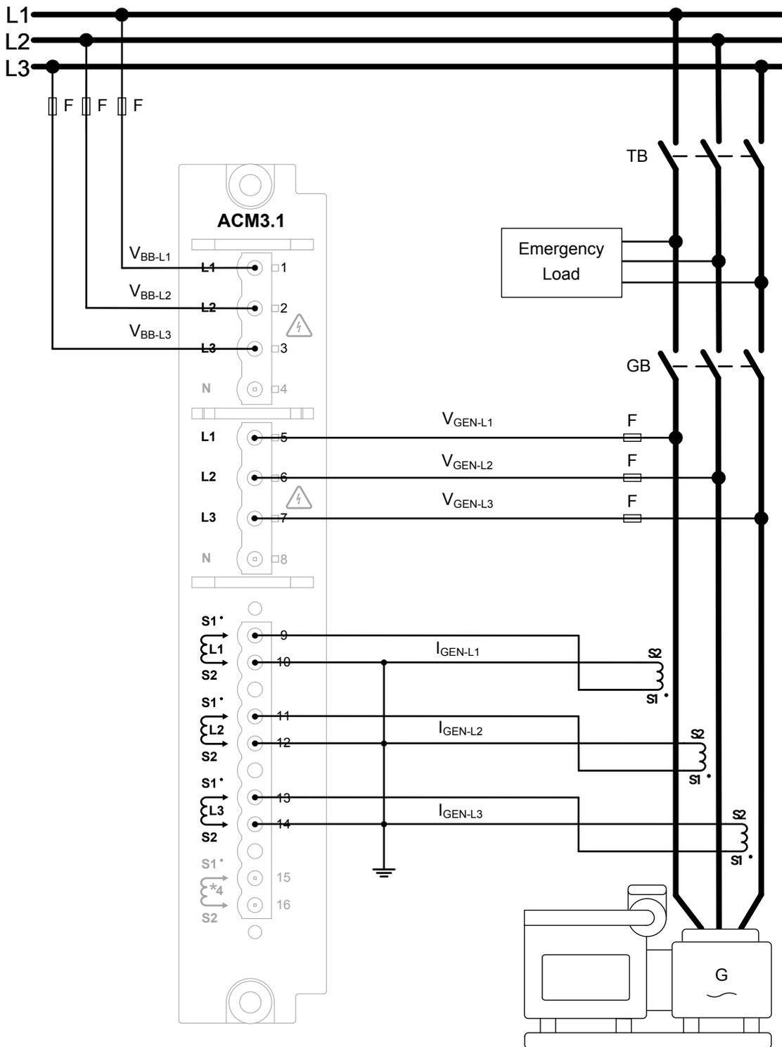
Alternatively, you can ground the S1 side of the current transformers, instead of S2 as shown.
