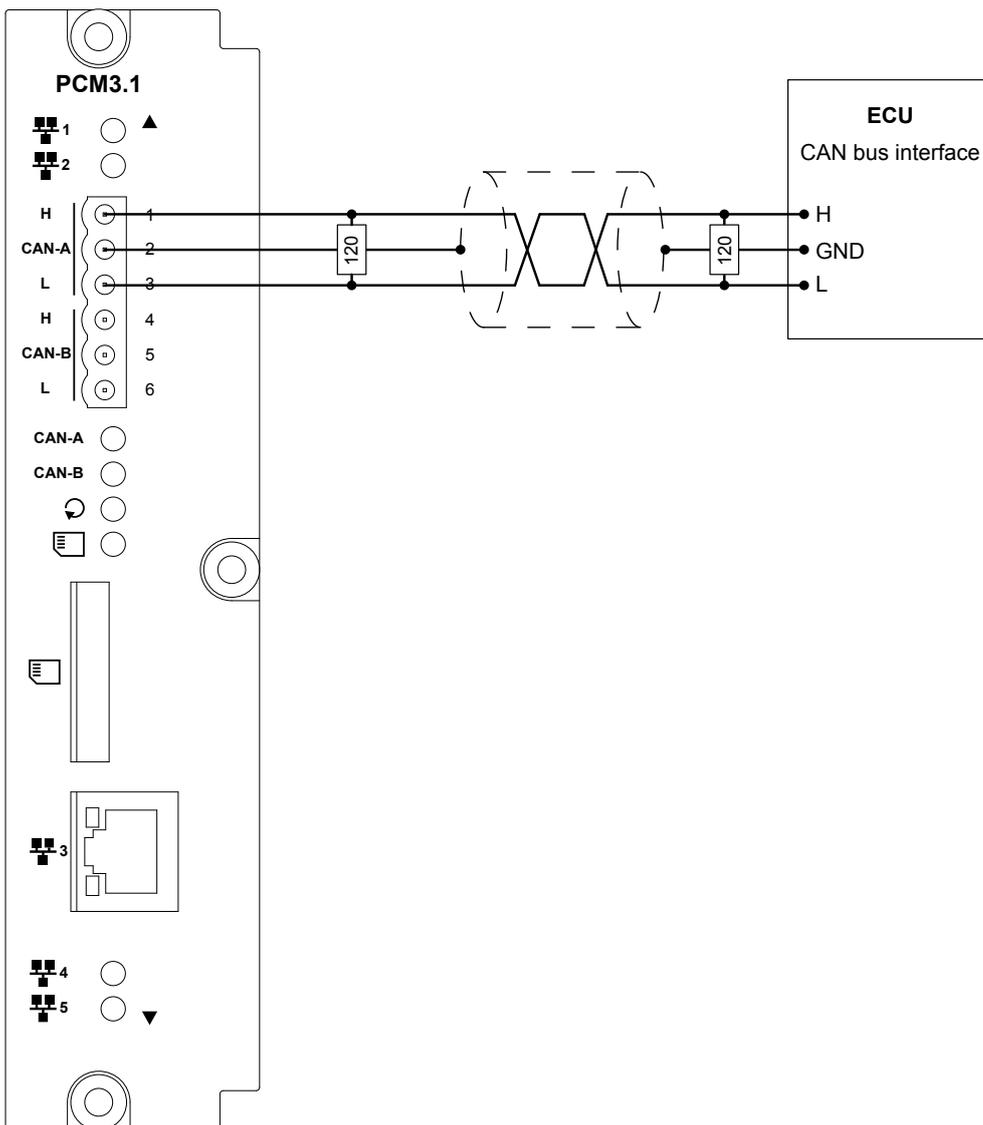
Use 120 Ω (Ohm) shielded twisted pair cable. Terminating resistors at the ends of the cable must be 120 Ω (Ohm).
