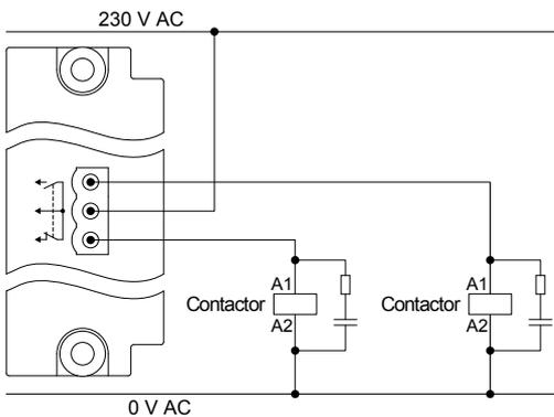
For 230 V AC contactors, we strongly recommend that you use an RC snubber for noise suppression across the contactor.
