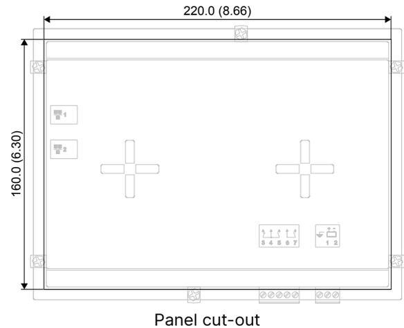
**NOTE** This panel cut-out drawing is meant as a guideline. Use the dimensions given to create your panel cut-out template.
