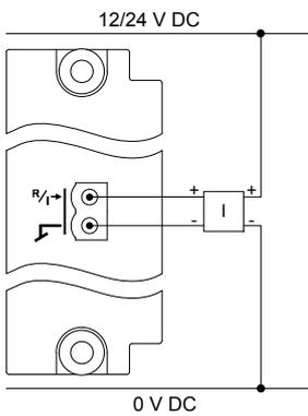
**Figure 4.65** Connection of a passive transducer
