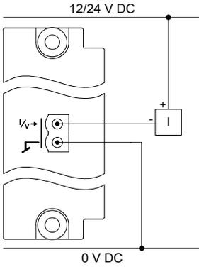
The two analogue inputs on GAM3.1 are galvanically connected. You therefore cannot use the analogue inputs on GAM3.1 in series with each other, for example, if you wanted a backup measurement. If you need two analogue inputs in series, you can use an analogue input on another module in series with an analogue input on GAM3.1, since the modules are galvanically isolated from each other.
