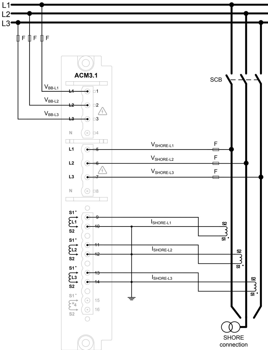
Alternatively, you can ground the S1 side of the current transformers, instead of S2 as shown.
