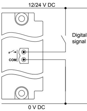
**Figure 4.45** Example: Digital input wiring (common = 12 or 24 V)
