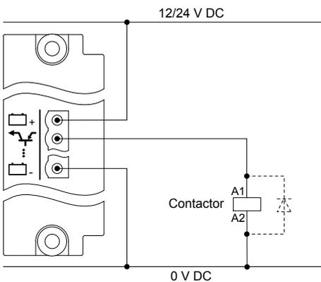
**NOTE** You can install a diode () to reduce electromagnetic interference.
