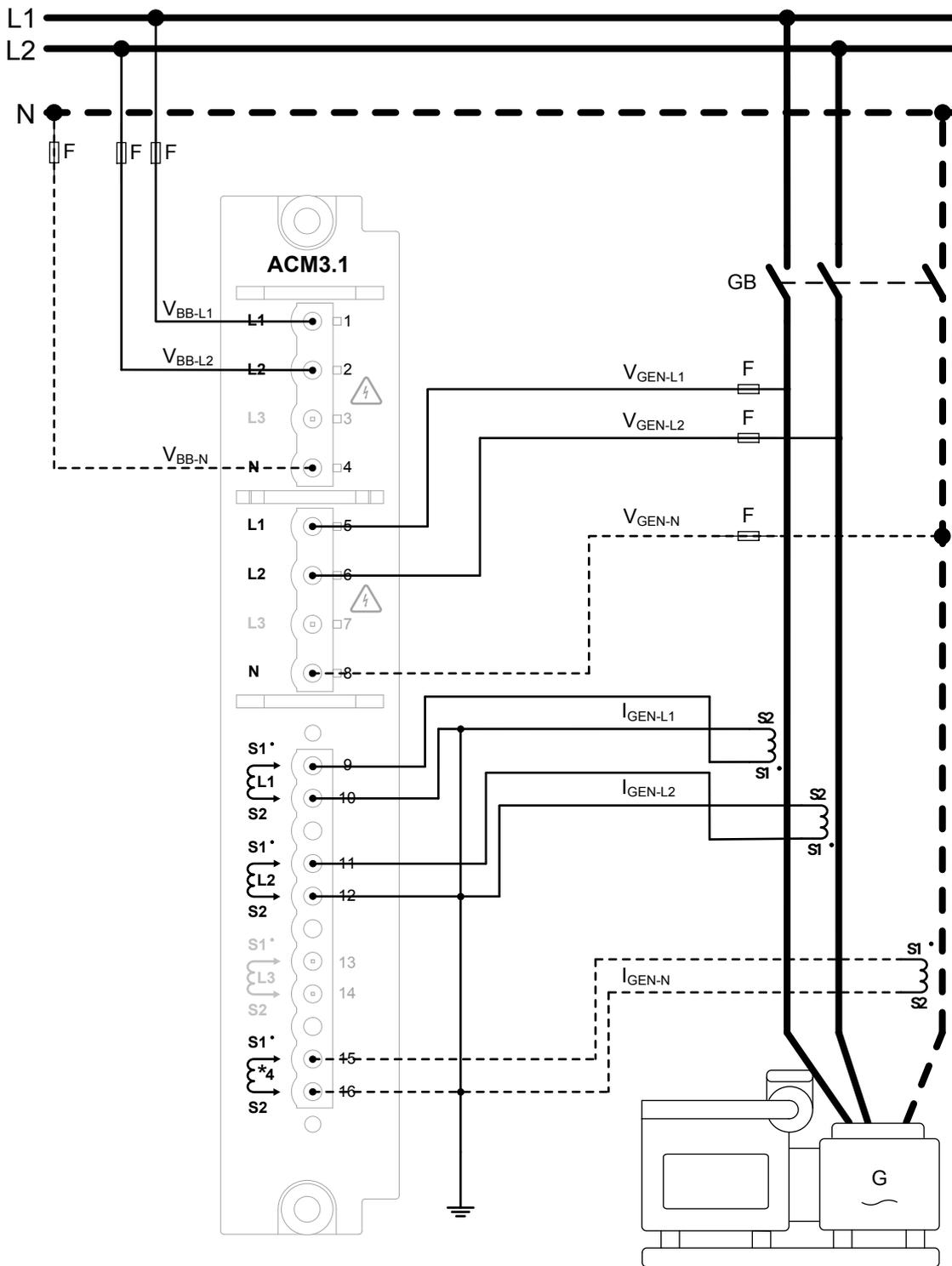
For split-phase, the waveforms are offset by a half-cycle (180 °) from the neutral wire. Split-phase is also called L1-N-L2, or single-phase in the USA.
