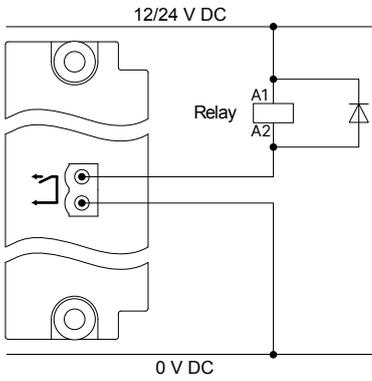
Install a freewheeling diode (
