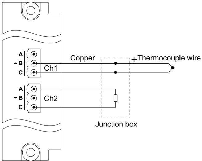
The cold junction compensation can be wired to any input on the controller that can measure a temperature sensor.
