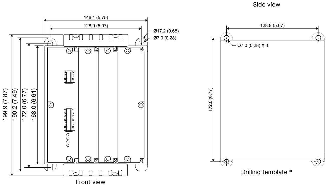
**NOTE** The drilling template drawings are meant as guidelines. Use the dimensions given to create your drilling template.
