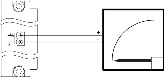
We recommend you use instruments from the DEIF DQ moving coil instrument series. See [www.deif.com](http://www.deif.com) for more information.
