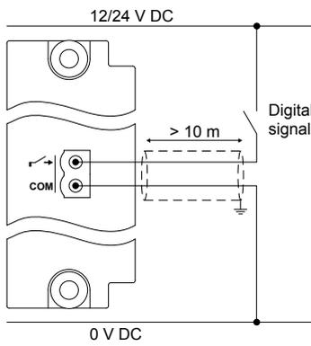
**Figure 4.83** Example: Closed contact for compliance with EN60255-26
