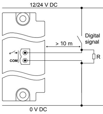
**Figure 4.81** Example: Twisted wire for compliance with EN60255-26
