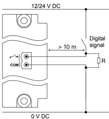
**Figure 4.61** Example: Twisted wire for compliance with EN60255-26
