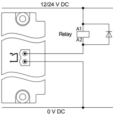
Install a freewheeling diode (
