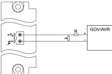
Typical value for the resistor is 2.5 k $\Omega$ , while the potentiometer is 5 k $\Omega$ .
