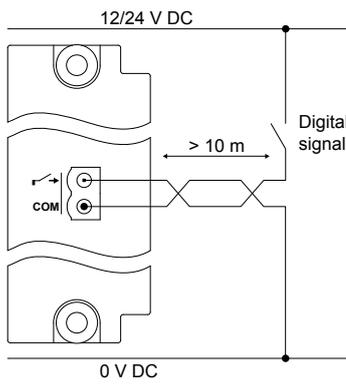
**Figure 4.82** Example: Shielded wire for compliance with EN60255-26
