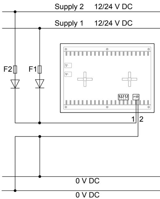
We recommend a 2 A time-delay fuse for 24 V DC and a 4 A time-delay fuse for 12 V DC for F1 and F2, and that the diodes are rated 50V or higher.
