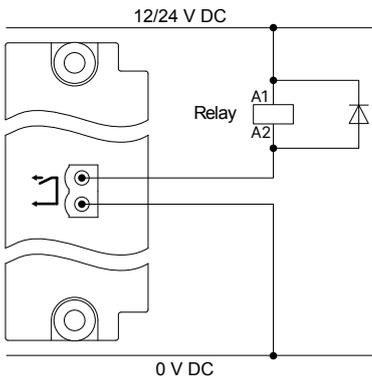
Install a freewheeling diode (
