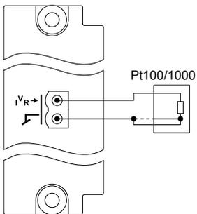
You do not have to connect the third wire (shown by the dashed line). If you want to connect the third wire, connect it to the common, as shown in the diagram.
