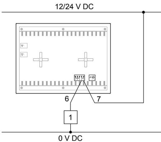
It is not possible to configure the relay state. The relay is in a **Normally open (NO)** and **De-energised** state.
