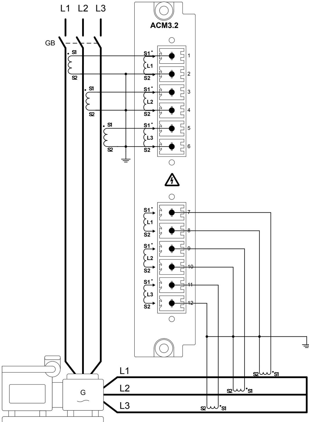
All the current transformers in the example diagram have a direction towards the protected object. Make sure that the current transformers are installed correctly according to the wiring diagrams for your site, and that the *Current reference dir.* parameters for the controller match the installed direction.
