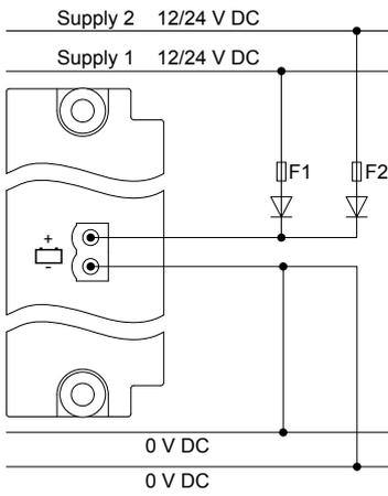
We recommend a 2 A time-delay fuse for 24 V DC and a 4 A time-delay fuse for 12 V DC for F1 and F2, and that the diodes are rated 50V or higher.
