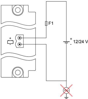
If the EIM power supply fails or is not connected, the PSM will supply power to the EIM.
