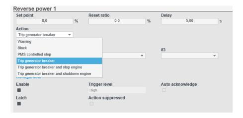
In order to select when the alarms are to be active, there is a configurable inhibit setting for every alarm. Inhibits are also different from PPM-2 to PPM 300 parameter. The inhibit functionality is only available via the PC utility software. For every alarm there is a drop-down window where it is possible to select which signals that have to be present in order to inhibit the alarm.
