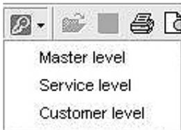
If the password level is not entered, it is not possible to enter the parameters.
