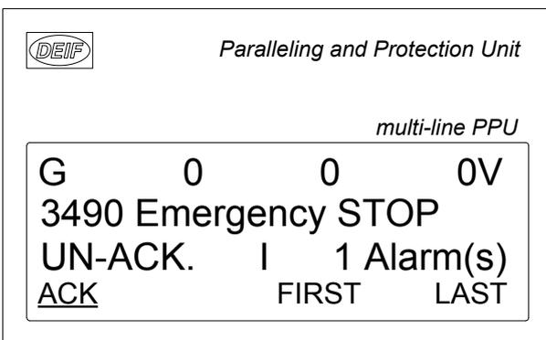
This display example indicates an unacknowledged alarm. The display can only show one alarm at a time. Therefore, all other alarms are hidden.
