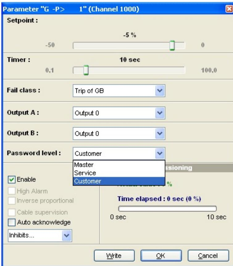
The password level can be found in the column "Level" in the parameter view.
