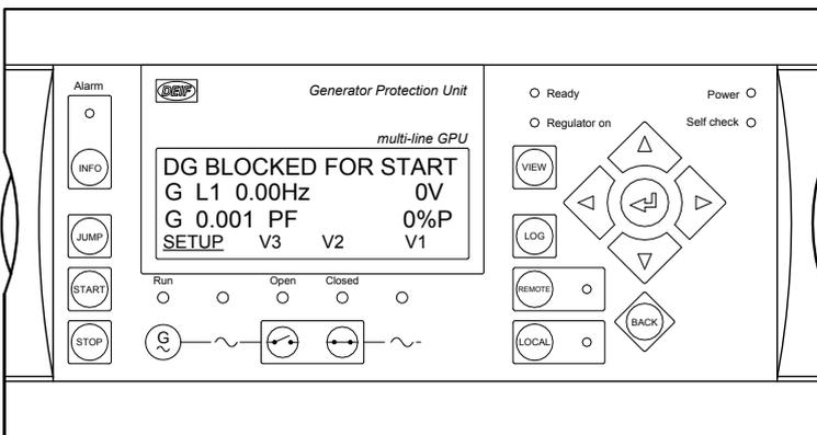
Place the cursor under **SETUP** and press the
