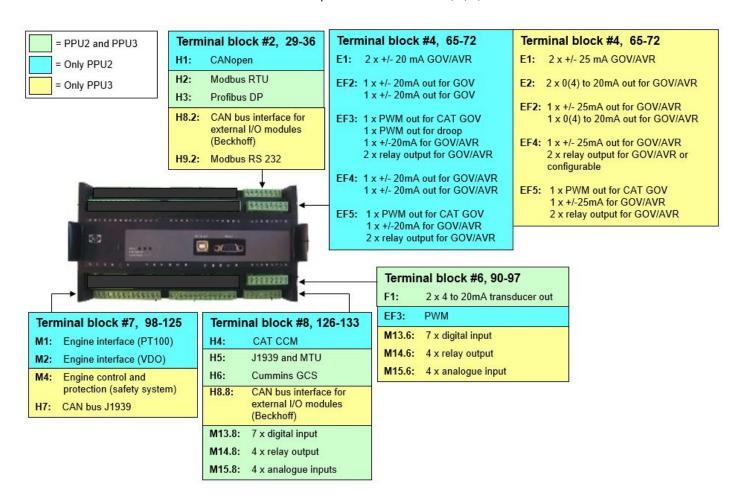
The table below provides an overview and description of the PPU-2 options and shows which options that can be converted to PPU-3. PPU-2 options B1 and C1 are implemented as standard software in PPU-3.
