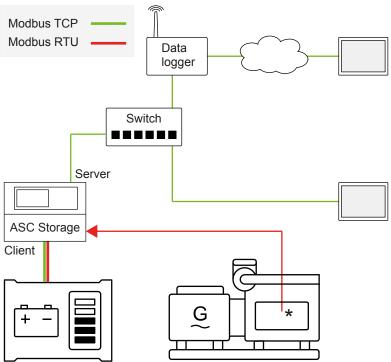
The ASC can communicate over Modbus as the client and/or server device. The ASC can communicate with the ESS using Modbus TCP and/or Modbus RTU. \* The ASC reads from power meters or genset controllers using Modbus RTU.
