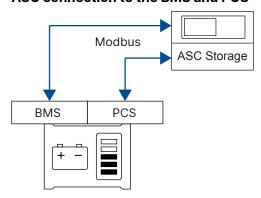
Select **DEIF Generic** in *ESS protocol* (parameter 7561) to control the PCS and select **DEIF Generic** in *BMS protocol* (parameter 7681) to control the BMS.
