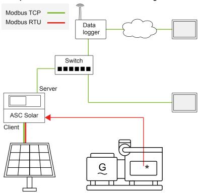
The ASC can communicate over Modbus as the client and/or server device. The ASC can communicate with the PV system using Modbus TCP or Modbus RTU. The ASC reads from power meters or genset controllers using Modbus RTU.
