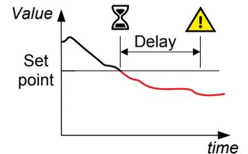
Busbar > Voltage protections > Under-voltage > BB U< [1 to 4]
