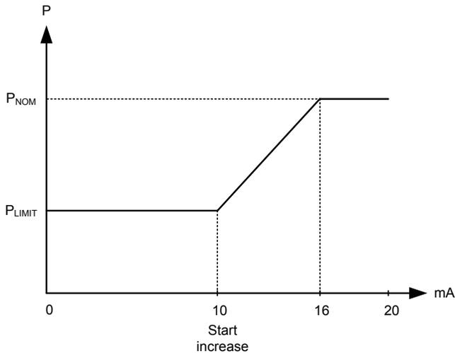
The inverter is derated when the control value is lower than the set point. In the example above, the control value is a mA signal.
