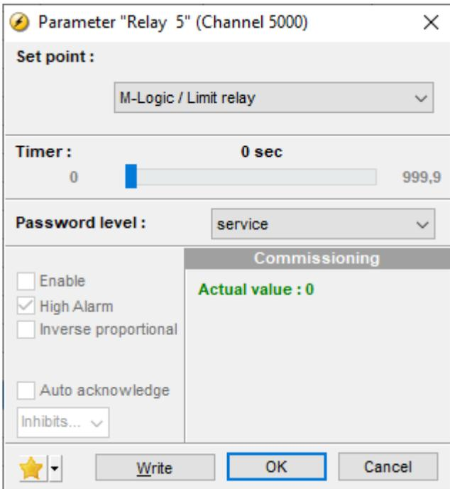
**NOTE** If the relay function is not *M-Logic / Limit relay*, the controller activates an alarm every time that the PV system is running.
