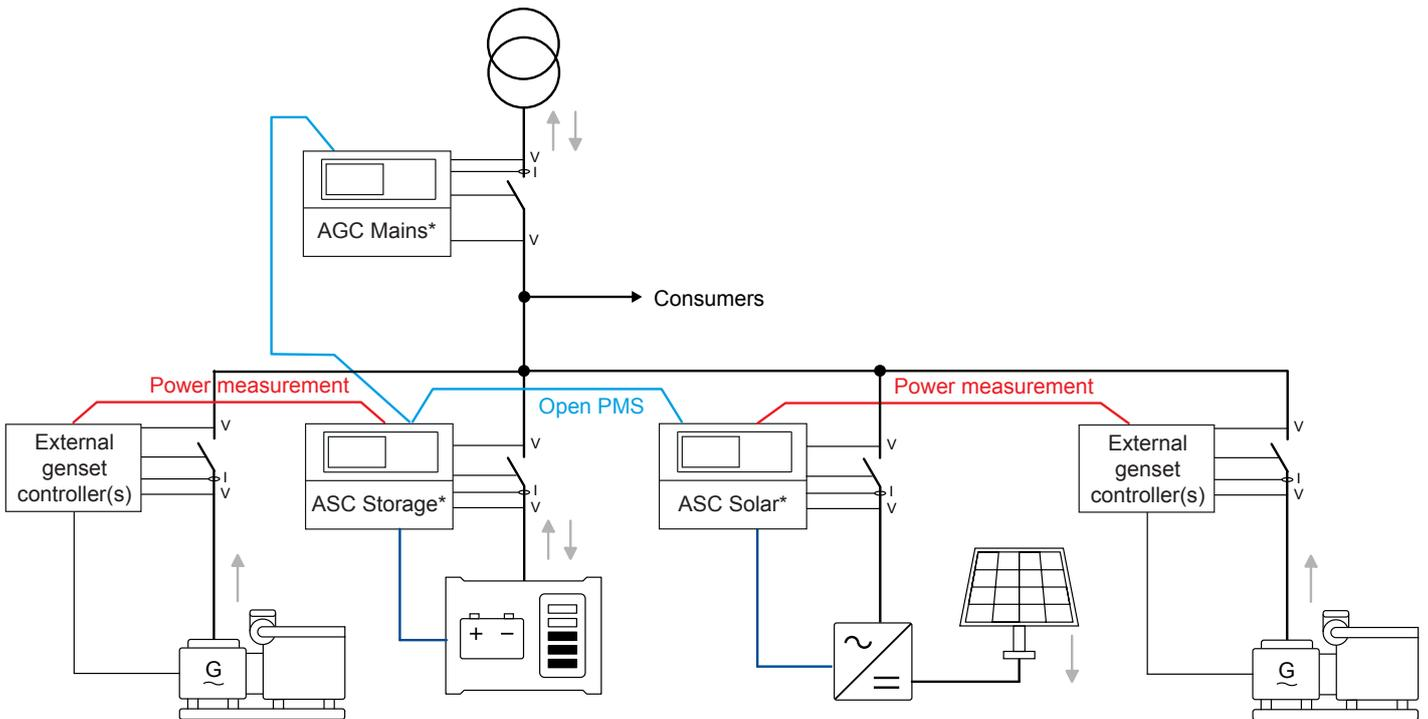
**NOTE** \* You can use multiple controllers in the application. Power measurements can be connected to the closest ASC controller.
