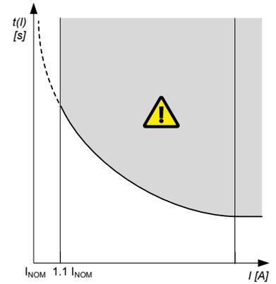
AC configuration and protections > Current protections > Earth fault inverse time over-current
