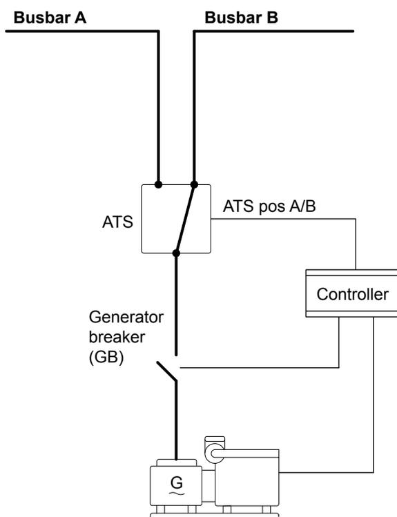
In the ASC in M-Logic, you can program whether the genset is connected to the PV side (enabled) or connected to the side without the PV (disabled):
