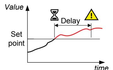
Busbar > Voltage protections > Over-voltage > BB U> [1 to 3]
