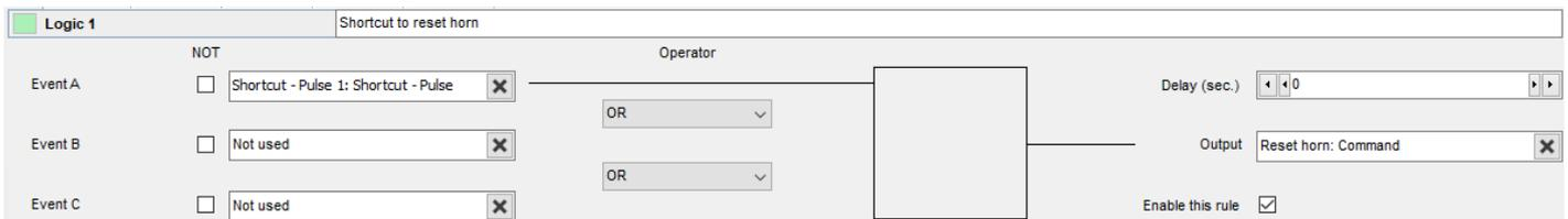
The screenshot shows the configuration for 'Logic 1' titled 'Shortcut to reset horn'. It features three event inputs (Event A, B, C) under a 'NOT' section. Event A is selected with 'Shortcut - Pulse 1: Shortcut - Pulse'. The 'Operator' section has two 'OR' dropdown menus. The 'Output' is set to 'Reset horn: Command'. The 'Delay (sec.)' is 0, and 'Enable this rule' is checked.
