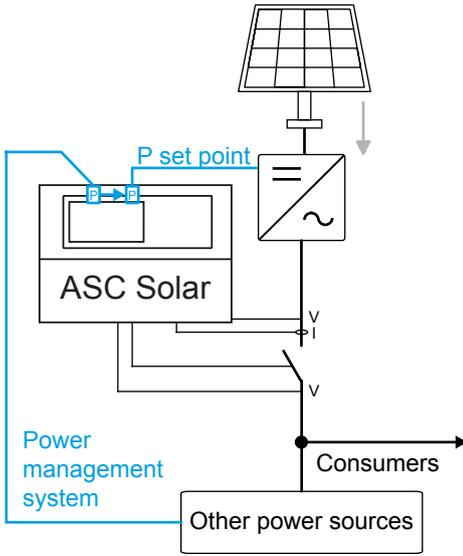
By default, *Closed loop* (parameter 2631) is **Not enabled**. The ASC sends the power set point from the power management system to the PV system.
