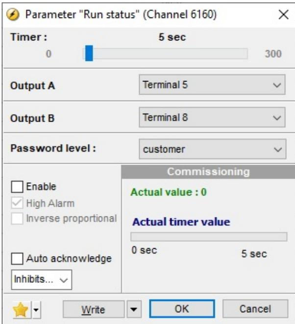
Select the relays in output A and/or output B, and enable the function. If the timer setting is 0 s, the function is activated as soon as the controller gets running feedback from the PV system.
