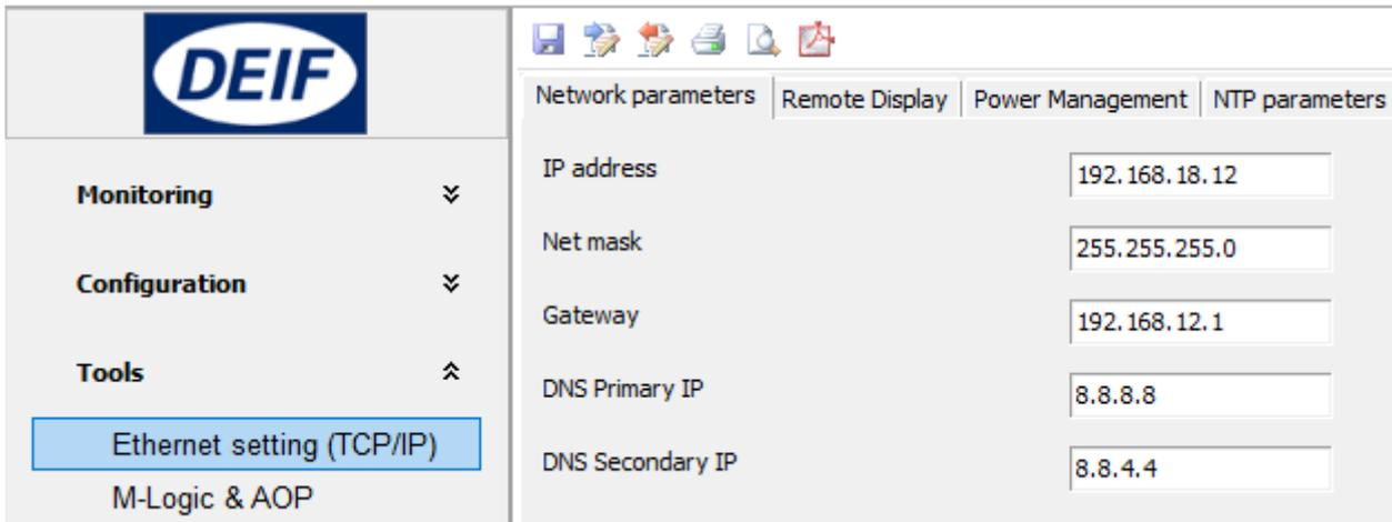
When the controller network parameters have been changed, press the *Write to device*
