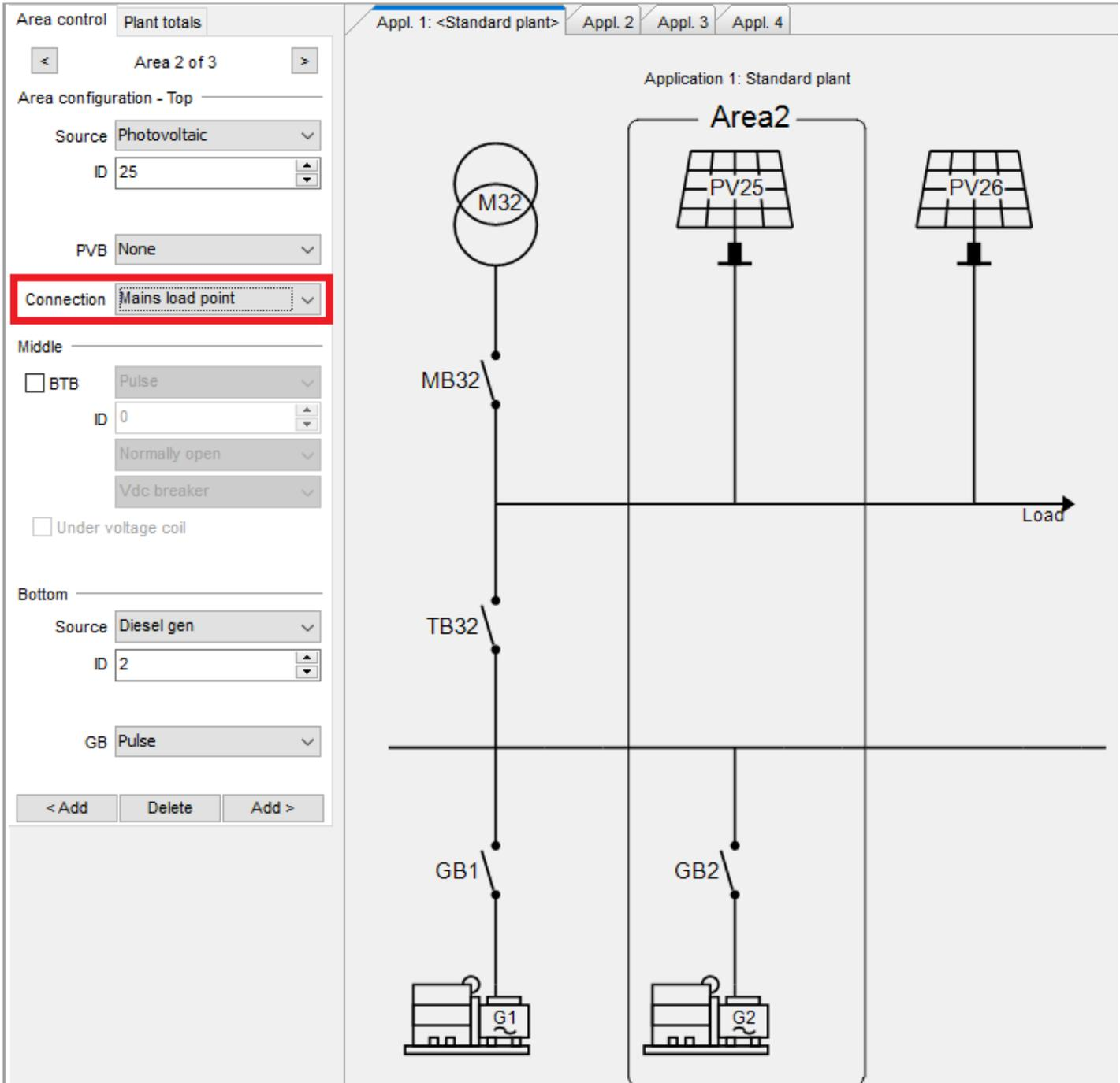
**NOTE** For ASC 150 Solar, PV can only be connected to the load point if the ASC does not control the PVB.
