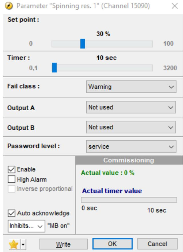
**NOTE** Select *Auto acknowledge* to automatically deactivate the output when the spinning reserve required is available again. Select *Enable* to enable the alarm.
