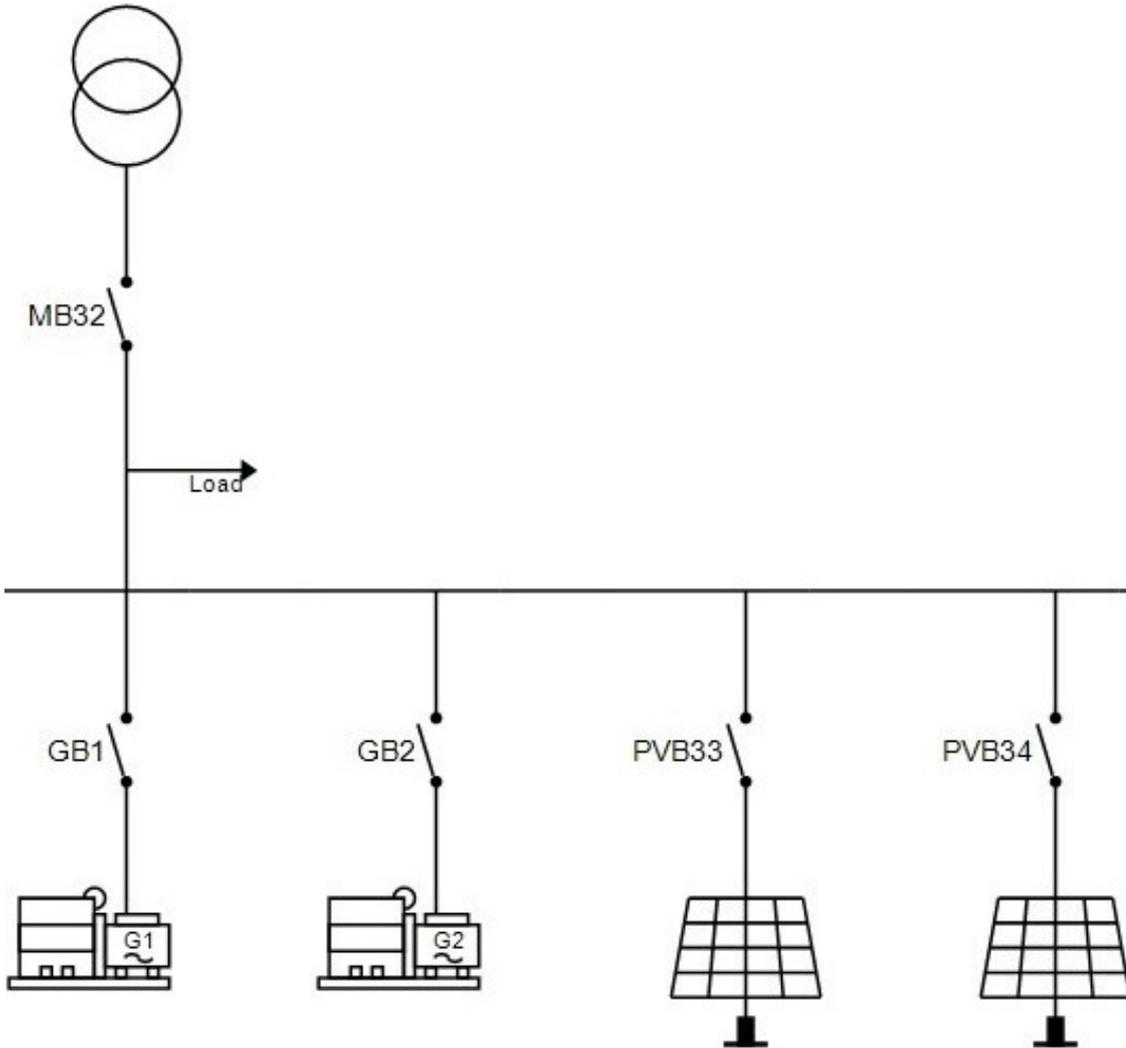
The ASC can control a PV breaker. For PV, this can be useful if there is a breaker in front of the string of inverters. The breaker can close when the busbar is live and Hz/voltage is normal. If the busbar is outside its limits, the ASC can open the PV breaker but not close it.
