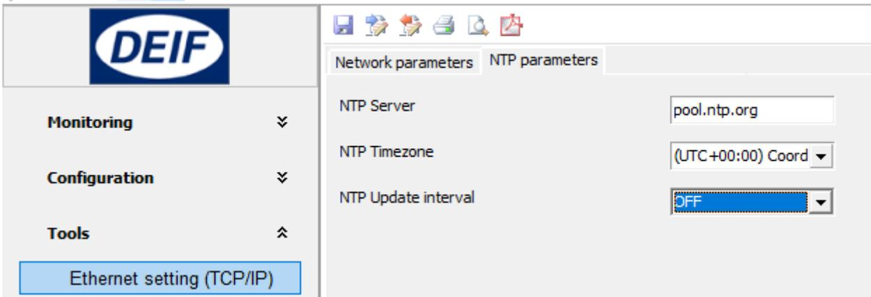
You can select an NTP server, a time zone and an update interval. Write the changes to the controller to activate the NTP function.
