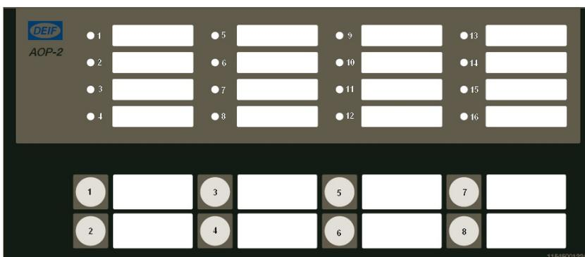
The configurable LEDs are named 1 to 16, and the buttons are named 1 to 8.
