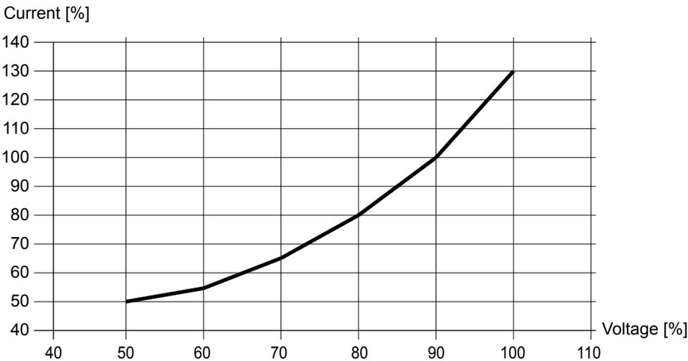
When the operating values are above the curve, the breaker is tripped. The PVB also trips when the PV voltage is below 50 % of rated, and the current is above 50 % of rated.
