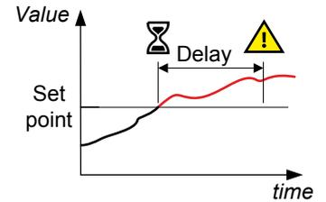
AC configuration and protections > Frequency protections > Over-frequency > PV f> [1 to 3]
