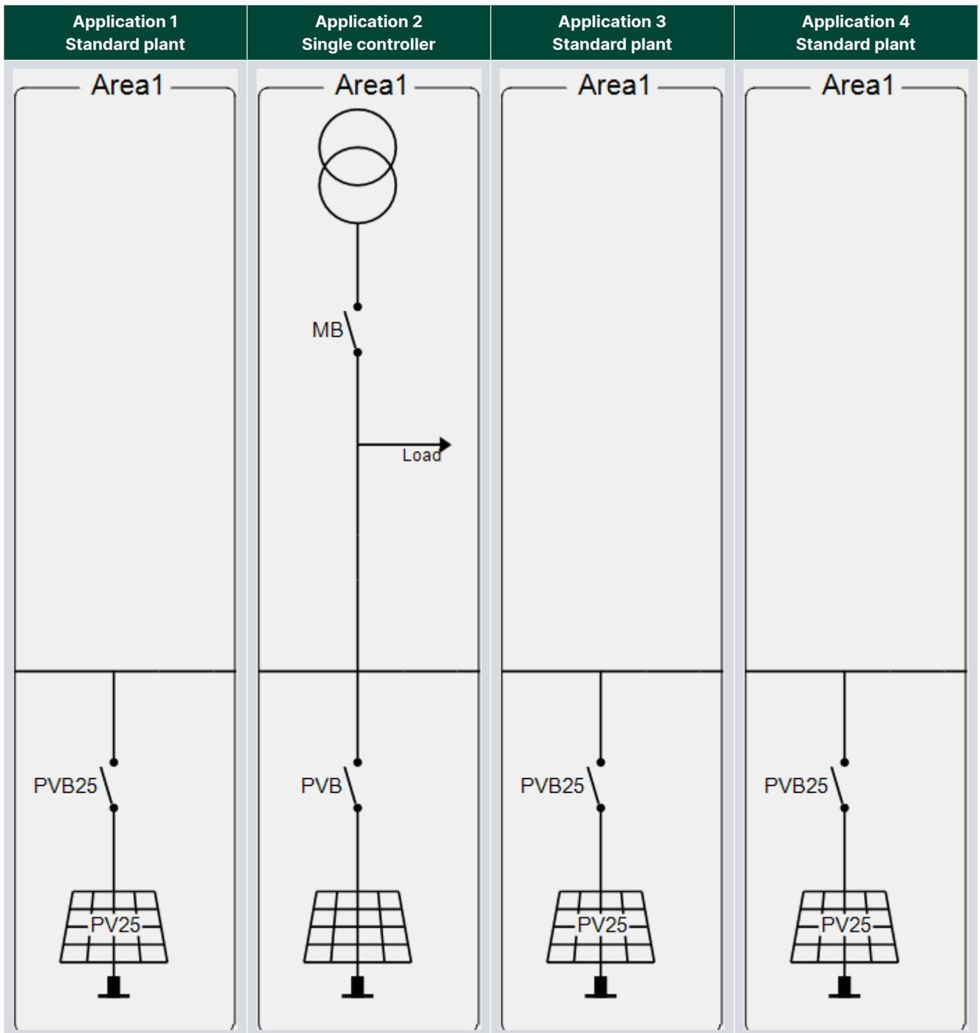
Select *Application configuration* in the left menu. The controller comes with four pre-configured standard applications. Standard applications 1, 3 and 4 are identical.
