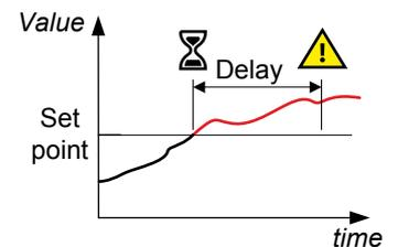
**AC configuration and protections > Current protections > Over-current > I> [1 to 4]**
