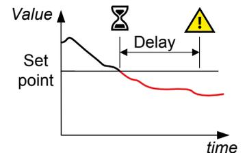
AC configuration and protections > Frequency protections > Under-frequency > PV f< [1 to 3]
