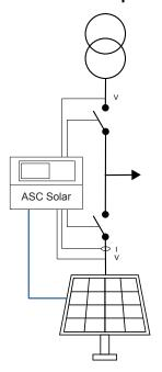
**Fixed power**: When given a signal, the controller starts, synchronises, and connects the PV. After the breaker closes, the controller ramps up the load to the set point level. When the stop command is given, the PV breaker is de-loaded, opened and the PV is stopped.
