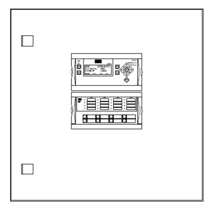
Typically, this switchboard is used where the PV is installed with existing gensets, hence it can be fully equipped with all necessary equipment for supporting this application. This includes measurement transducers, power supply and a summation CT.
