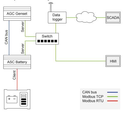
NOTE You can use an RTU to TCP/IP converter for the communication between the ASC and the battery. See the **ASC-4**Commissioning guidelines for more information.
