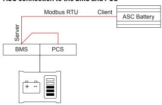
Select **DEIF Generic** in *ESS protocol* (parameter 7561) to control the PCS and select **DEIF Generic** in *BMS protocol* (parameter 7681) to control the BMS.
