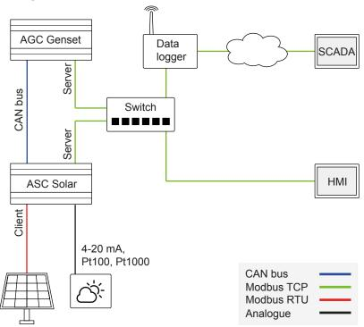
**NOTE** The ASC can get analogue weather data and/or use a Modbus RTU interface.
