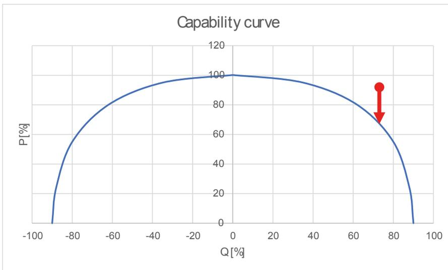
**NOTE** If the curve is set up like below, P derate cannot be used since the derate does not improve the situation. Only Q derate can bring the set point inside the limitations.
