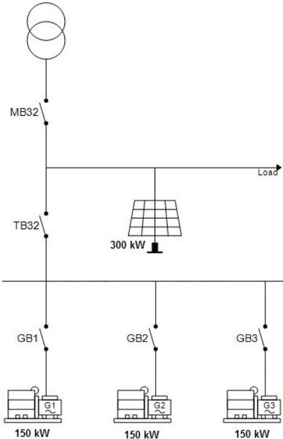
Alternatively, use the mains controller tie breaker to separate the gensets from the PV plant.
