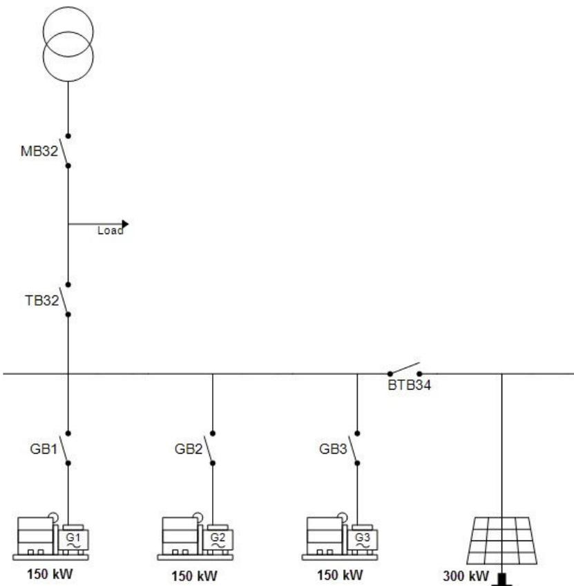
Keep BTB34 open unless grid-tied or if MB32 is open, then close BTB34 only if more than one (two or three) gensets are connected.
