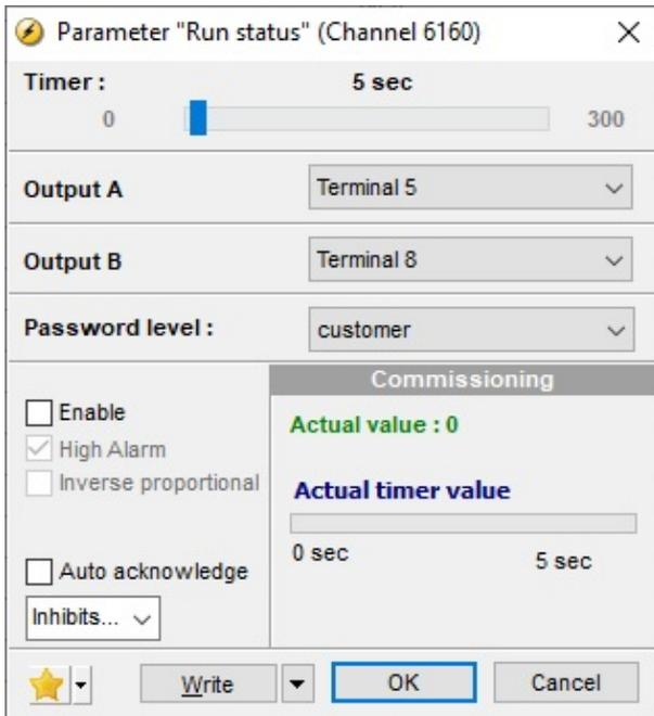
Select the correct relay numbers in output A and output B and enable the function. Change the relay function to limit in the I/O menu. Then the relay activates, but no alarm will appear.
