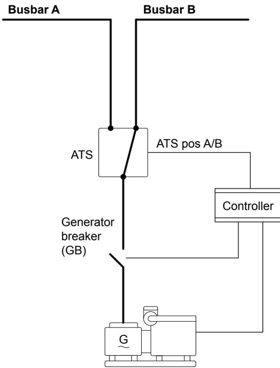
This M-Logic uses a digital input to enable and disable a genset. Set it up so that the genset is enabled when it is connected to the busbar with the PV. For the diagram above, the output from the ATS is connected to digital input 23.
