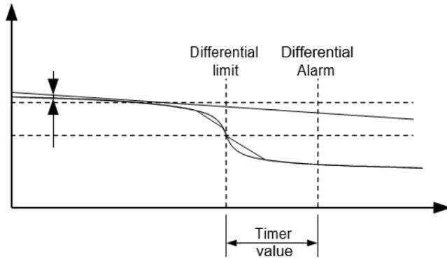
Three different differential measurements between two analogue input values can be configured.
