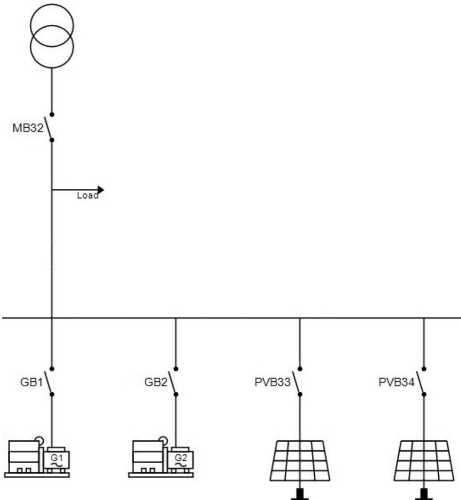
The ASC can control a PV breaker. For PV, this can be useful if there is a breaker in front of the string of inverters. The breaker can close when the busbar is live and Hz/voltage is normal. If the busbar is outside its limits, the ASC can open the PV breaker but not close it.
