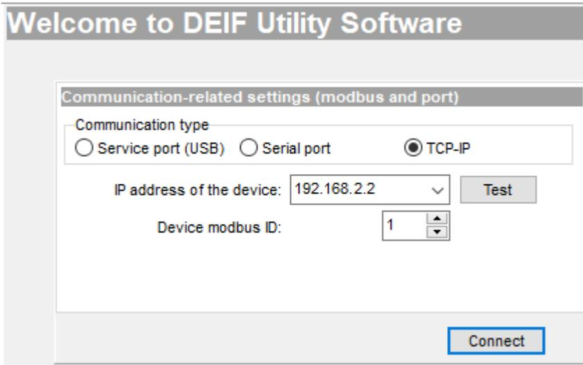
4. You can use the *Test* button to check if the connection is successful.
