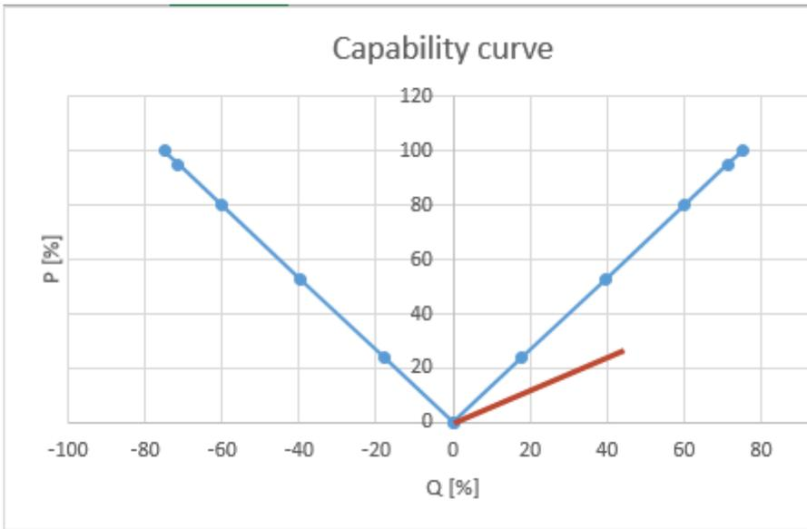
It can be seen that the current running condition is out of the capabilities of the inverters and the set point will (typically) be ignored (depends on inverter design).
