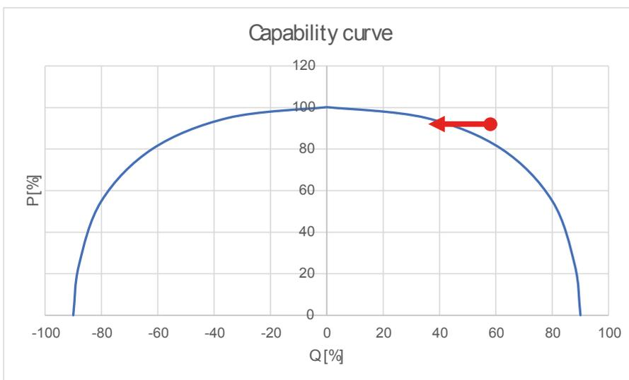
If the inverter has some limitations that it can only operate within for example +/- 0.8PF, it must be adjusted in the curve. In that case, the ASC will behave according to this, and the set points in the ASC system will take the limitations into account.
