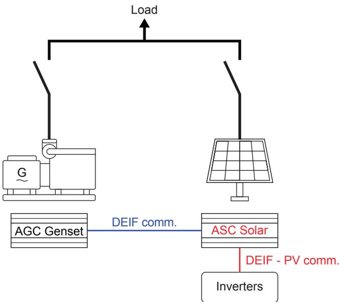
The blue line on the diagram shows the CAN bus power management communication between the ASC Solar and the AGC.
