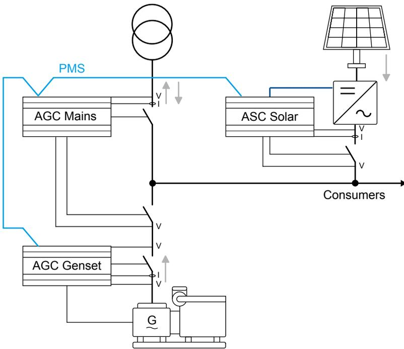
In a power management combination application, the ASC can have the following modes of operation:
