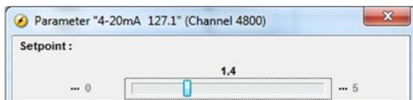
In the example shown above, the value can be adjusted with one decimal. If the parameters were not refreshed, it would still only be possible to adjust the set point without decimals.
