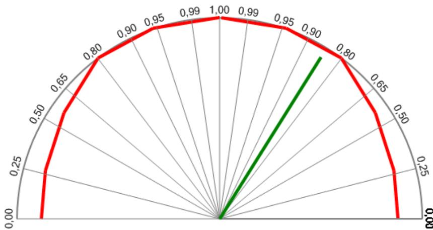
The curve is described by 6 points on the capacitive side and 6 points on the inductive side using these settings:
