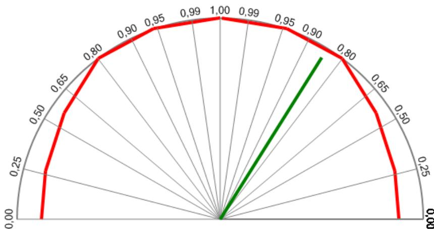
The kvar set points depend on the plant mode. In island operation, the PVs and the gensets share equally and therefore run at the same cos phi. In mains parallel, the cos phi set point follows the set point as configured in the ASC or it can receive set points from the mains controller.
