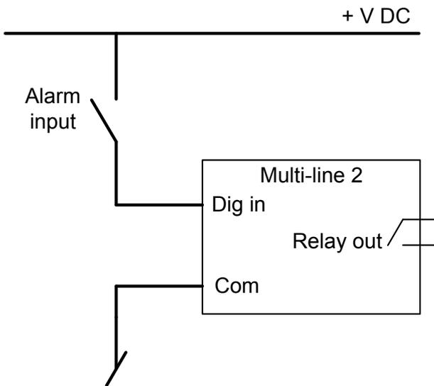
**NOTE** You can use *Output A* and *Output B* to select a relay output for the digital input alarm.
