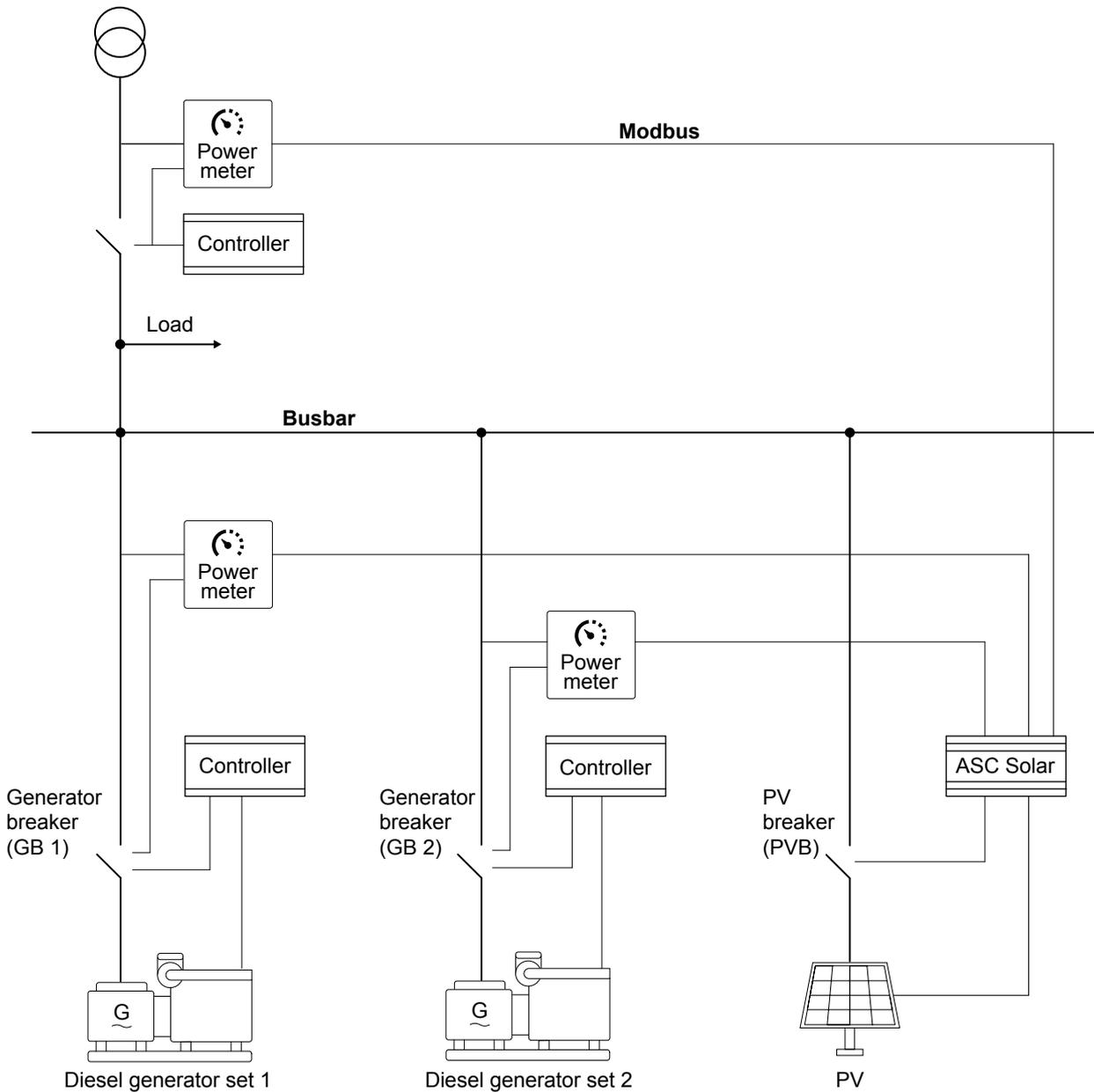
Alternatively, you can hardwire feedback from the breakers (GBs and MB).
