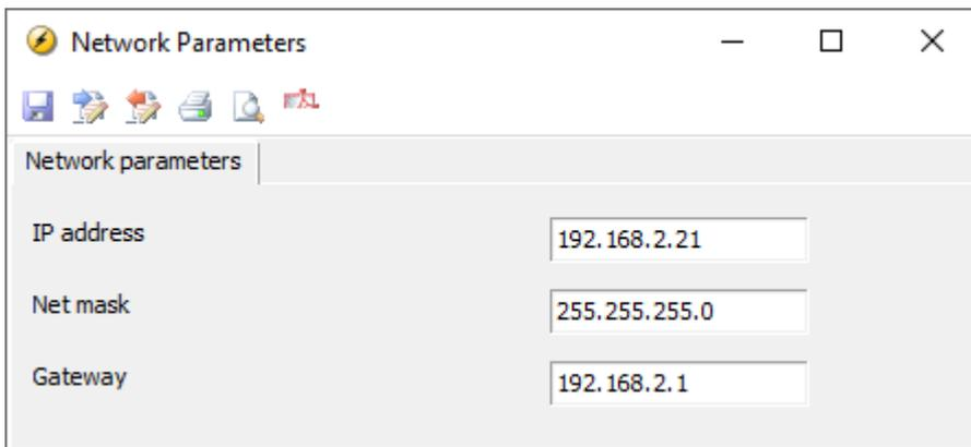
When the controller network parameters have been changed, select the *Write to device*
