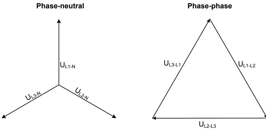
As indicated in the vector diagram, there is a difference in voltage values at an error situation for the phase-neutral voltage and the phase-phase voltage.
