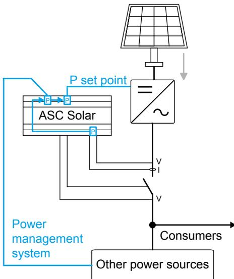
To use the closed loop function, select **Enable** for *Closed loop* (parameter 2631).
