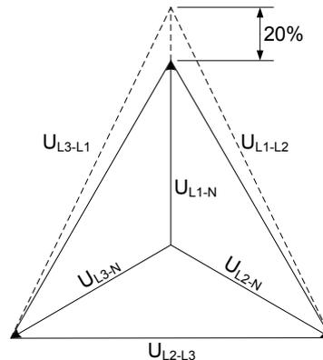
**NOTE** Phase-neutral or phase-phase: both the generator protections and the busbar/mains protections use the selected voltage.
