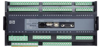
In a power/energy management system (PMS), the controller is designed for seamless integration of PV power with other power sources. Multiple ASC-4 Solar controllers can be used in each PMS. The PMS makes sure that spinning reserve requirements are met, and responds quickly to load and weather changes. To save fuel, the PMS maximises PV penetration, while making sure that the gensets meet their minimum load requirements.
