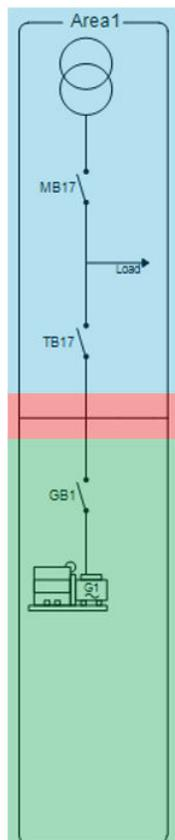
The single-line diagram of the plant is shown on the Application configuration canvas, to the right of the **Area control** window. The single-line diagram has three horizontal sections:
