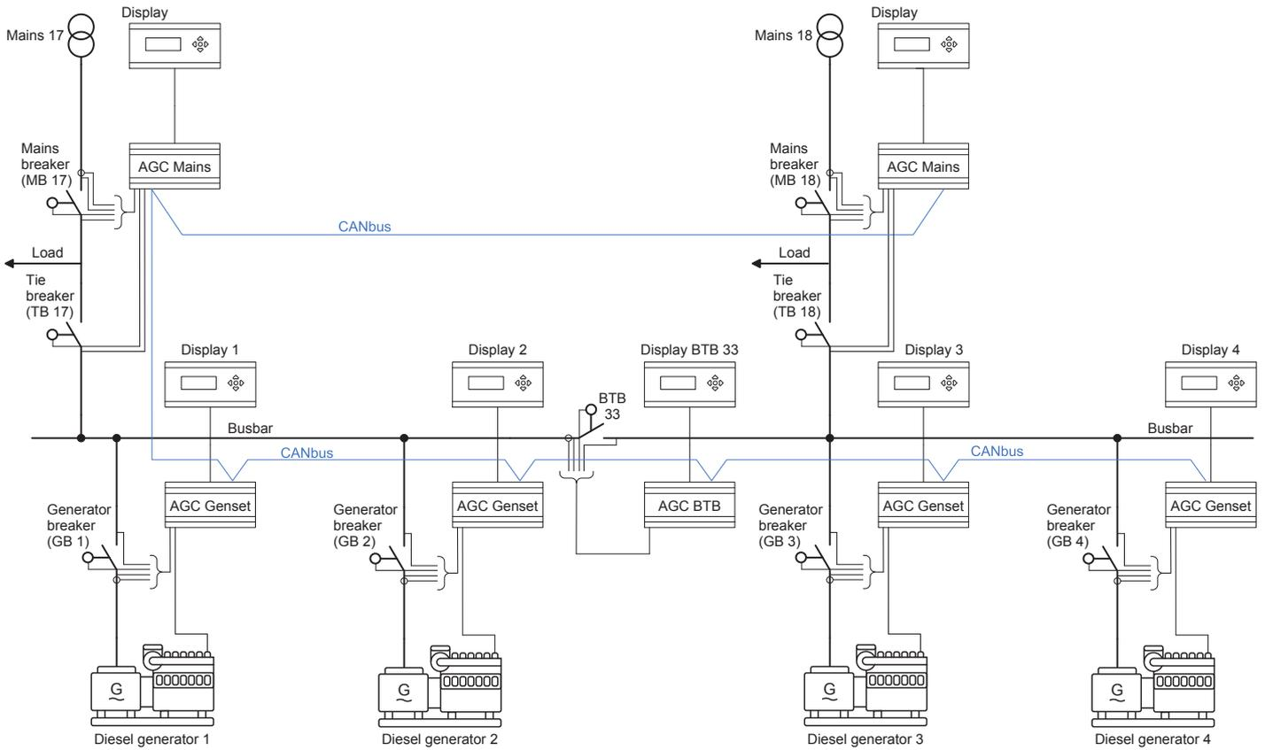
**NOTE** The diagram shows four generators, but the system supports up to 32 generators. For more information, see **Option G5**.
