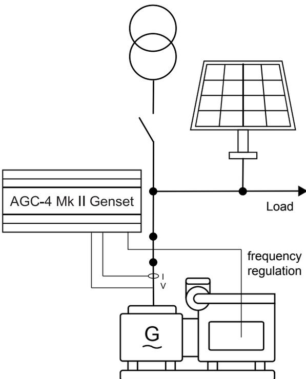
DFR uses the standard genset controller's connections. DFR uses the measurements from the voltage and current terminals to calculate the genset power. DFR uses governor regulation to regulate the busbar frequency.
