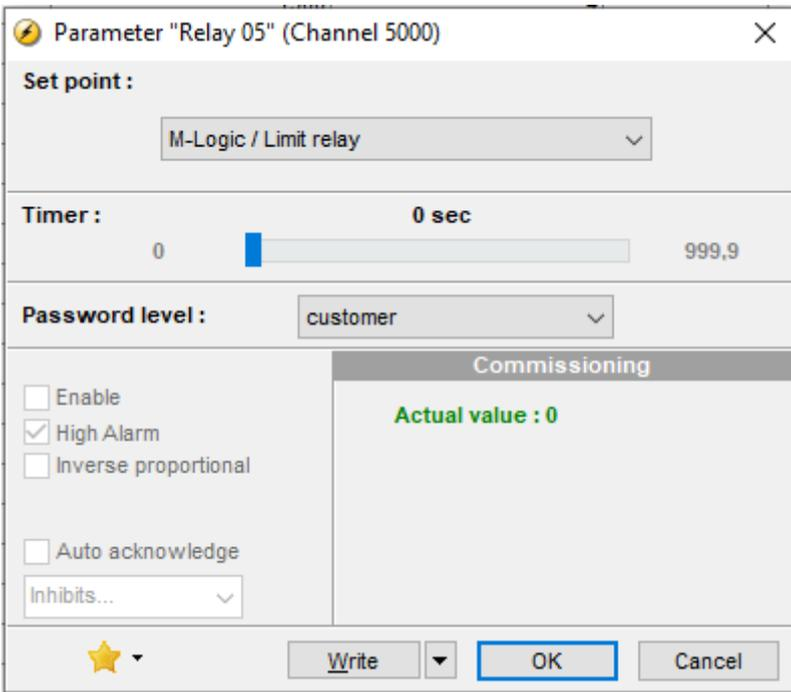
Alternatively, you can configure the relay in the USW under *I/O Setup*:
