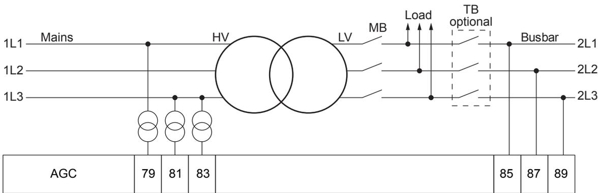
**NOTE** The connection shown in the picture should always be used when a controller is used for a mains breaker.
