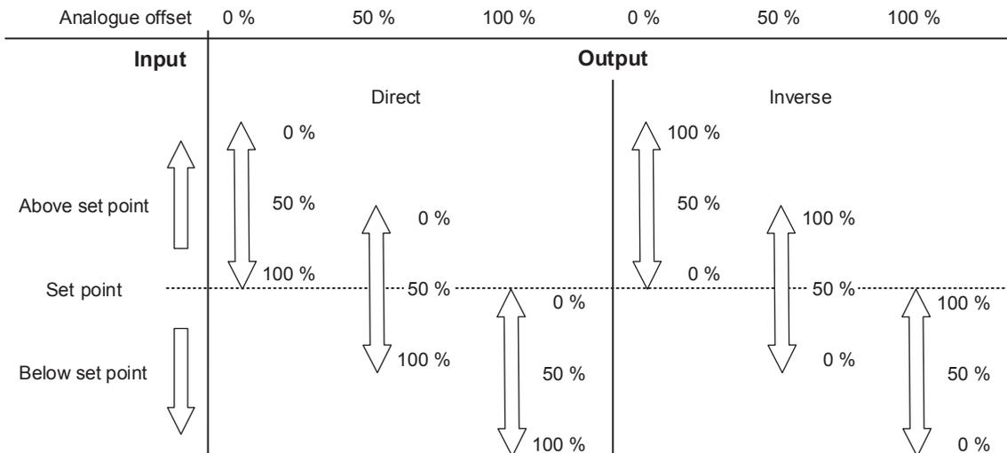
An offset of 100 % is commonly used with inverse output, like in the previous cooling example. See also **Example of inverse output with 0 % offset**.
