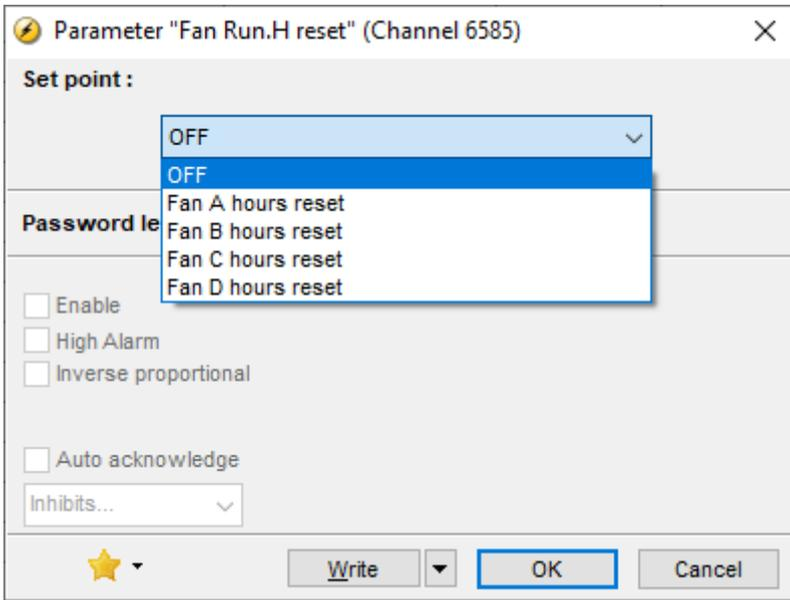
**NOTE** Only reset is possible. It is not possible to add an offset to the run hour counter.
