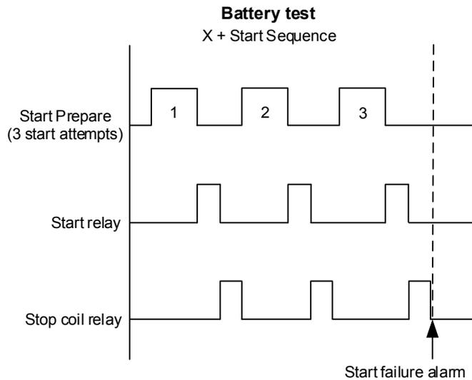
A battery test configured as *X + Start sequence*, as shown in the above example, will use: *Start prepare* timer, *Start on time* and *Start off time*. In this example, the genset will crank three times with *Start prepare* and *Start off time* delay in between each crank. When the test has finished, a start failure alarm will be present.
