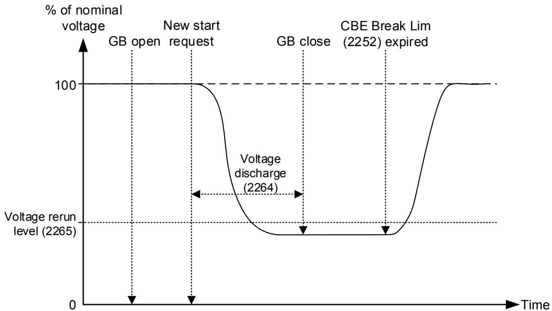
In the diagram above, the excitation is ON during cooldown. When a new start request is made, the excitation is shut off. When the excitation is shut off, the voltage discharge timer starts.
