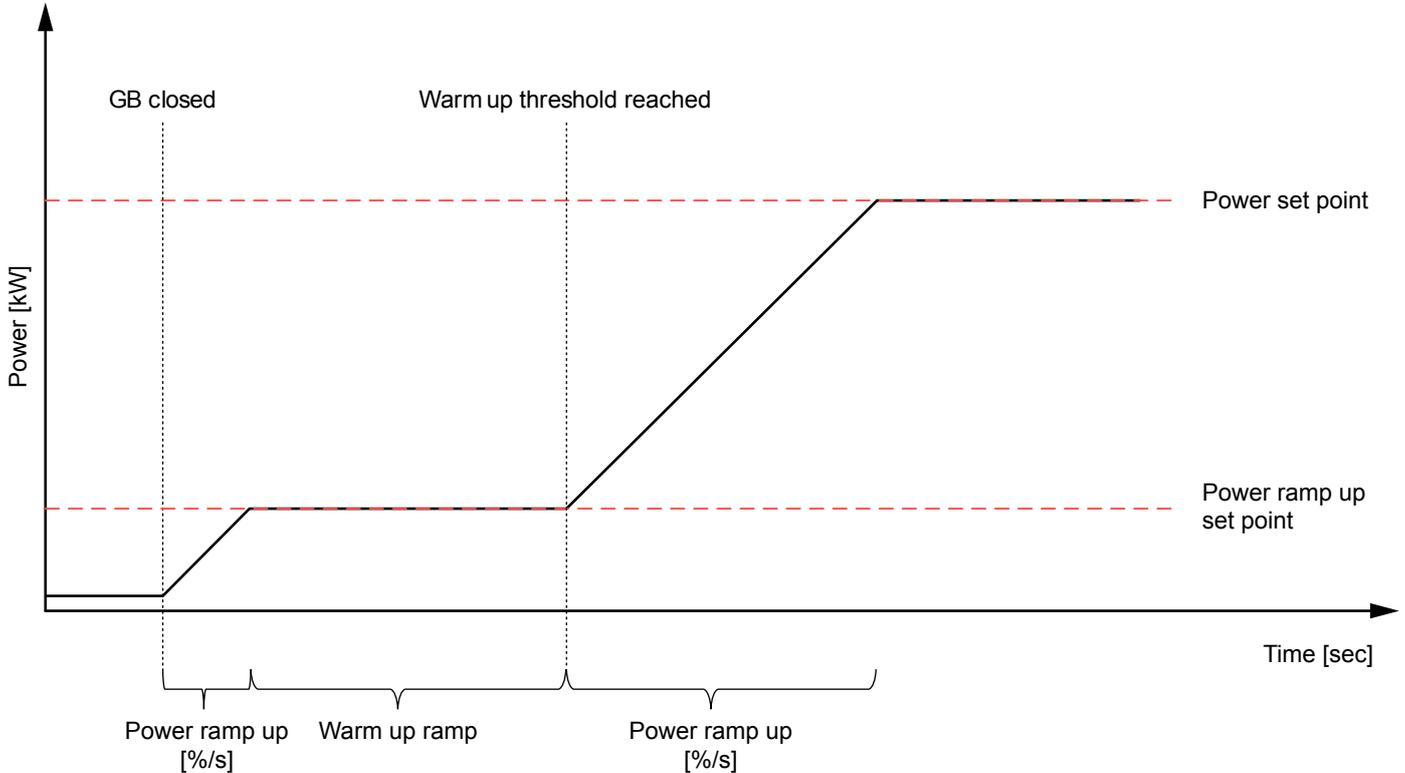
The warm up ramp activation is enabled and the input is configured via *Warm up type* (parameter 2961). The activation of the warm up ramp input limits the available power of the genset to the percentage level configured in *Power ramp up* (parameter 2612).
