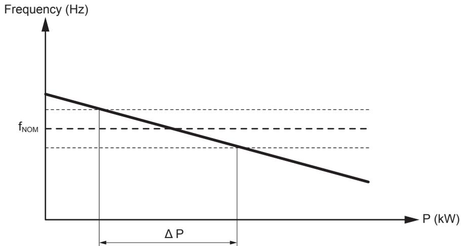
**NOTE** This can be used if the generator must operate as a peak load machine.
