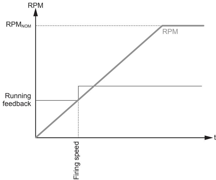
The diagram illustrates how the digital running feedback (terminal 117) is activated when the engine has reached its firing speed.
