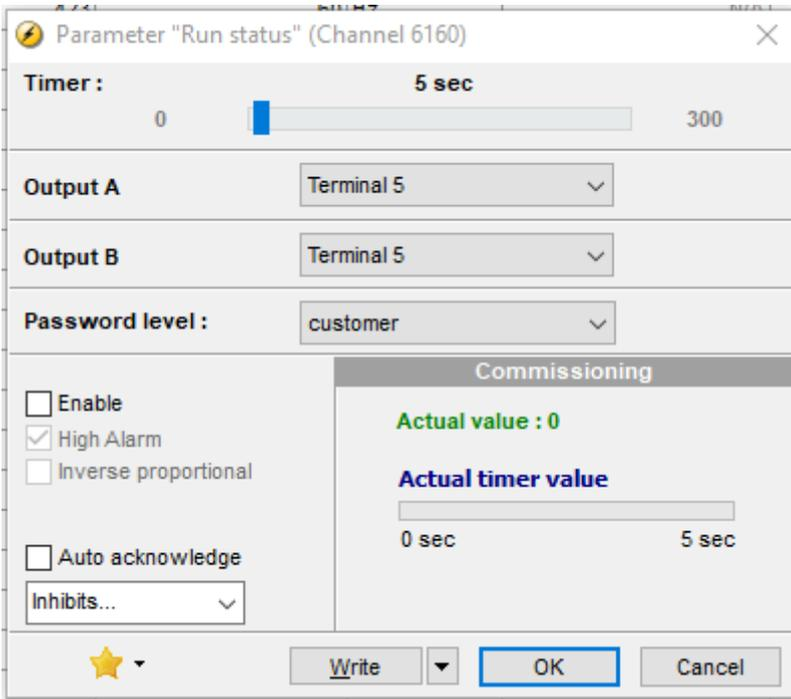
Select the correct relay number in output A and output B and enable the function. Change the relay function to limit in the I/O menu. Then the relay will activate, but no alarm will appear. Note that to avoid an alarm, both output A and output B need to be configured to a relay.
