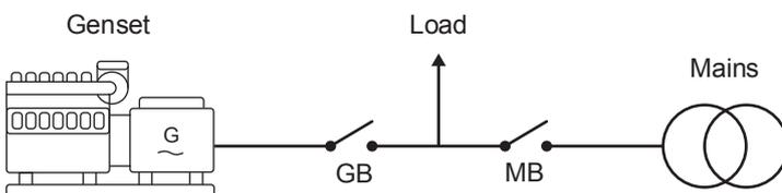
When the AGC is mounted correctly, the gensets voltage measurements are mounted between the Generator Breaker (GB) and the genset. The other voltage measurements are mounted between the Mains Breaker (MB) and the incoming grid connection. On the different controllers the voltage terminals is shown below:
