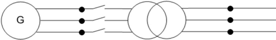
The phase angle compensation would not be an issue if there was no phase angle shift across the step-up transformer, but in many cases there is. In Europe, the phase angle shift is described using the vector group description. Instead of vector group, this could also be called clock notation or phase shift.
