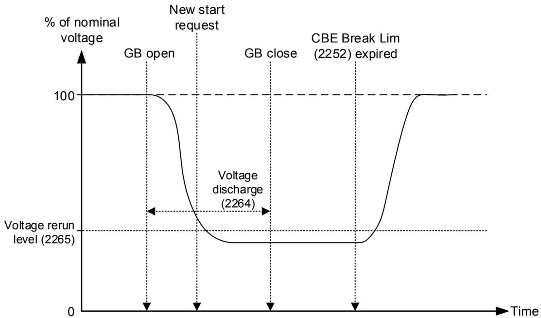
In the diagram above, the excitation is shut off as soon as the breaker is opened. Soon after the breaker is opened, a new start request appears. The controller delays closing the GB until the voltage discharge timer has expired.
