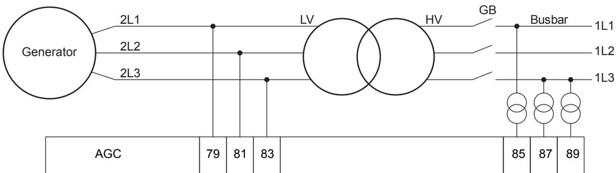
**NOTE** The connection shown in the diagram should always be used when an AGC is used for a genset.
