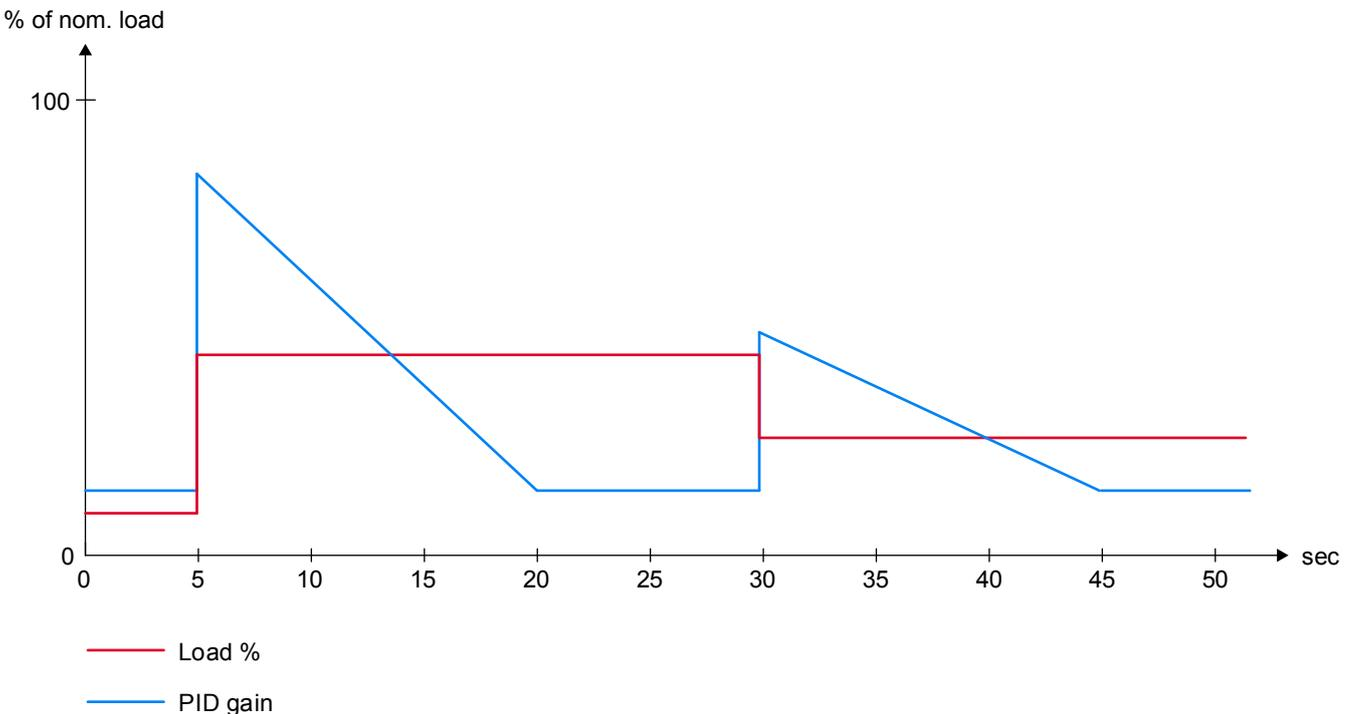
The diagram above shows the reaction of the gain, based on two load changes.
