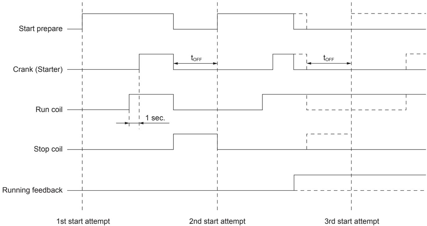
**NOTE** The run coil can be activated from 1 to 600 sec. before the crank (starter) is activated. In the example above, the timer is set to 1 sec. (menu 6150).
