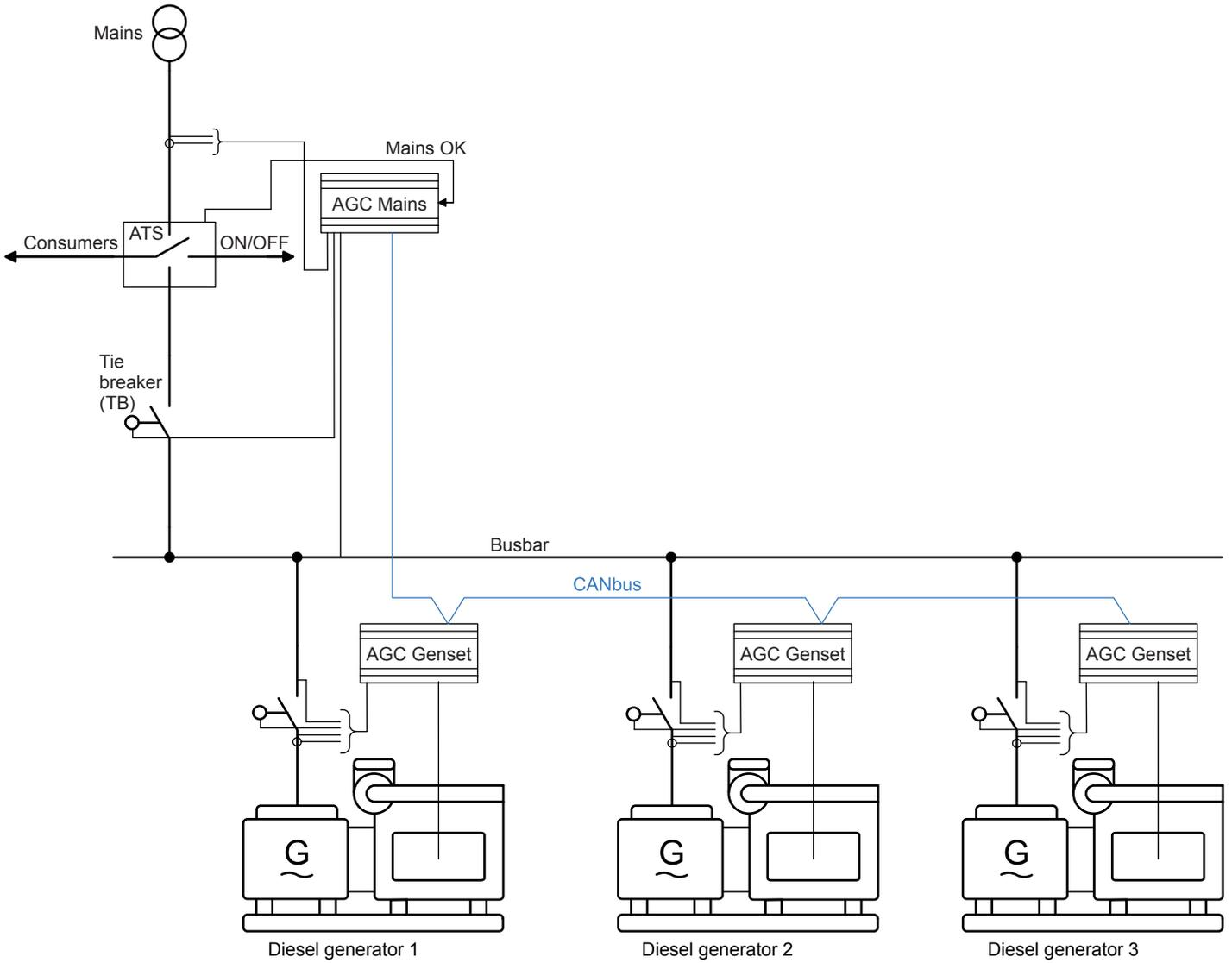
**NOTE** The simple ATS function (a *Mains OK* signal is sent to an AGC digital input) is shown here. See **Option G5 Power management** for a description of the more advanced ATS function.
