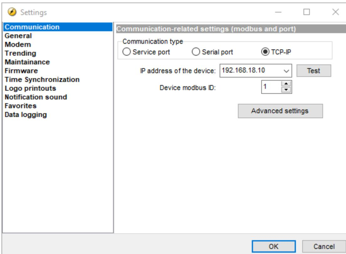
4. You can use the *Test* button to check if the connection is successful.
