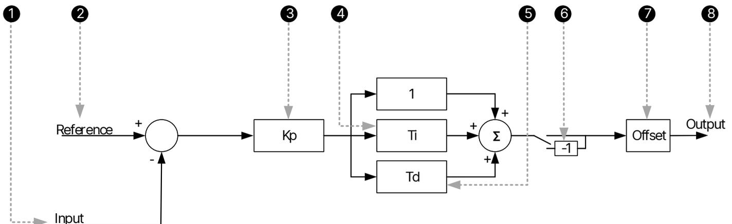
1. **Input:** This is the analogue input that measures the process that the controller is trying to regulate. See *Input* later in this document.
