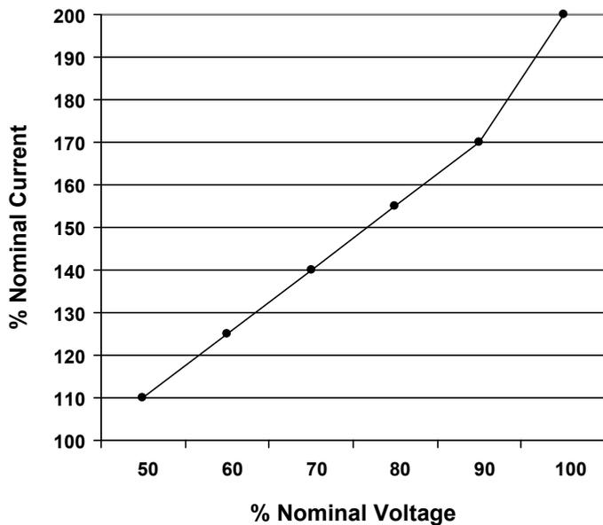
**NOTE** The voltage values for the six points on the curve are fixed. The current values can be adjusted in the range 50 to 200 %. Voltage and current % values refer to the nominal settings. The timer value can be adjusted in the range 0.1 to 60.0 seconds.
