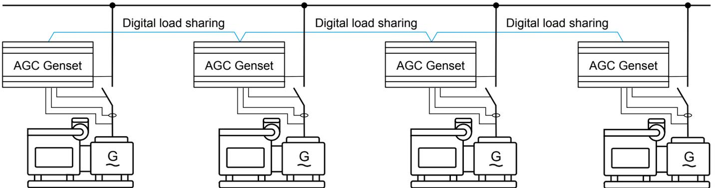
CANshare (digital load sharing) makes it possible for generators to load share using CAN bus, with simple installation and setup. CANshare load sharing is equal (as a percentage of each generator's nominal power). CANshare ensures that both active power (P) and reactive power (Q) are shared.
