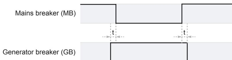
When the generator breaker is closed, the mains breaker is opened automatically before the timer runs out ( $t$ ). Similarly, when the mains breaker is closed, the generator breaker is opened before the timer runs out ( $t$ ). The timer is configurable (0.10 to 99.90 seconds).
