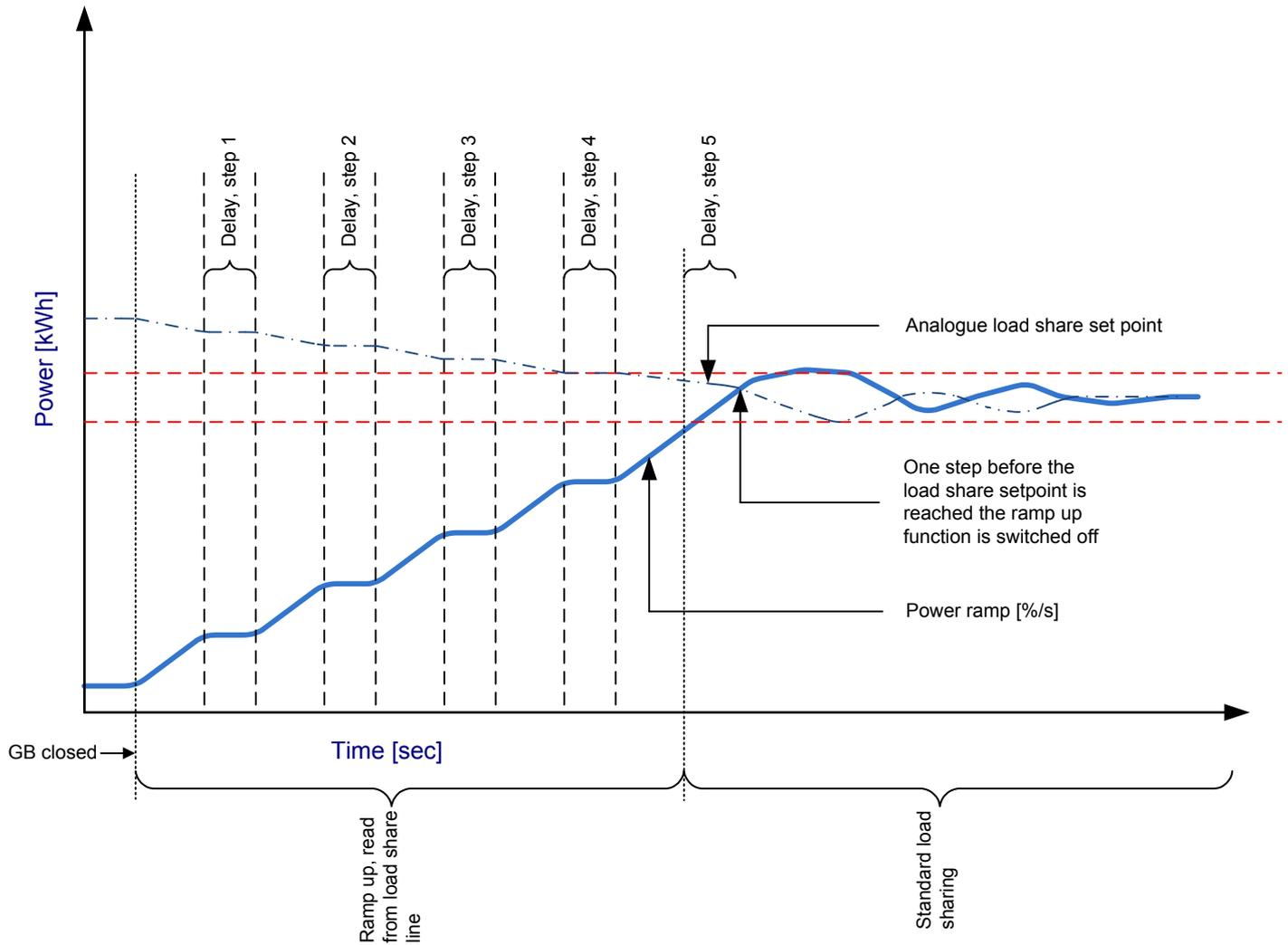
The genset controller includes a load ramp up function. If enabled, this also controls the load ramp up for analogue load sharing.
