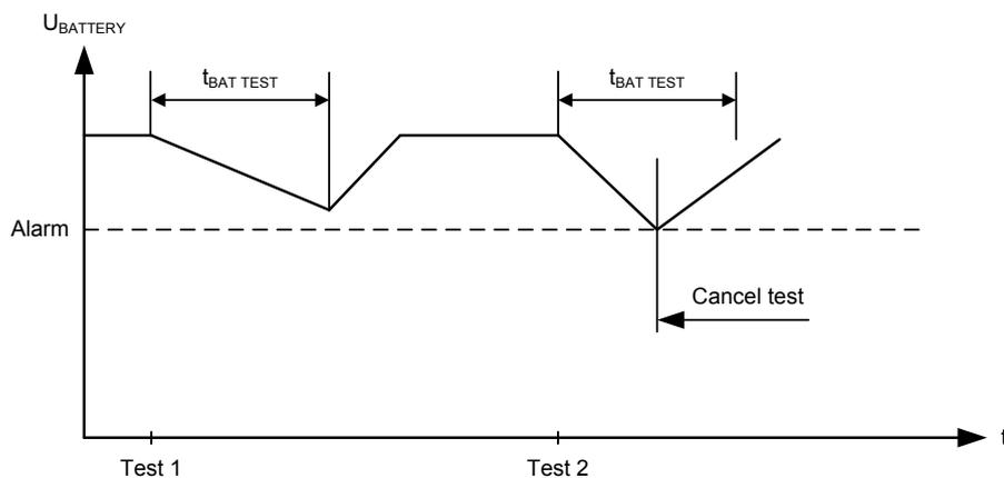
The drawing shows that test #1 is carried out without a large voltage drop of the battery voltage, whereas test #2 reaches the alarm set point. As there is no reason to wear the battery down even more, the test stops when the battery test alarm occurs.
