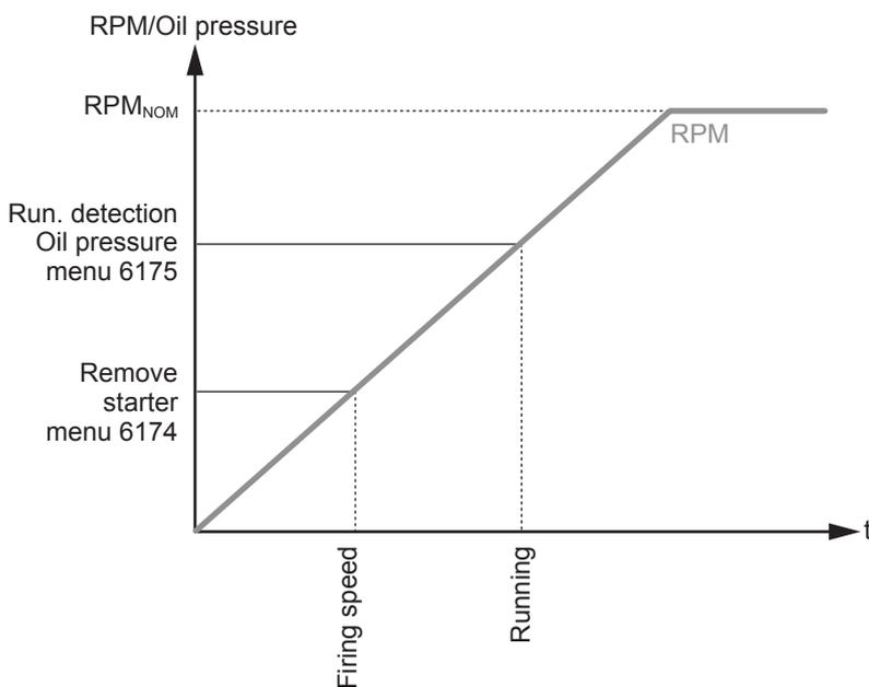
**NOTE** The remove starter function can use the MPU or a digital input.
