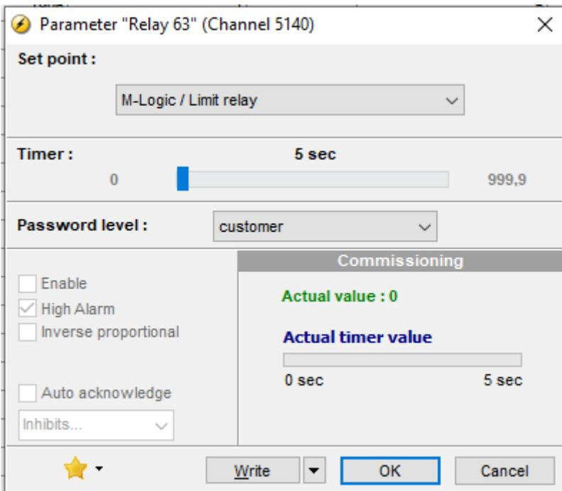
**NOTE** If the relay function is not changed to *M-Logic / Limit* function, an alarm will appear at every running situation.
