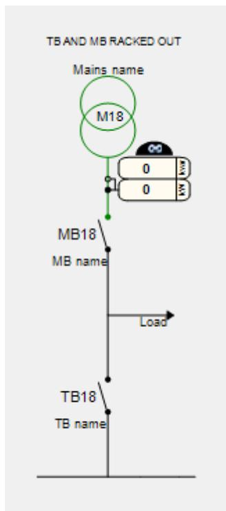
**NOTE** It is important to physically check that the breaker is actually racked out/disconnected from the busbar or is physically in the test position. When the racked out signal is active, no synchronisation is present, and if the
