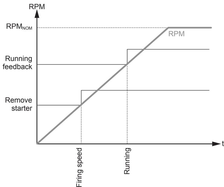
The diagram illustrates how the remove starter input is activated when the engine has reached its firing speed. At the running speed, the digital running feedback is activated.
