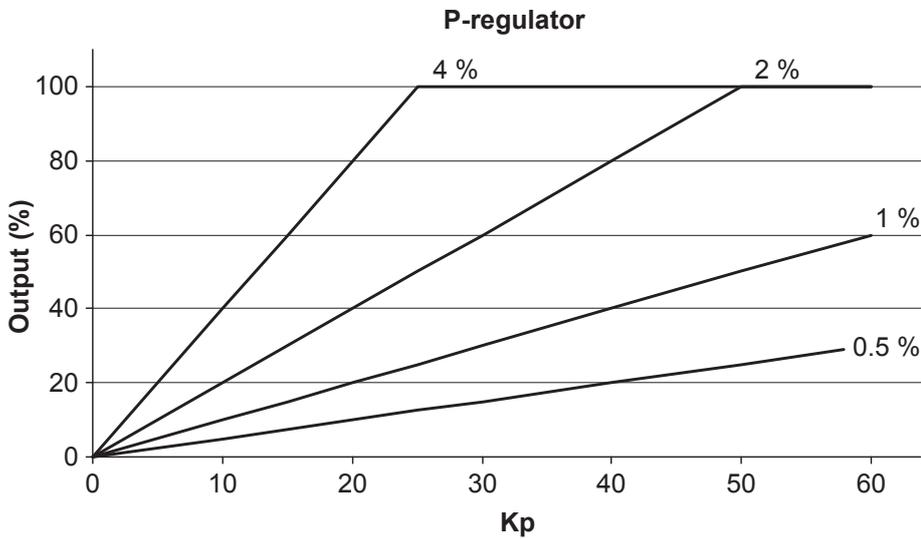
In this example we have a 2 percent regulation deviation and an adjusted value of the  $K_p = 20$ . The calculated regulator value of the controller is 40%. Now the pulse length can be calculated with a period time = 2500 ms:
