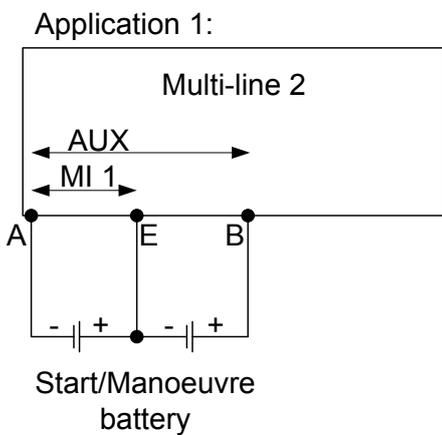
The power supply measurement is used as the reference RF1 (points A and B) in menu 6432 and multi-input 1 is used as the type T1 (points A and E) in menu 6431. By making these measurements, it is possible to calculate the voltage between E and B. This gives a full picture of battery voltages, for example:
