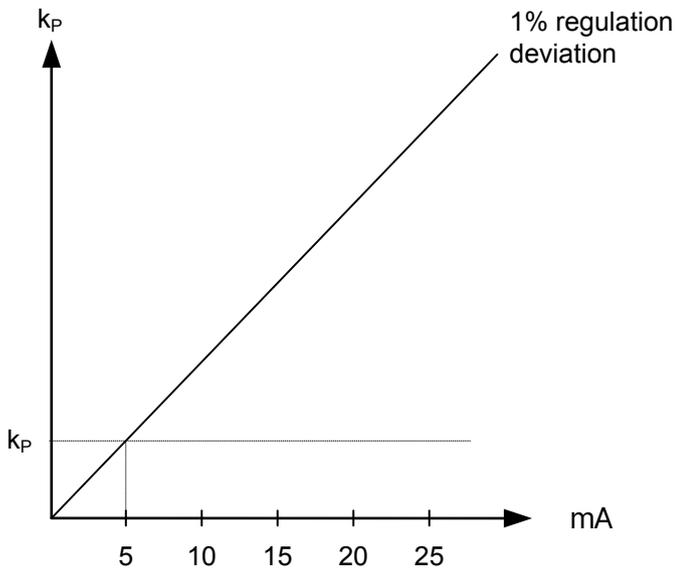
A 1% regulation deviation occurs. With the Kp setting adjusted, the deviation causes the output to change 5 mA. The table shows that the output of the AGC changes relatively much if the maximum speed range is low.
