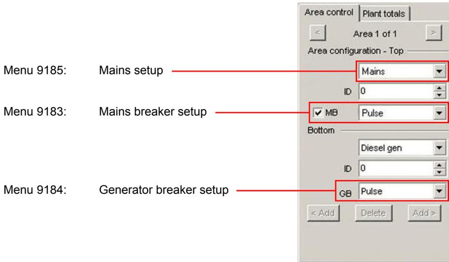
**NOTE** If *Setup stand-alone* is activated while the genset is running, an info text, *Quick setup error*, will appear.
