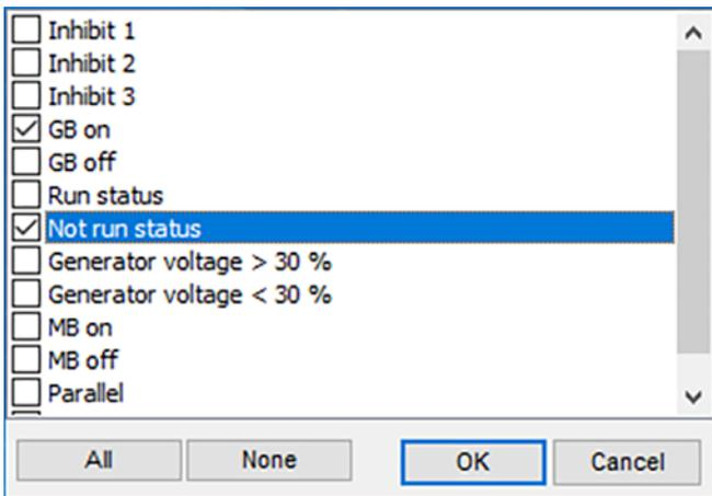
In this example, inhibit is set to *Not run status* and *GB ON*. Here, the alarm will be active when the generator has started. When the generator has been synchronised to the busbar, the alarm will be disabled again.
