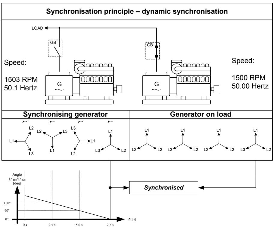
In the example above, the synchronising genset is running at 1503 RPM ~ 50.1 Hz. The generator on load is running at 1500 RPM ~ 50.0 Hz. This gives the synchronising genset a positive slip frequency of 0.1 Hz.
