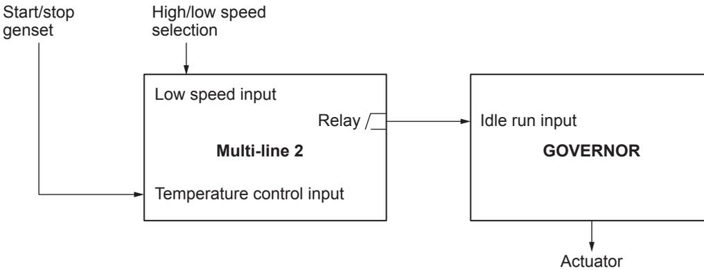
**NOTE** To invert the relay output, you need to use a changeover relay. Connect the wiring to the common and normally closed terminals.
