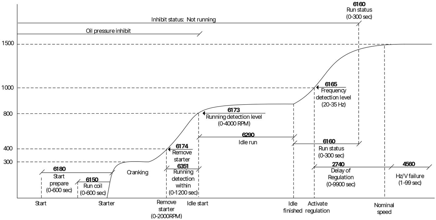
The set points and failures in this overview are the same as described in the chapter "Start-up overview", except for the idle run function. This function is described in the chapter "Idle running".
