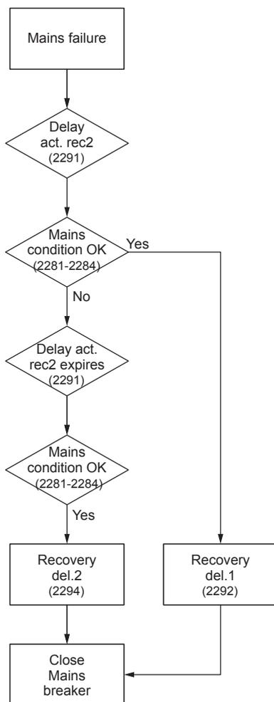
If the *Delay activate recovery 2* timer runs out, the long interruption timer (menu 2294 *Recovery del. 2*) will start to run.
