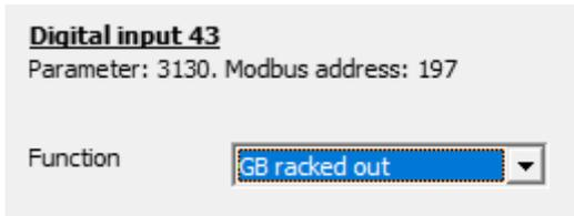
**NOTE** Depending on the controller type, GB, TB, MB or BTB -*racked out* is shown in the input list.
