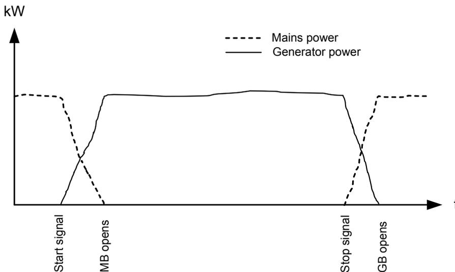
**NOTE** The load takeover mode can be combined with the overlap function. In that case, the generator and the mains breakers will never be closed at the same time for a longer period than the adjusted *overlap* time.
