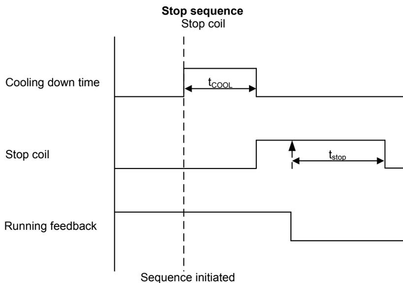
The stop sequence is activated if a stop command is given. The stop sequence includes the cooling down time if the stop is a normal or controlled stop.
