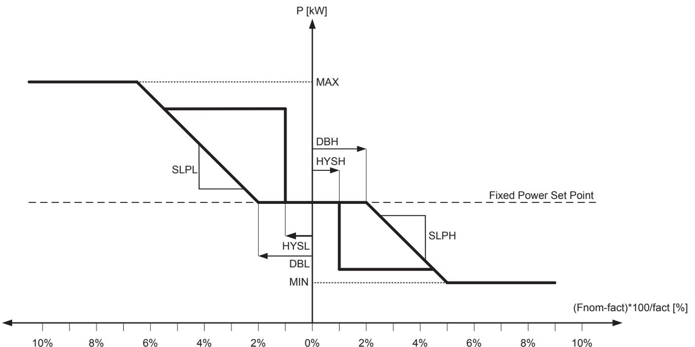
The droop curve can be specified within the area from P min to P max.
