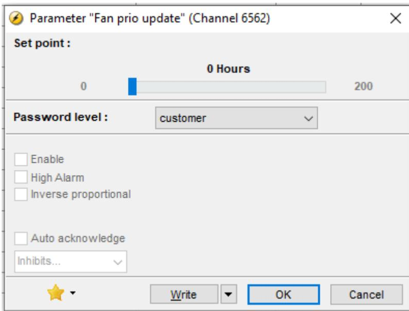
If the fan priority update is set to 0 hours, the priority order is: Fan A, Fan B, Fan C, Fan D.
