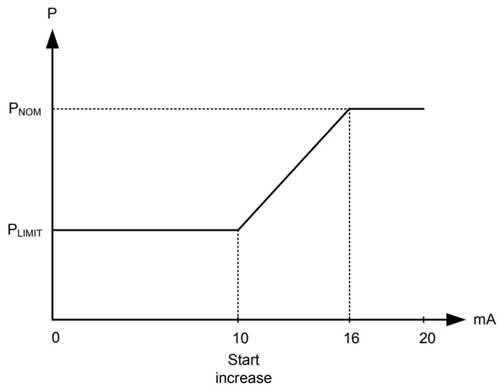
Use *Enable* in parameter 6246/6256/6266 to select the derate characteristic:
