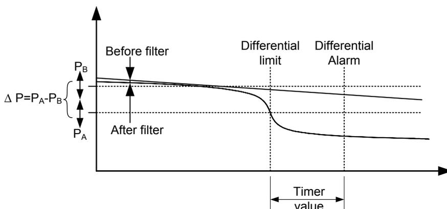
Nine different differential measurements between two analogue input values can be configured. Differential measurements between two sensors can be configured in menus 4600-4606, 4670-4676 and 4741-4746.
