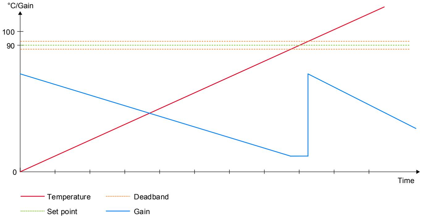
The diagram above shows how the reaction to a set point deviation could look.
