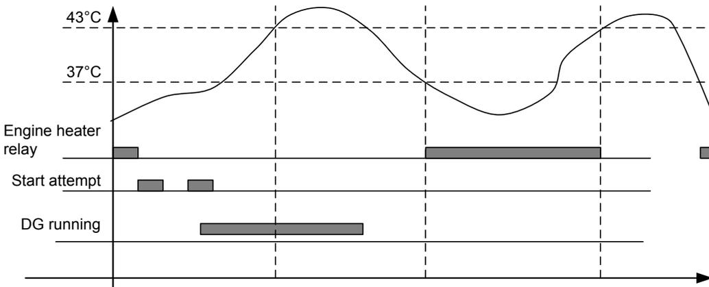
**NOTE** The engine heater function is only active when the engine is stopped.
