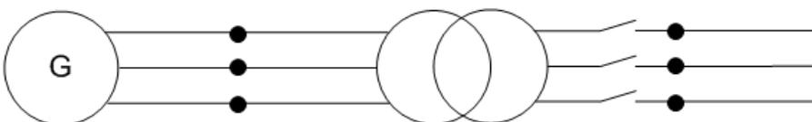
Typically the synchronising breaker is on the high voltage (HV) side, and there is no breaker (or only a manually operated one) on the low voltage (LV) side. In some applications, the breaker could also be placed on the LV side. But this does not influence on the setting in the ML-2, as long as the breaker and the step-up transformer are both placed between the
