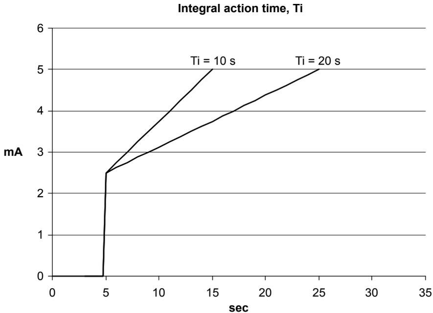
As shown in the drawing, the output reaches 5 mA twice as fast at a  $T_i$  setting of 10 s than with a setting of 20 s.
