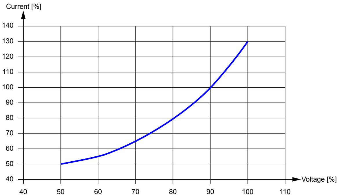
When the actual values represent a point above the curve, the breaker should be tripped. The curve shows that the generator breaker will trip when two requirements are met: The generator voltage is below 50 % of rated, and the current is above 50 % of rated.
