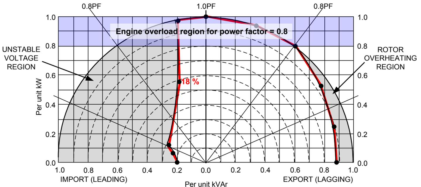
The alternator 100 % load is the outer circle, and the engine 100 % load is the bottom of the blue block. With the operating chart it is possible to see where the alternator-safe line is closest to the 1.0 PF line. In this operating chart each vertical line represents 10 %, and so the point closest to 1.0 PF is 18 %. Use the nominal alternator values and the nominal engine values to do the calculations.
