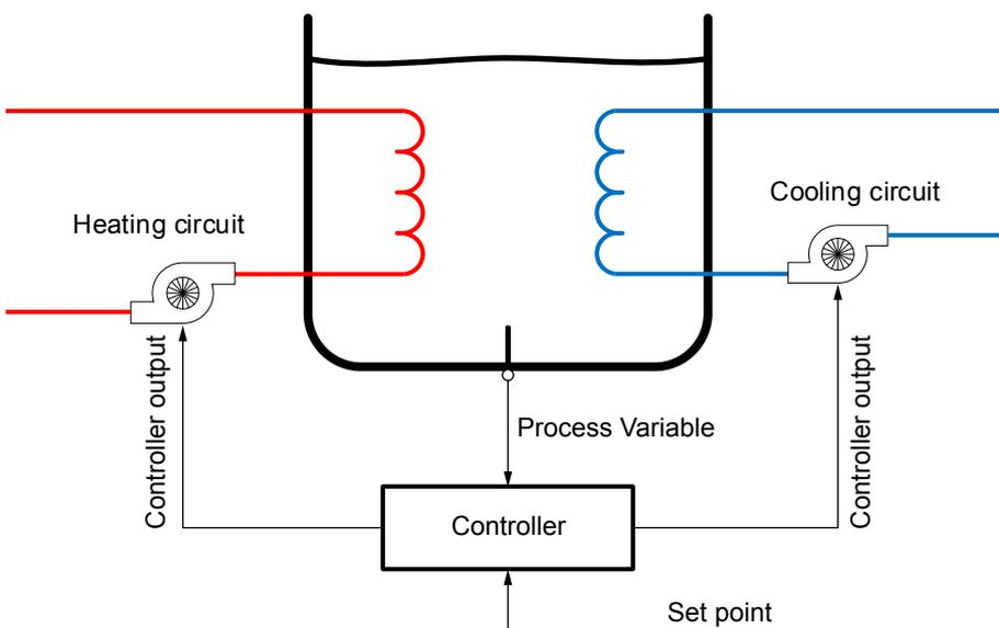
For this application, two controllers must be configured. one with a direct output for the heating pump and one with an inverse output for the cooling pump. To achieve the inverse output shown, an offset of 100 % is needed. See **Analogue offset** and **Example of inverse output with 100 % offset** for more information.
