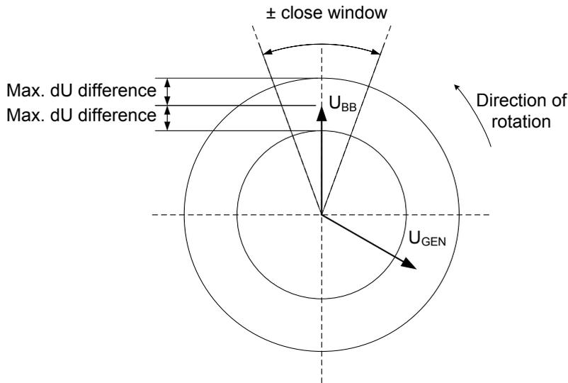
The synchronisation pulse is sent dependent on the settings in menu 2030. It depends on whether it is the GB or the MB that is to be synchronised.
