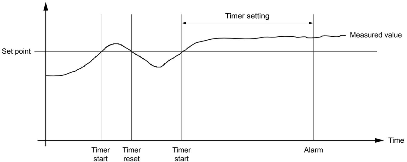
When the timer runs out, the output is activated. The total delay will be the delay setting + the reaction time.
