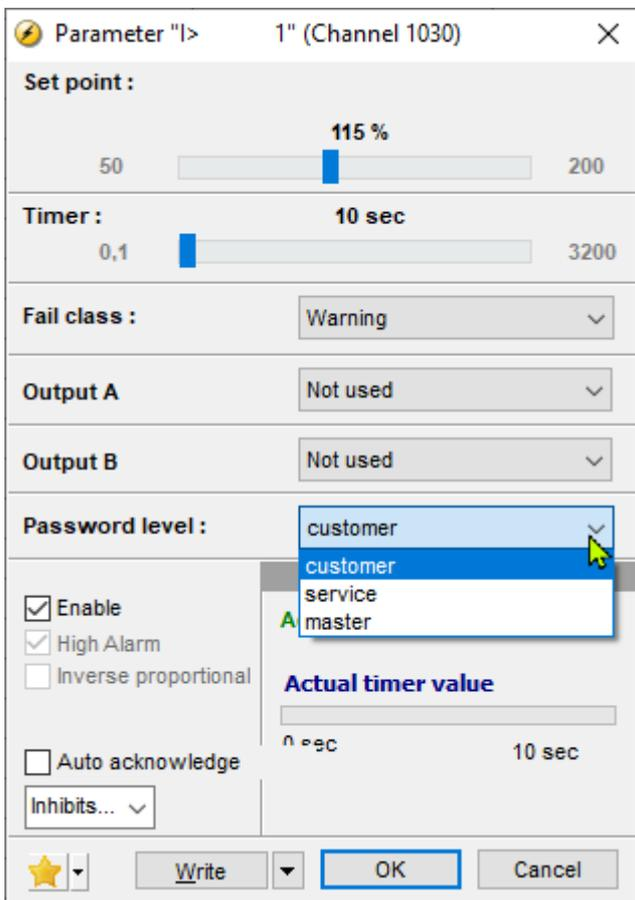
The password level can also be changed from the parameter view in the column "Level". Right-click the field, select "Change access level" and then select the required password level.
