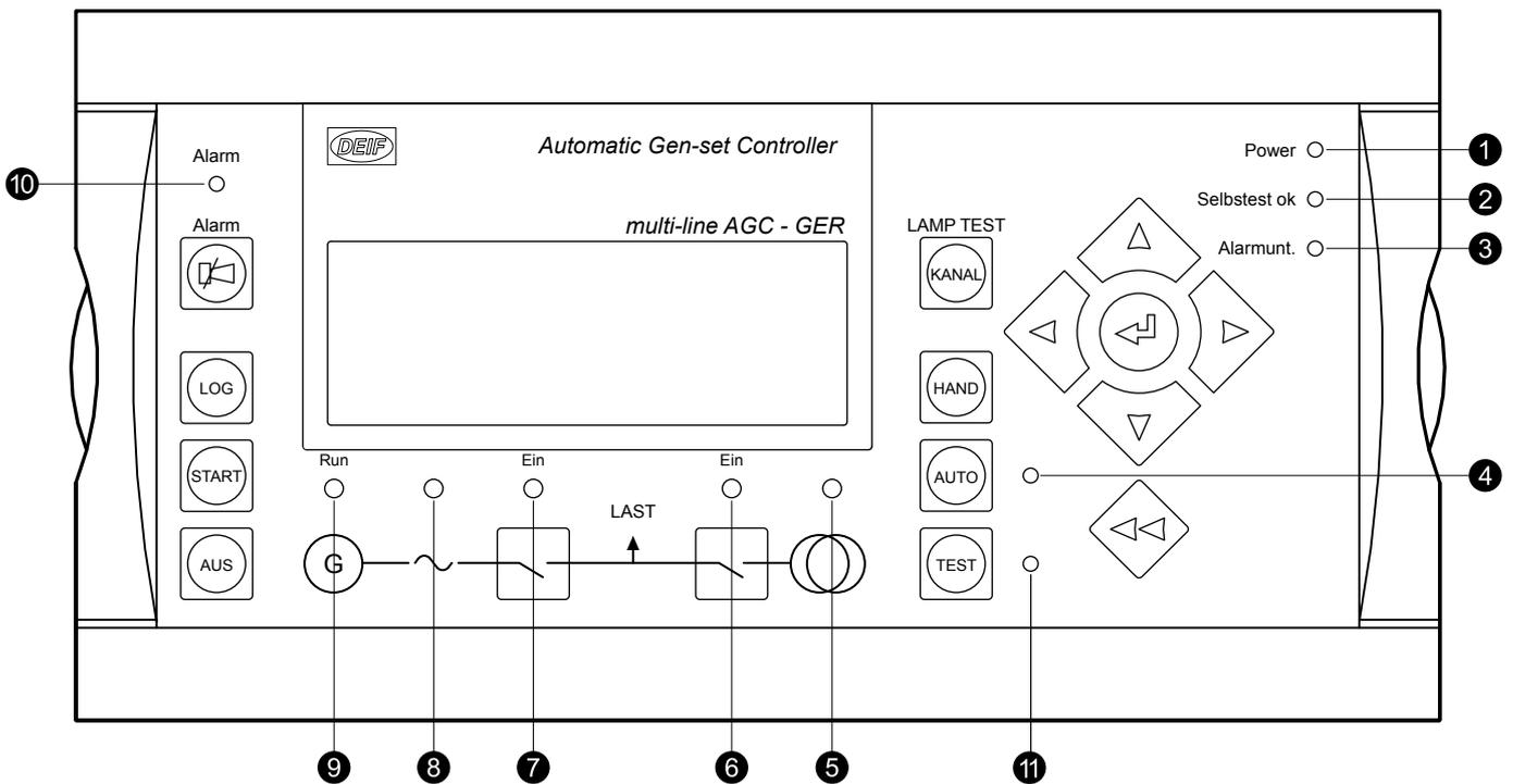
1. LED indicates that the auxiliary supply is switched on.
