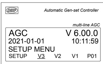
This window is the gateway to the other menus. View V3 can always be reached by pushing the BACK button three times.
