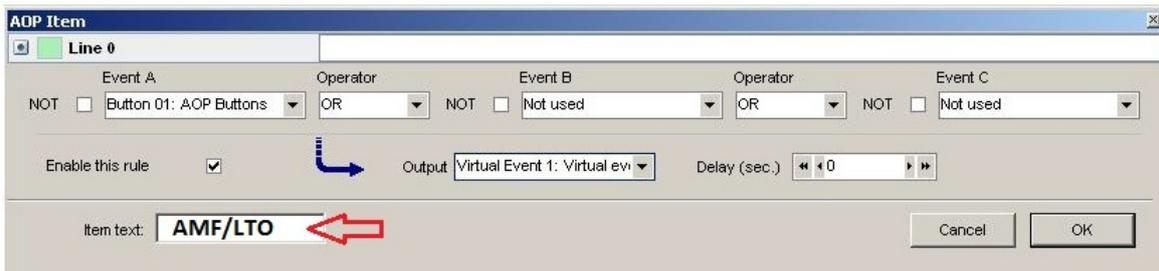
The item text can be written individually and printed, so it can be put in the AOP-2 front pockets. In this case, it is "AMF/LTO".
