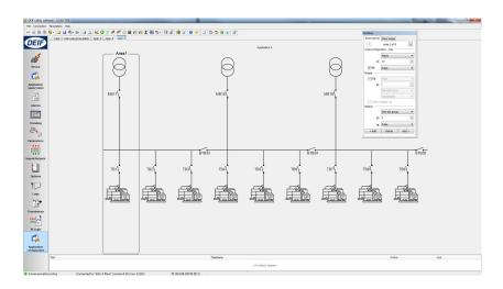
The application drawing is programmed to the controller, and the plant layout is then programmed.
