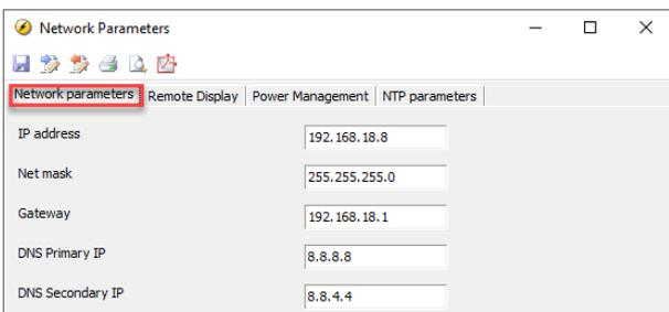
4. Select the *Write to device button*
