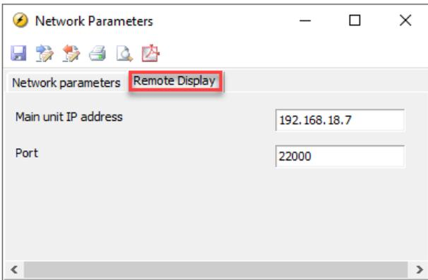
5. Click the *Write to device button*
