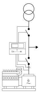
**Automatic Mains Failure (AMF):** If there is a significant loss of mains power or a total blackout, the controller automatically changes the supply to the emergency generator. This makes sure that there is power during a mains failure and prevents damage to electrical equipment.
