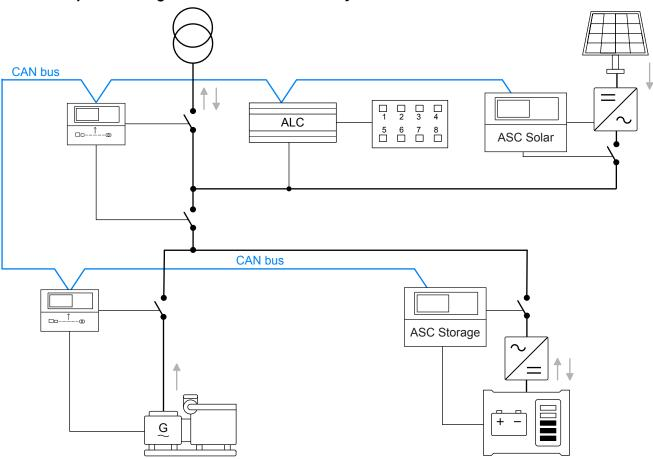
**NOTE** You can use AGC 150 generator, mains, and bus tie breaker controllers for power management in a hybrid system. However, the AGC 150 hybrid controller cannot be used in a power management application. To control the photovoltaic (PV) power source(s), use ASC Solar.
