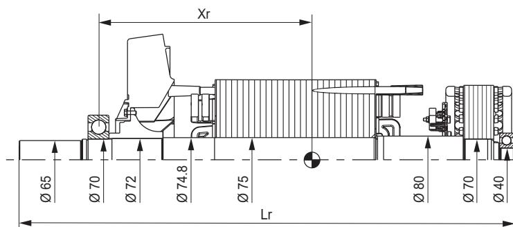
Centre of gravity: Xr (mm), Rotor length: Lr (mm), Weight: M (kg), Moment of inertia: J (kgm<sup>2</sup>): (4J = MD<sup>2</sup>)
