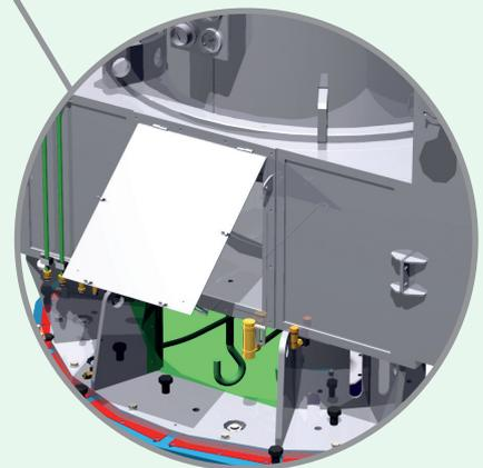
Fast opening louvers for powerhouse heating and/or in case of water supply failure
