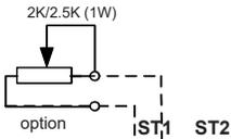
Option: R1-R2 - External remote voltage trimmer (remove ST1)
